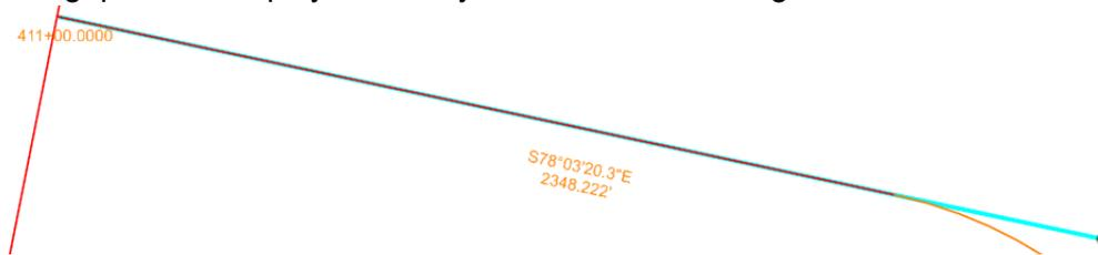
An interval element is ruled to the original geometry (or "*gap*" element), and this dependency can be viewed in the *OpenRoads Model* tab in the *Explorer*.
