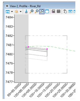
Upon completion the components of the MtnHwy corridor will now be displayed onto the profile. If the corridor changes, you will need to refresh the 3D cut by using the *Refresh 3D Cut* tool located to the right of the 3D Cut icon.
