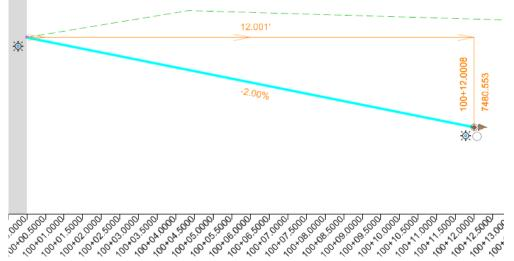
Sometimes it is necessary to display components of a corridor onto the profile. You can do this by using the *Create 3D Cut* tool. This tool will allow you to cut through a corridor and display the corridor's components onto the profile.
