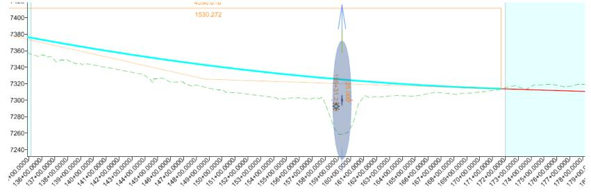
To finish up the vertical geometry, we need to create one last vertical curve at station 110+00 [1+300].
