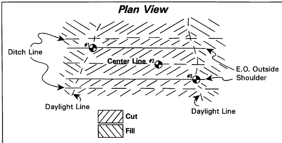
**FIGURE SS-1.** Recommended location of test holes in the cut section.
