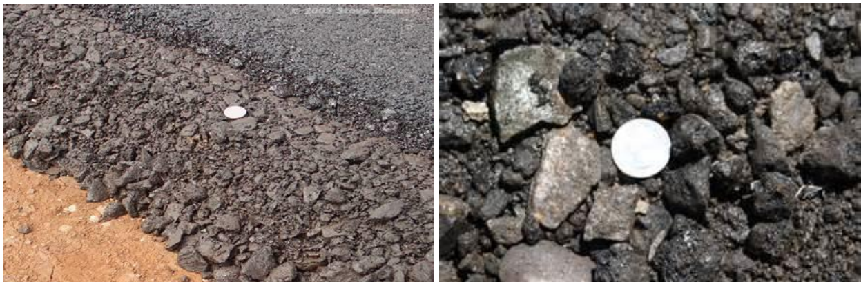
Figure 5.8 Photos of Reclaimed Asphalt Pavement Base
