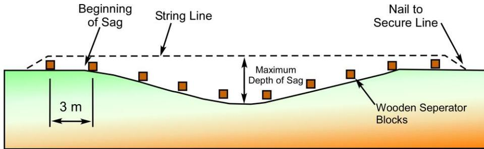
**Figure 10.20 Typical Slab Raising in Slabjacking**
