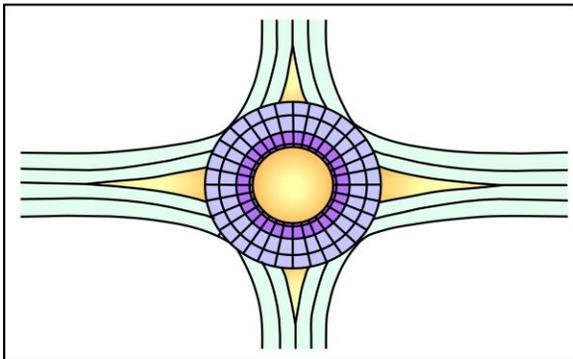
Step 3. In the circle, add "transverse" joints radiating out from the center of the circle. Make sure that the largest dimension of the pie-shaped slab is smaller than the maximum recommended. Extend these joints through the back of the curb and gutter.
