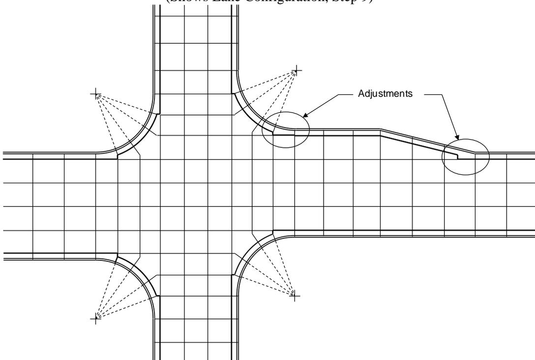
**Figure 12.7 Typical Joint Layout for a Rigid Pavement Intersection**
