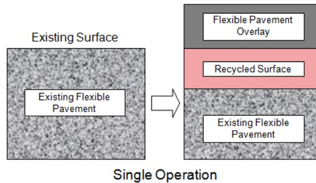
Repaving is the process of heating, scarifying, adding rejuvenating agent and mixing of the surface. A new hot mix asphalt overlay is placed over the heated recycled surface. These two operations are done simultaneously in a paving train operation. A strong thermal bond is formed between the two layers. The overlay is compacted with a roller. Depth of scarification is usually between  $\frac{3}{4}$ " and  $1\frac{1}{2}$ ".
