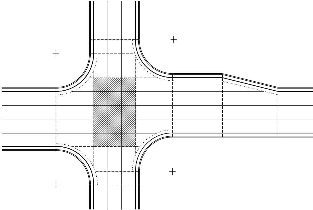
**Figure 12.4 Typical Joint Layout for a Rigid Pavement Intersection**
