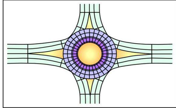
Step 4. On the legs, add transverse joints at all locations where a width change occurs in the pavement (at bullnose of median islands, begin and end of curves, tapers, tangents, curb returns, etc.). Extend these joints through the back of the curb and gutter.
