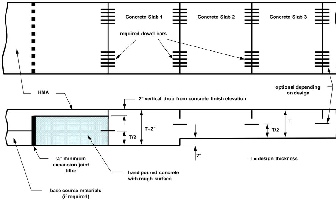
**Figure 12.8 Detail of Asphalt and Concrete Slab Joint**
