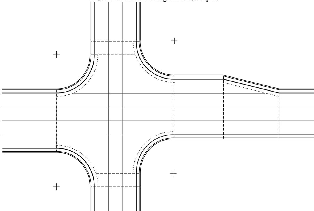
**Figure 12.3 Typical Joint Layout for a Rigid Pavement Intersection**
