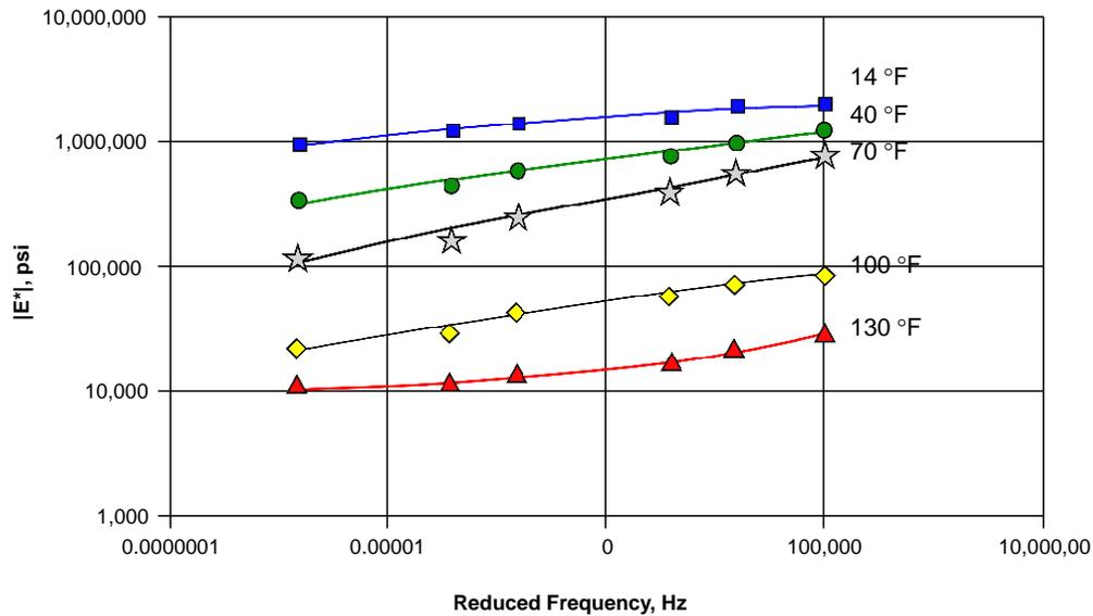
The  $|E^*|$  master curve can be represented by a sigmoidal function as shown (27):
