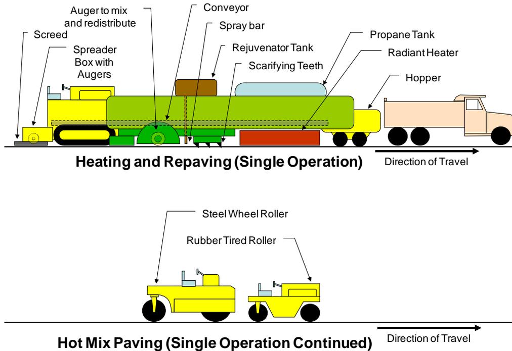
**Figure 8.20 Hot Mix Paving (Single Operation Continued)**
