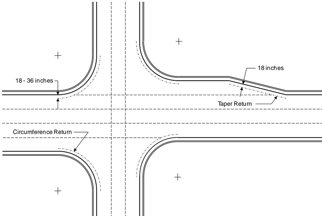
**Figure 12.2 Typical Joint Layout for a Rigid Pavement Intersection**
