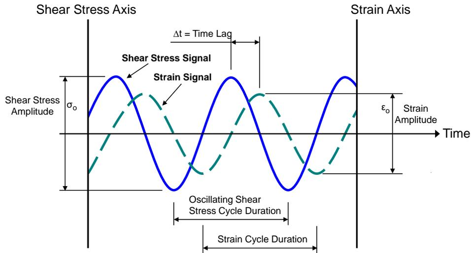
**Figure S.9 Dynamic Modulus Stress-Strain Cycles**
