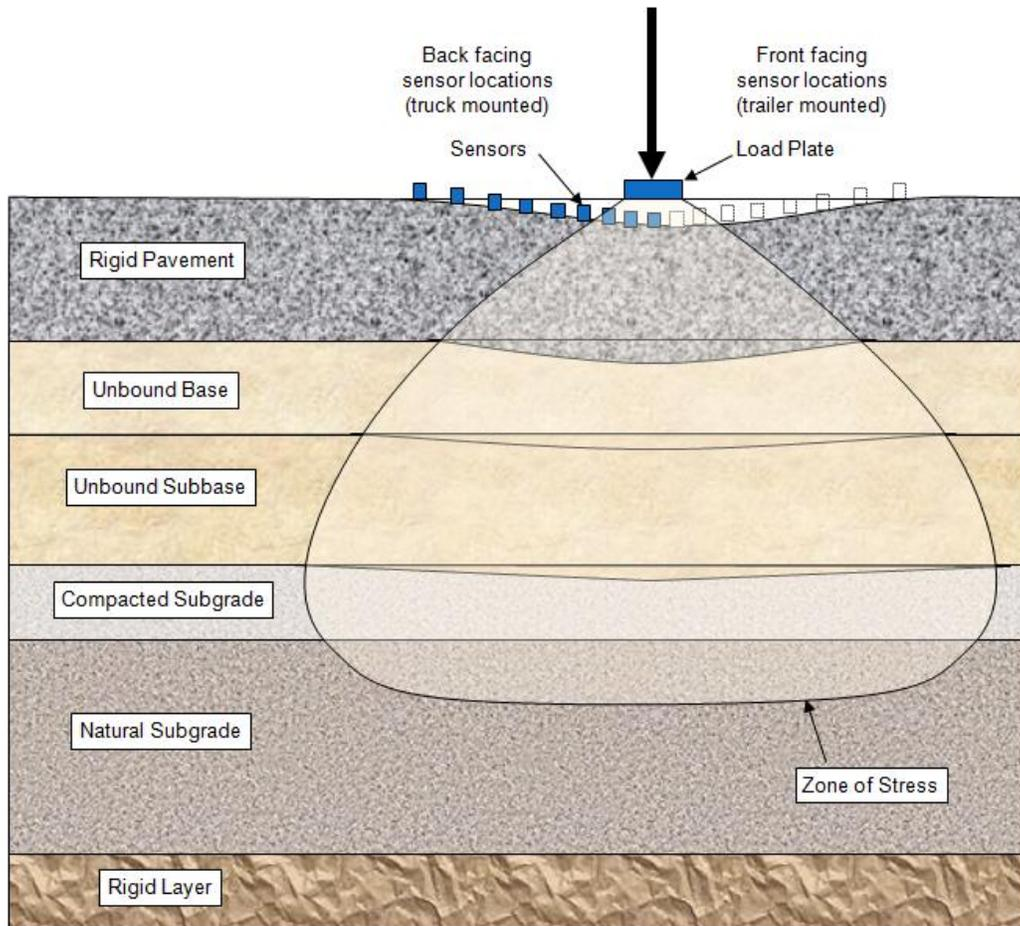
**Figure C.1 Depiction of FWD Load Distribution Through Pavement**
