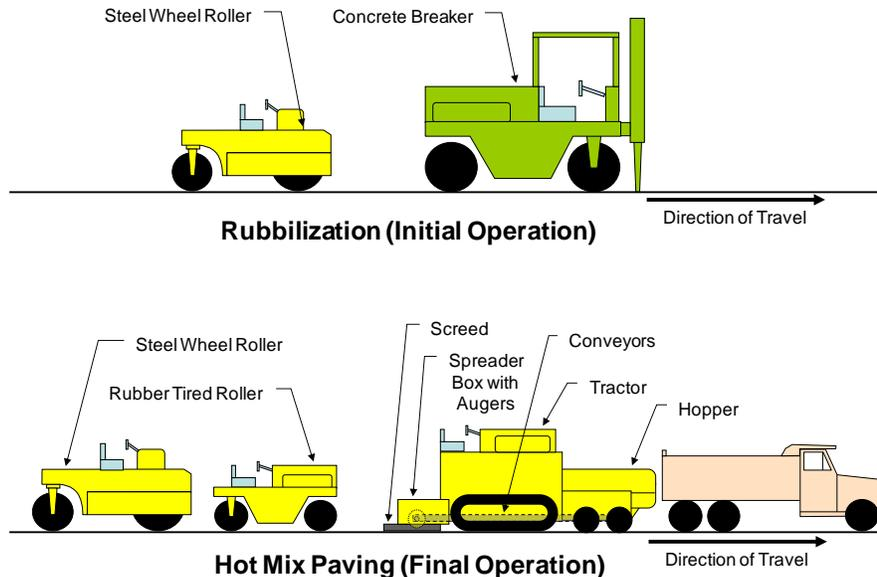
**Figure 8.34 Schematic of Rubblization and Overlay Equipment**
