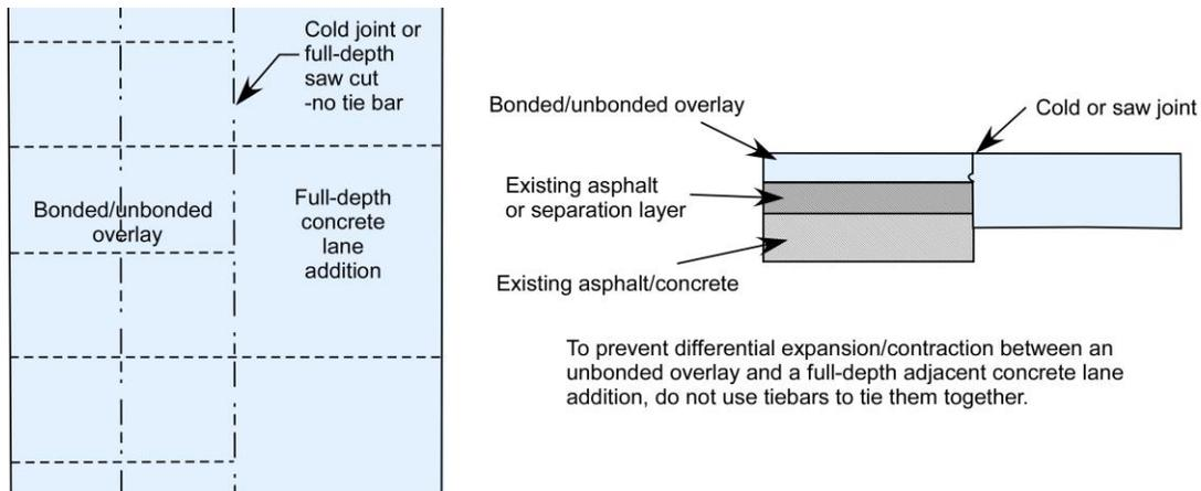
Note: The figure illustrates lane addition details. To prevent cracking related to differential expansion and contraction between a concrete overlay and a full-depth adjacent concrete lane addition, use a butt joint with no tiebars.
