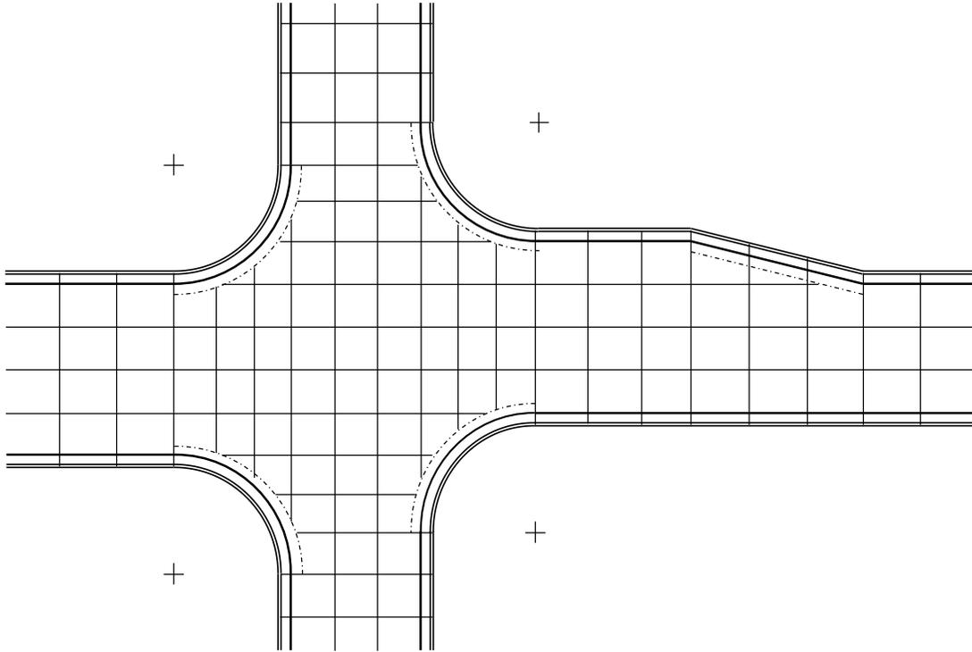
**Figure 12.6 Typical Joint Layout for a Rigid Pavement Intersection**
