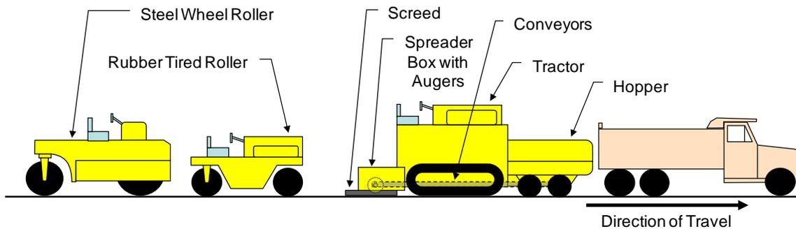
**Figure 8.26 Schematic of Conventional HMA Paving Equipment**
