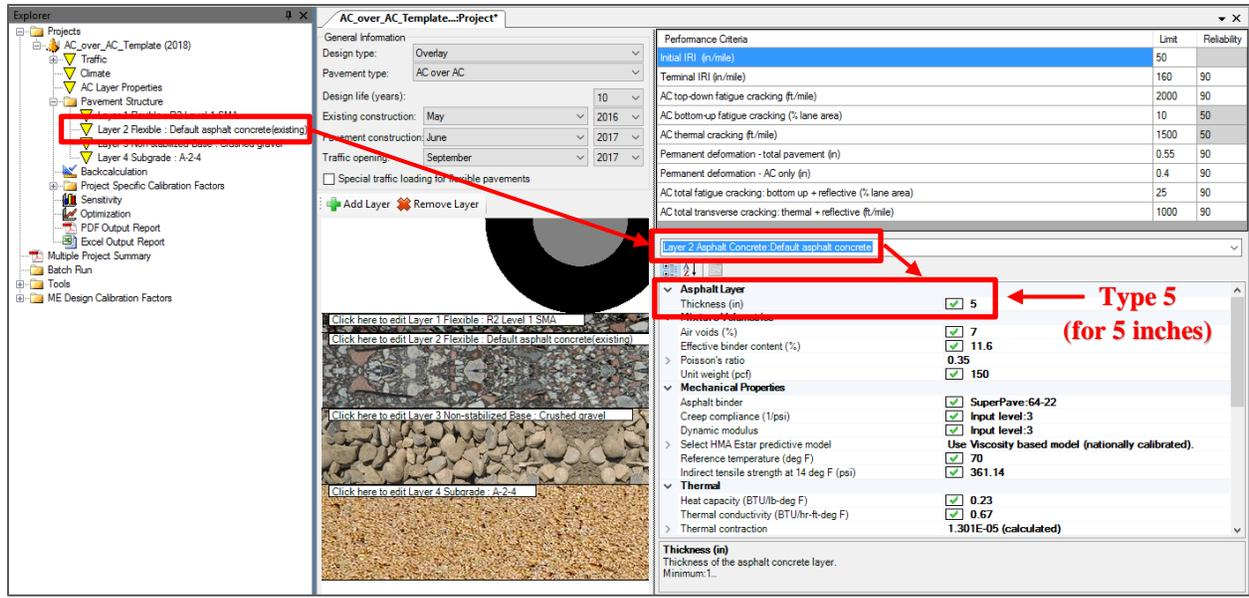
Figure 8.53 Existing Layer Thickness if Milling is Planned
