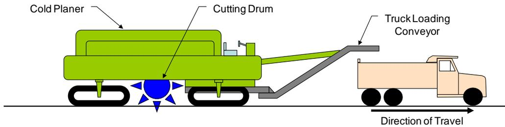
**Figure 8.10 Schematic of Cold Planing Equipment**
