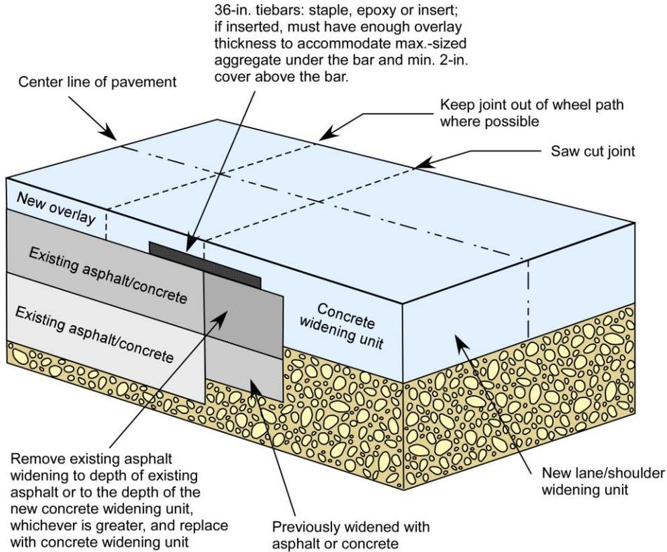
Note: Three to six foot widening units are illustrated in this figure. The intent of the tiebars is to tie the widening unit to the existing pavement.
