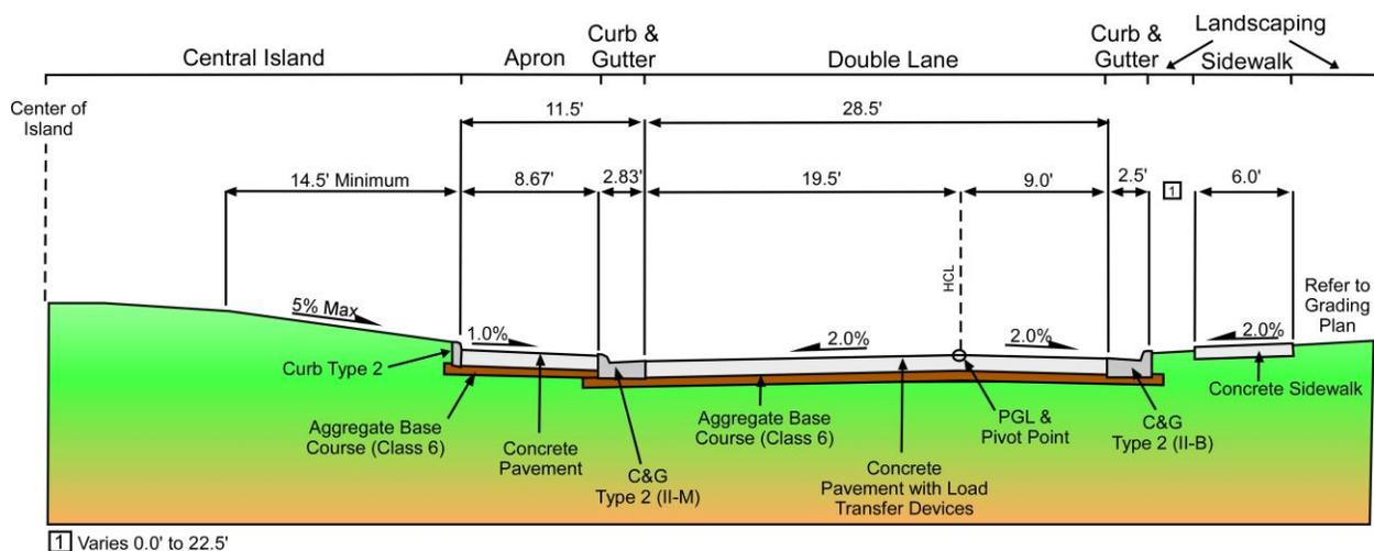
**Figure 12.14 Typical Section of an Urban Double-Lane Roundabout**
