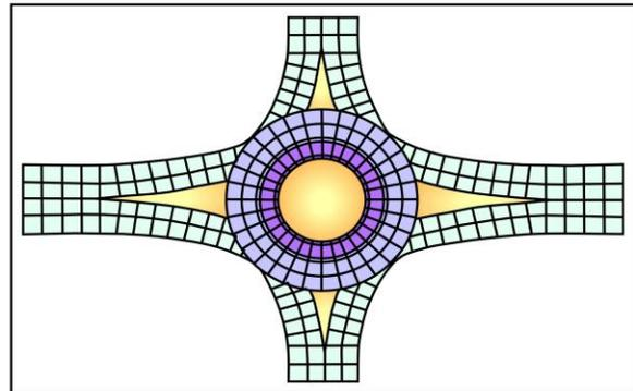
Step 5. Add transverse joints beyond and between those added in Step 4. Space joints out evenly between other joints, making sure not to violate maximum joint spacing.
