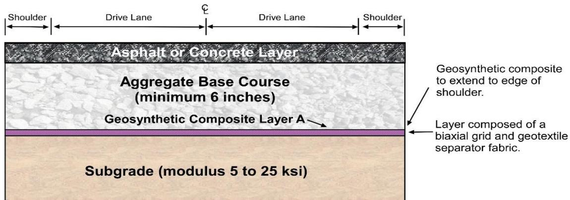
**Figure I.1 Typical Section**
