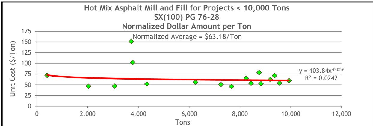
**Figure 13.67 HMA Mill and Fill Normalized Unit Costs for SX(100) PG 76-28 on Projects Less Than 10,000 Tons**
