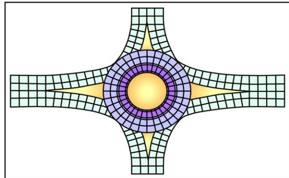
Step 6. Make adjustments for in-pavement objects, fixtures and to eliminate L-shapes, small triangular slabs, etc.
