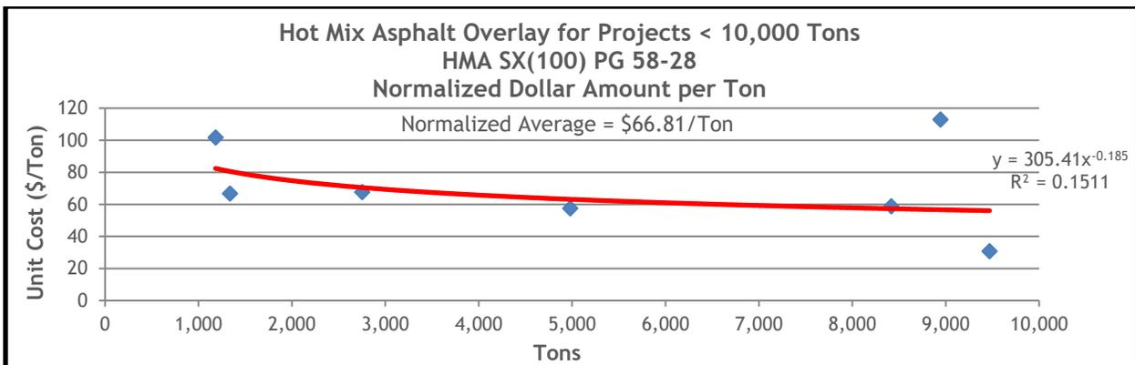
**Figure 13.53 HMA Overlay Normalized Unit Costs for SX(100) PG 58-28 on Projects Less Than 10,000 Tons**
