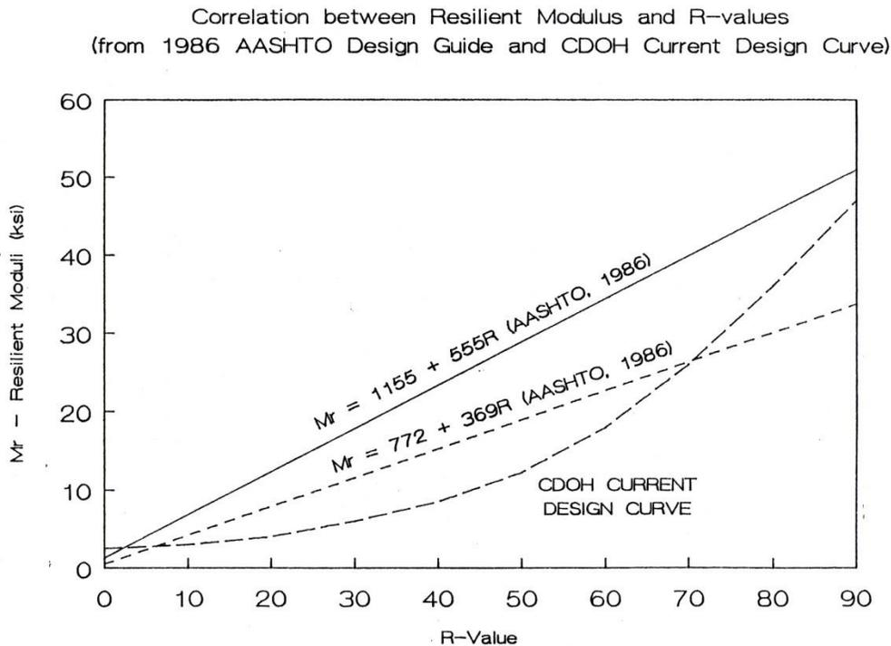
**Figure S.26 Correlation Plot between Resilient Modulus and R-value**
