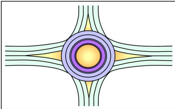
Step 2. Draw all lane lines on the legs and in the circular portion. If isolating circle from legs, do not extend these through the circle. If using "pave-through" method, determine which roadway will be paved through. Make sure no distance is greater than the maximum recommended width.
