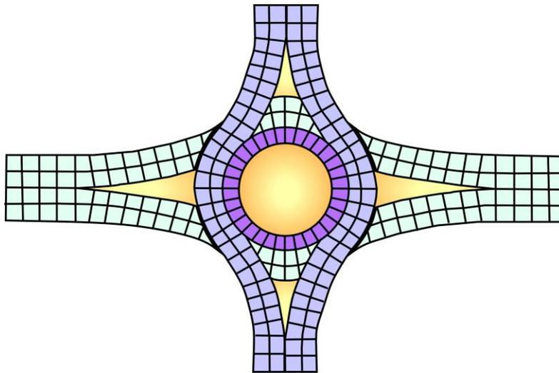
**Figure 12.11 Pave-Through Layout**
