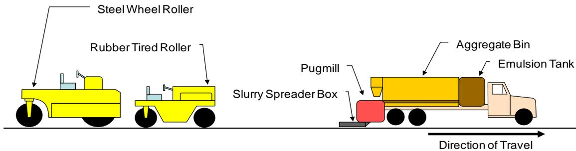
**Figure 8.23 Schematic of Thin Wearing Course Equipment**
