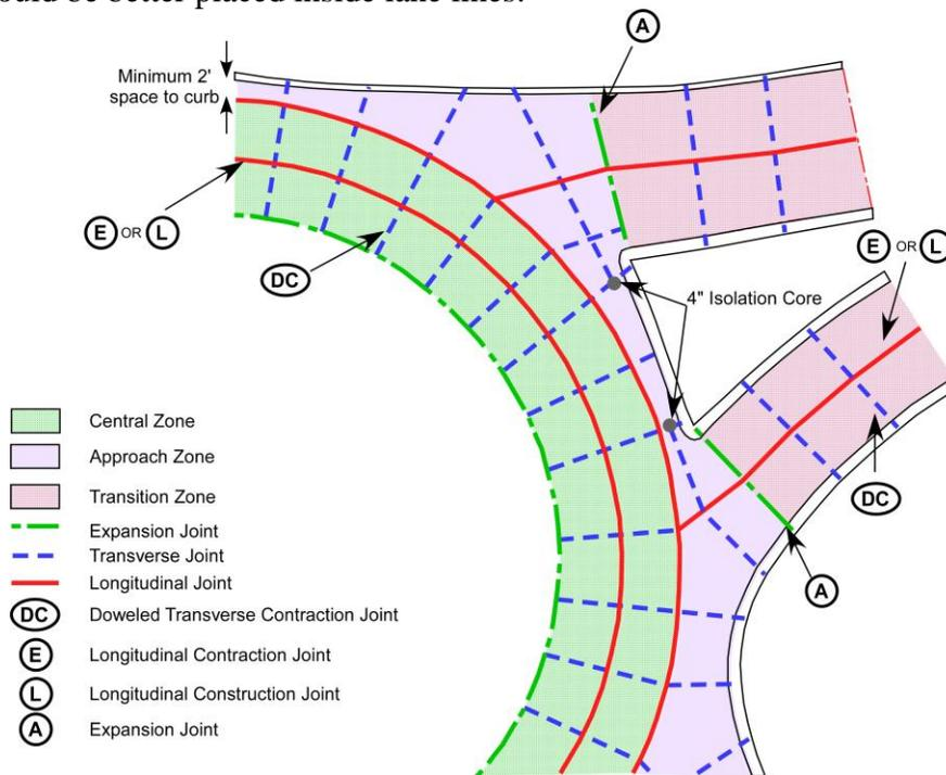
**Figure 12.13 Basic Joints and Zones of a Roundabout**
