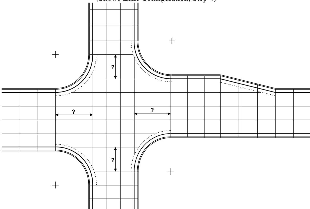
**Figure 12.5 Typical Joint Layout for a Rigid Pavement Intersection**
