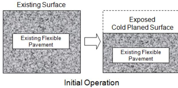
Cold planing is the removal of the top portion of existing flexible pavement. The material is removed and stockpiled.
