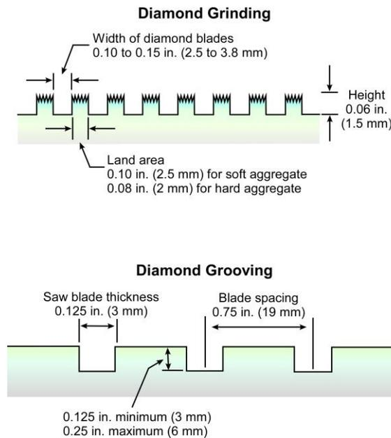
**Figure 10.3 Dimensions for Grinding and Grooving**
