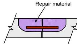
**Figure 10.15 Typical Dowel Bar Retrofit Sequencing of the Installation**
