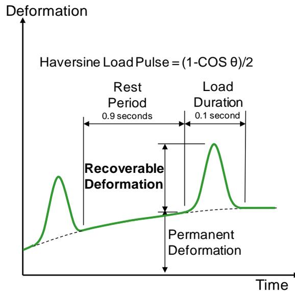
**Figure S.23 Resilient Modulus Test Specimen Loading**
