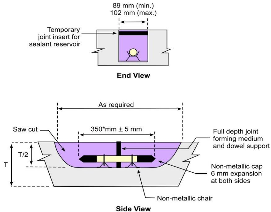
**Note:** For pavements with poor support conditions slightly longer bars should be considered.
