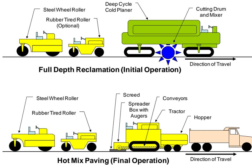
**Figure 8.31 Schematic of FDR Equipment**
