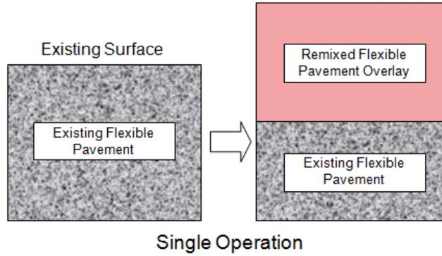
Remixing is a process that heats, plans (mills) and removes 1 ½" to 2" of the existing pavement, then adds in rejuvenating agent, virgin aggregate or new hot mix asphalt (HMA). All materials are mixed in a small mobile pug mill to form a single, homogenous mixture. The operation is simultaneously performed in a paving train operation. The overlay mixture is compacted with a roller.
