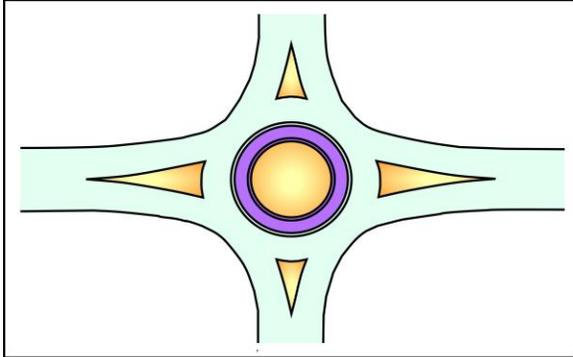
Step 1. Draw all pavement edge and back-of curb lines in the plan view. Draw location of all manholes, drainage inlets, and valve covers so that joints can intersect these.
