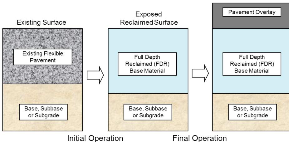
FDR is the pulverizing, without heat, of existing flexible pavement to produce an aggregate base material by mixing of some or all of the underlying granular base, subbase or subgrade material.
