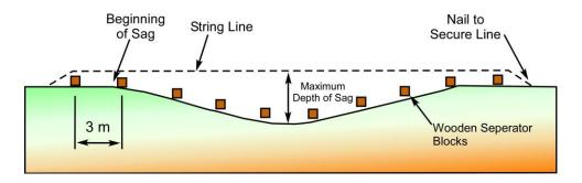
Figure 10.20 Typical Slab Raising in Slabjacking
