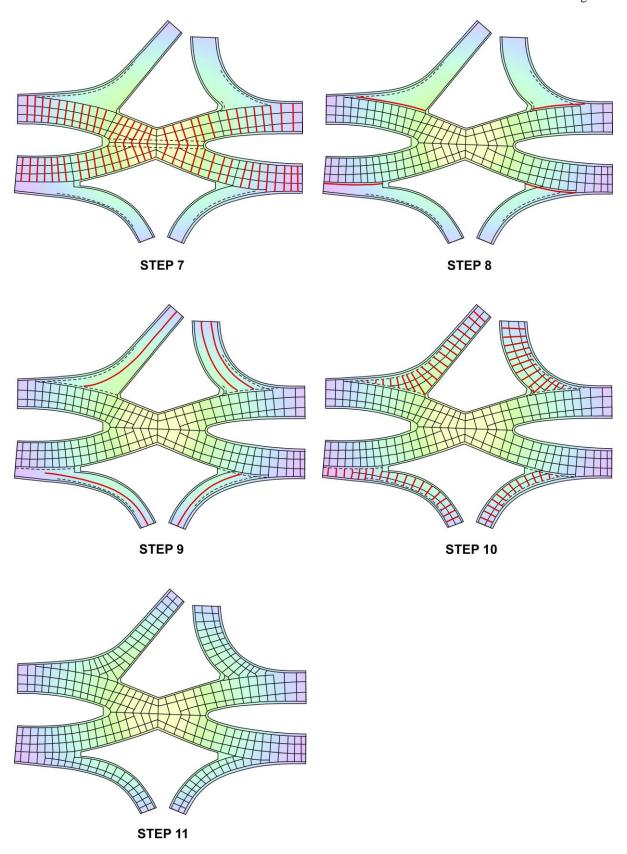
Figure 12.15 Divergent Diamond Interchange 11-Step Quadrant Method
