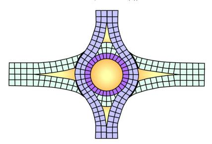
Figure 12.11 Pave-Through Layout
