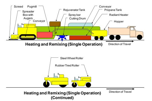
Figure 8.17 Schematic of Remixing Equipment
