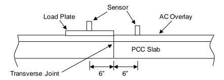
Figure C.7 Joint Load Transfer Testing Sensor Spacing
