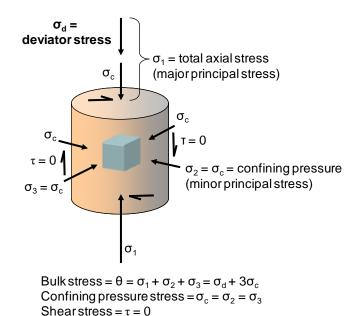
Figure S.22 Resilient Modulus Test Specimen Stress State
