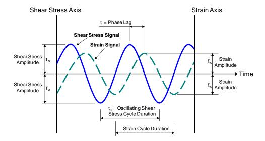
Figure S.14 Binder Complex Shear Modulus Shear-Strain Cycles
