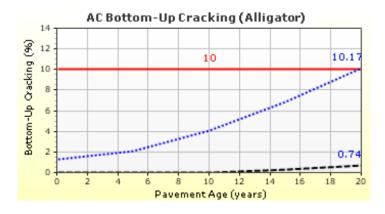
Figure 13.2 AC Bottom-Up Cracking at 95 Percent Reliability
