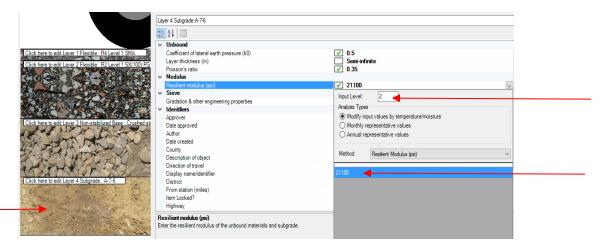
Figure I.7 Adjusting the Resilient Modulus of the Subgrade in PMED
