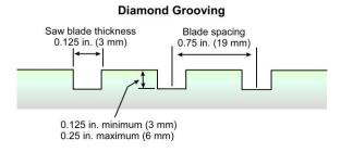
**Figure 10.3 Dimensions for Grinding and Grooving** From Figure 7, *Concrete Pavement Rehabilitation and*
