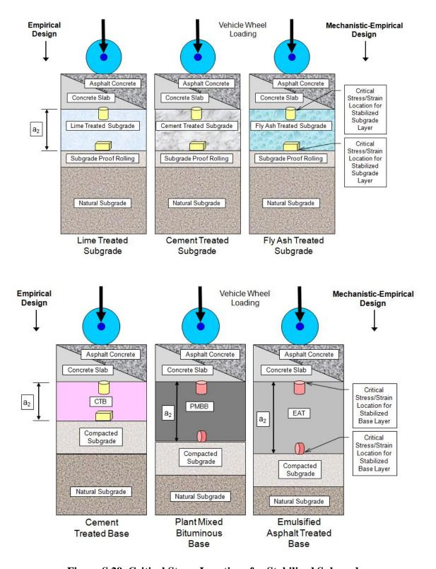
Figure S.29 Critical Stress Locations for Stabilized Subgrade
