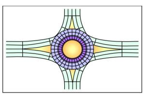
Step 4. On the legs, add transverse joints at all locations where a width change occurs in the pavement (at bullnose of median islands, begin and end of curves, tapers, tangents, curb returns, etc.). Extend these joints through the back of the curb and gutter.
