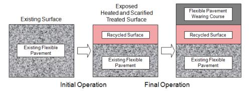
Surface Recycling heats, scarifies, and sprays rejuvenating agent. The material is then mixed with an auger, leveled off with a screed and rolled with a rubber-tired roller. Depth of scarification is usually between 3/4" and 1 1/2".
