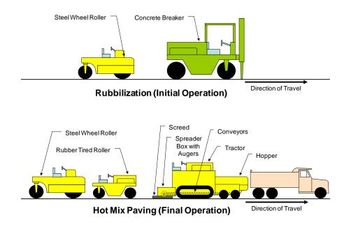
Figure 8.34 Schematic of Rubbilization and Overlay Equipment
