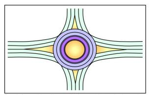
Step 2. Draw all lane lines on the legs and in the circular portion. If isolating circle from legs, do not extend these through the circle. If using "pave-through" method, determine which roadway will be paved through. Make sure no distance is greater that the maximum recommended width.
