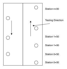
Figure C.2 Flexible Pavement Staggered Testing Pattern
