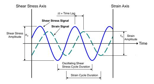
Figure S.9 Dynamic Modulus Stress-Strain Cycles
