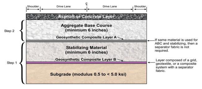
**Note 1:** As a minimum, a separator fabric shall be required between the subgrade and the stabilizing material.
