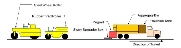
Figure 8.23 Schematic of Thin Wearing Course Equipment
