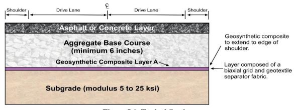
**Figure I.1 Typical Section**
