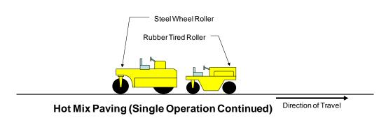
Figure 8.20 Hot Mix Paving (Single Operation Continued)
