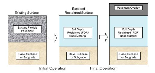
FDR is the pulverizing, without heat, of existing flexible pavement to produce an aggregate base material by mixing of some or all of the underlying granular base, subbase or subgrade material.
