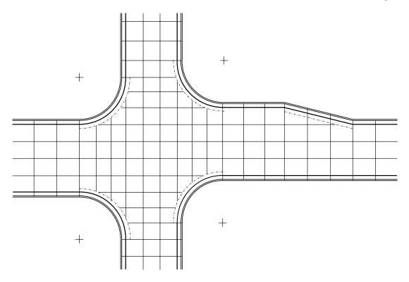
Figure 12.6 Typical Joint Layout for a Rigid Pavement Intersection (Shows Lane Configuration, Step 9)
