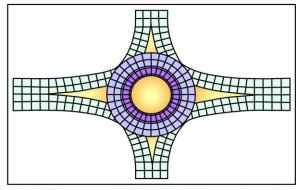
Step 5. Add transverse joints beyond and between those added in Step 4. Space joints out evenly between other joints, making sure not to violate maximum joint spacing.
