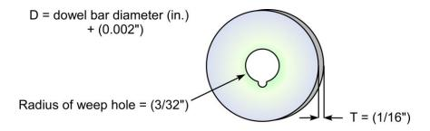
Figure 10.11 Grout Retention Disk
