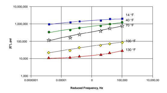
The  $|E^*|$  master curve can be represented by a sigmoidal function as shown (27):
