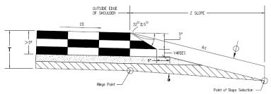
SAFETY EDGE DETAIL FOR HOT MIX ASPHALT PAVEMENT GREATER THAN 5 INCHES
