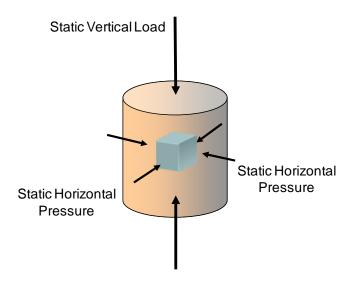
Figure S.25 Resistance R-value Test Specimen Loading State
