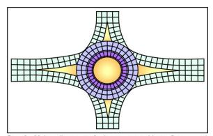
Step 6. Make adjustments for in-pavement objects, fixtures and to eliminate L-shapes, small triangular slabs, etc.
