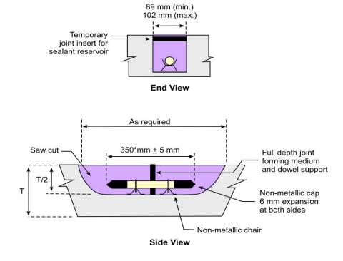
**Note:** For payements with poor support conditions slightly longer bars should be considered.
