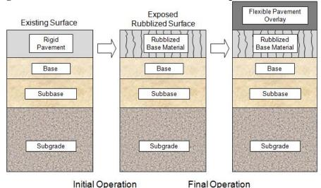
Rubbilization is a fracturing of existing rigid concrete pavement. The rubblized concrete responds as a high-density granular base material.
