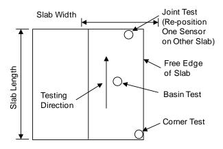
Figure C.3 JPCP Testing Pattern
