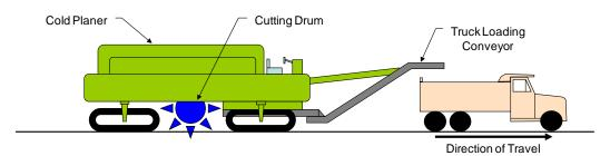
Figure 8.10 Schematic of Cold Planing Equipment
