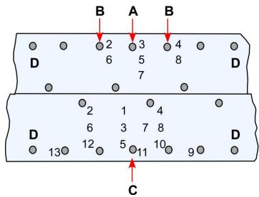
Figure 10.21 Typical Slabjacking Hole Layout
