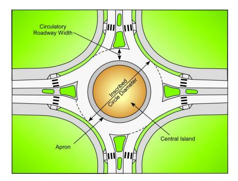
Figure 12.9 Basic Geometric Elements of a Roundabout
