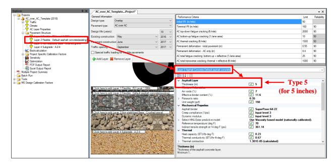
Figure 8.53 Existing Layer Thickness if Milling is Planned
