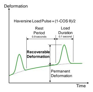
Figure S.23 Resilient Modulus Test Specimen Loading
