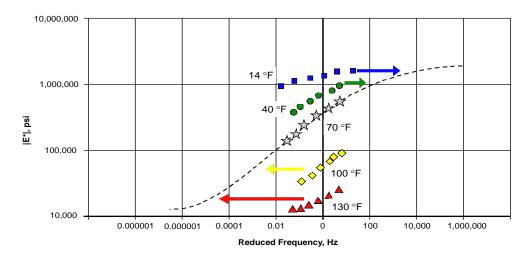
Figure S.10 Shifting of Various Mixture Plots
