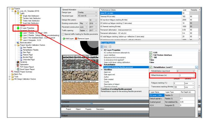
Figure 8.52 Milled Thickness Input Screen
