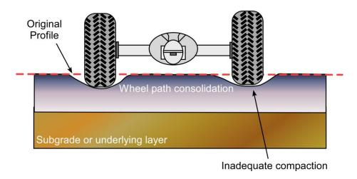
Figure 11.3 Rutting in Asphalt Layer
