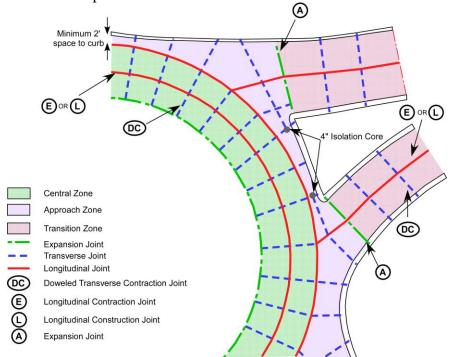
Figure 12.13 Basic Joints and Zones of a Roundabout
