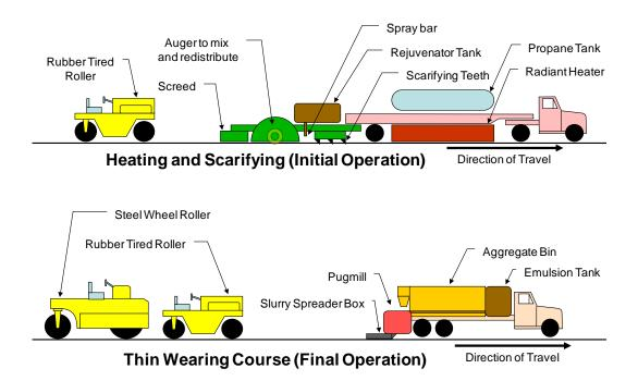
Figure 8.13 Schematic of Surface Recycling Equipment
