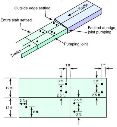
Figure 10.19 Typical Slab Stabilization Hole Layout
