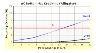
Figure 13.4 AC Bottom-Up Cracking at 98 Percent Reliability
