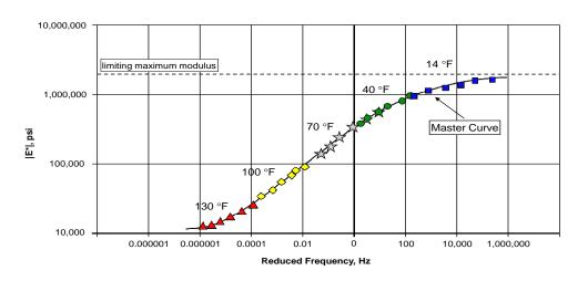
Figure S.11 Dynamic Modulus |E\*| Master Curve
