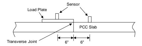
Figure C.4 Joint Transfer Testing Sensor Spacing
