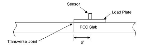
Figure C.5 Corner Testing Sensor Location
