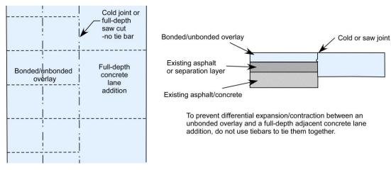
Note: The figure illustrates lane addition details. To prevent cracking related to differential expansion and contraction between a concrete overlay and a full-depth adjacent concrete lane addition, use a butt joint with no tiebars
