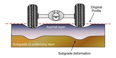
Figure 11.1 Rutting in Subgrade or Base
