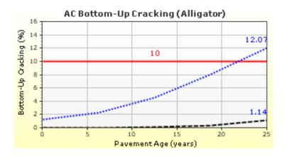
Figure 13.3 AC Bottom-Up Cracking at 92 Percent Reliability
