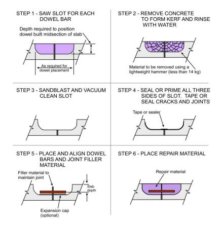
Figure 10.15 Typical Dowel Bar Retrofit Sequencing of the Installation From Figure 4-9.7, Construction Procedures for Retrofitted Dowel Bar Installation Techniques for Pavement Rehabilitation 1998 (6)
