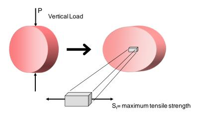
Figure S.18 Indirect Tensile Strength
