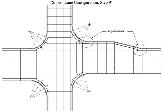
Figure 12.7 Typical Joint Layout for a Rigid Pavement Intersection (Shows Lane Configuration, Step 10)
