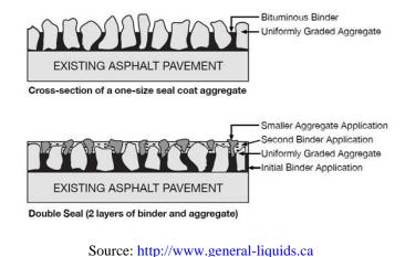
Figure 8.39 Diagram of a Double Chip Seal
