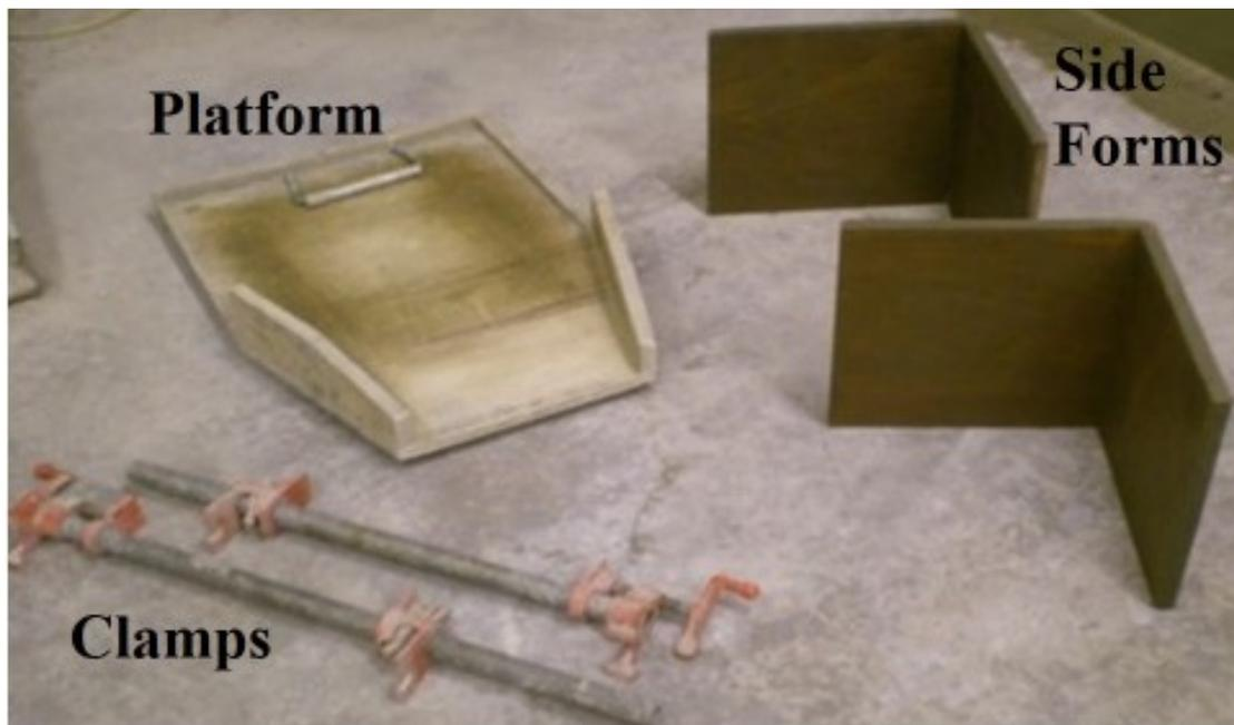
Figure 1 Each Component of the Box Test
