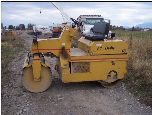
Photographs 7 and 8: Dual drummed steel vibratory roller and rubber-tired pneumatic roller.
