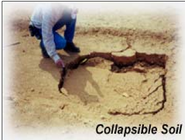
Photograph 20: Sinkhole development as a result of collapsible soil deposits settling at depth.
