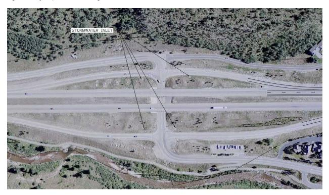
The interchange at MP 190 would not have as drastic an effect on the drainage design, but it could have a wetlands impact of around 50,000 sf (see below).
