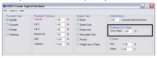
15. **Z-Slopes** are located between the edge of pavement (or the end of the **Bench** when curb is used) and the POSS. The length and slope of the **Z-Slopes** are user defined. To specify the length, use the **Dist** key in field. The slope of this segment is defined with a run over rise ratio. The **Slope** field is used to specify the run portion of the ratio.
