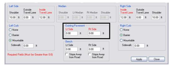
11. A **Bench** is the backfilled area behind a curb. The bench will be placed outside of a sidewalk if one is defined. The **Bench** area is only enabled when either the **Left Curb** and/or the **Right Curb** toggle is set to **Barrier** or **Mountable**. If only one side has a curb specified then only that side's Bench data field will be enabled. By default, a Bench has a 2% slope either towards the road. Toggle on the Slope Away From Road option if desired.
