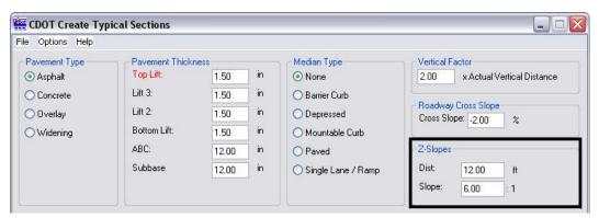
16. After all the desired settings have been entered, select the **Apply** icon to begin placement of the typical section.
