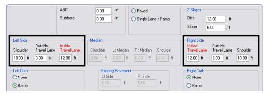
8. The **Left Curb** and **Right Curb** areas are use to define the presence and type of curb. If a curb is present, then a sidewalk can be specified. Turn on the desired toggle to on the desired curb type. If **Barrier** or **Mountable** is selected a sidewalk can be defined by entering a width in the key in field.
