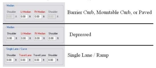
The **Lt. Median** and **Rt. Median** fields require data with a value greater than zero when present as does one **Travel Lane** field for **Single Lane / Ramp** typical sections.
