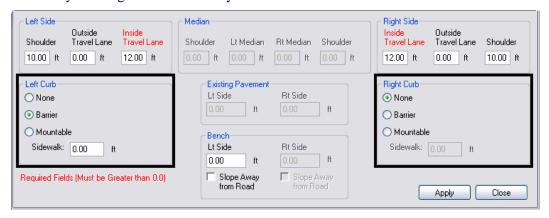
**Note:** Unlike the **Left Side** and **Right Side** areas, **Left Curb** and **Right Curb** are enabled when the **Single Lane / Ramp** median type is selected.
