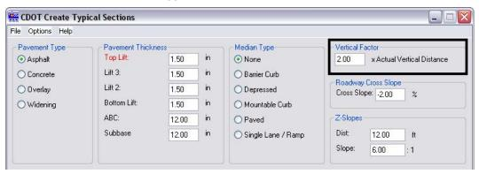
13. The **Roadway Cross Slope** determines the percent of slope used on travel lanes and shoulders. This is measured from the center of the typical section out to the end of the shoulder. A negative slope drops down from the center of the typical section and a positive number rises above the center point.
