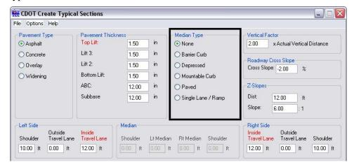
7. The Left Side and Right Side areas are use to define the number and width of driving lanes and the presence and width of a shoulder. With all median types, except Single Lane / Ramp, the Inside Travel Lane must contain a value greater than zero. If the Single Lane / Ramp median type is selected, these fields are disabled.
