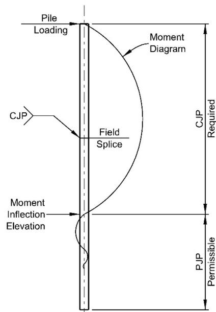
**Figure 10-2: Moment Inflection Point and H-Pile Field Splices**
