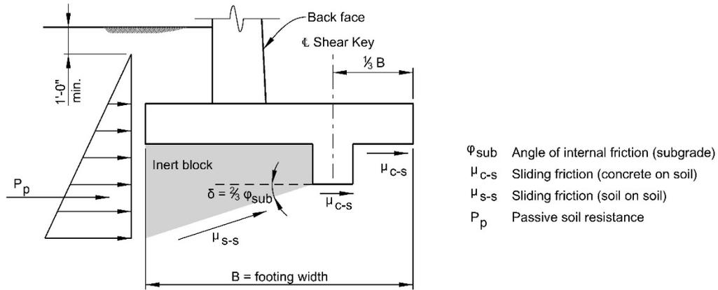
Figure 11-15: Shear Key
