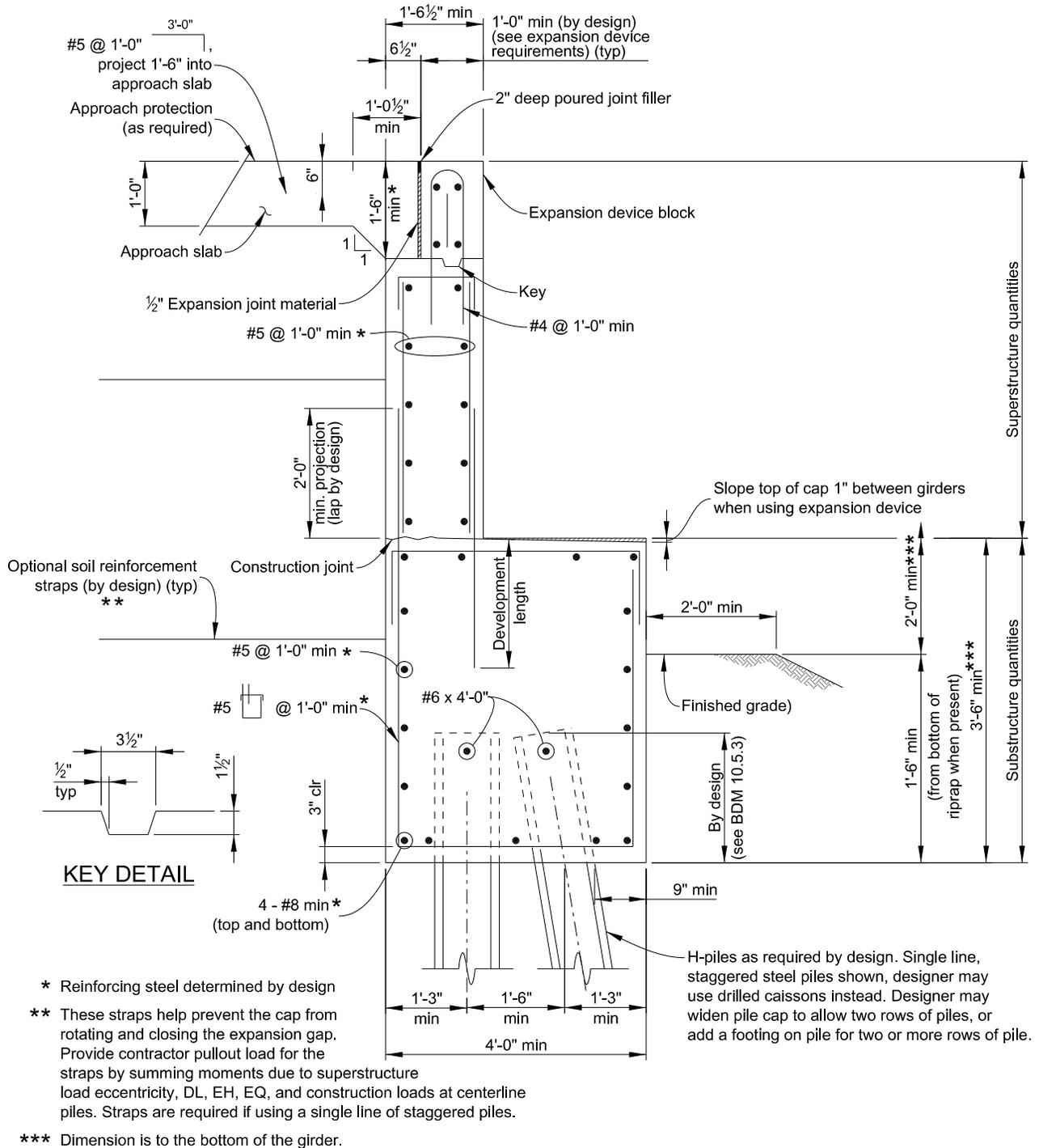
Figure 11-5: Seat Type Abutment
