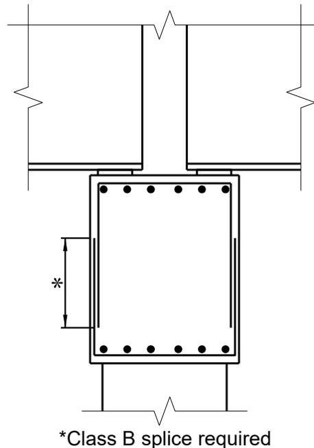
**Figure 5-5: Pier Caps in Precast Girder Bridges with Variable-Depth Cap
