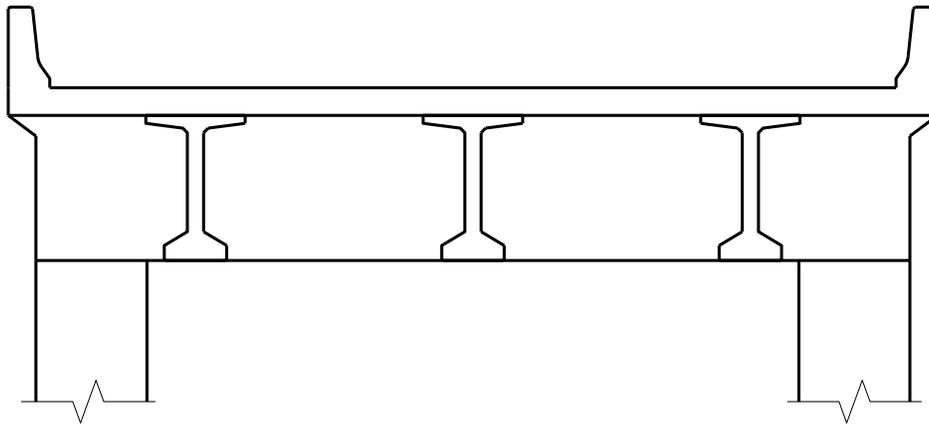
**Figure 5-10: Indirect Support/Loading – Integral Pier Cap**
