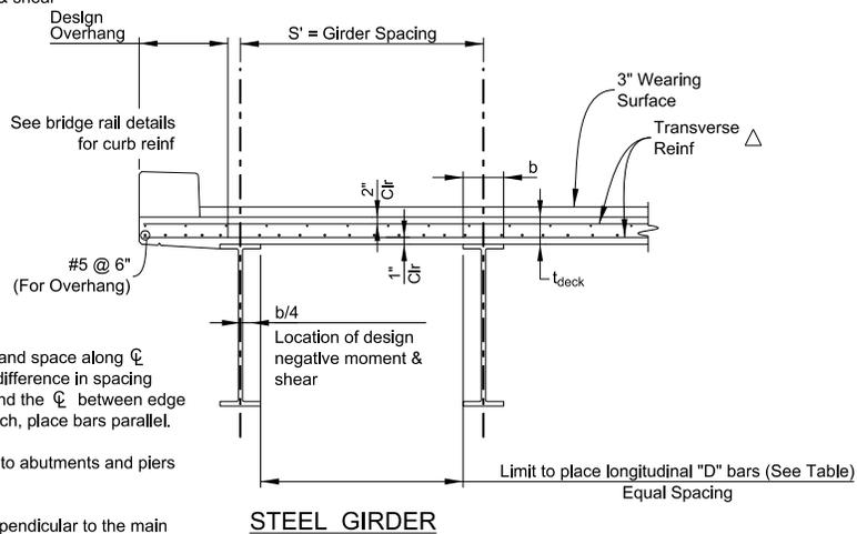
$\Delta$  For curved structures place radially and space along  $\bar{O}$  between edges of deck. When the difference in spacing between the outside edge of deck and the  $\bar{O}$  between edge of deck becomes greater than 1/4 inch, place bars parallel.
