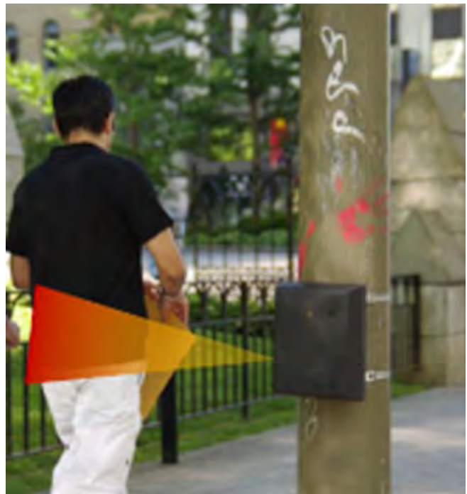
Figure A-2. Example of Passive IR Device Mounted at Sidewalk Location
