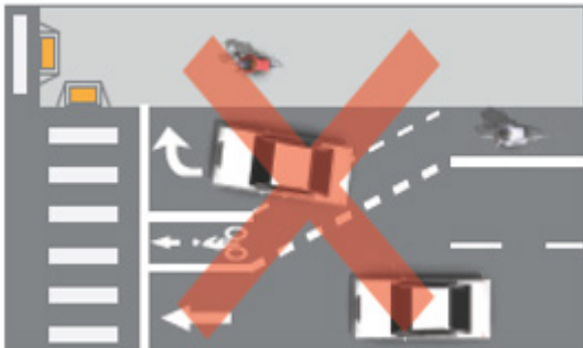
Bicyclists are not provided priority in weaving area and must use caution to merge across motor vehicle traffic. Dotted line transition areas should not be provided in these locations due to confusing geometry.
