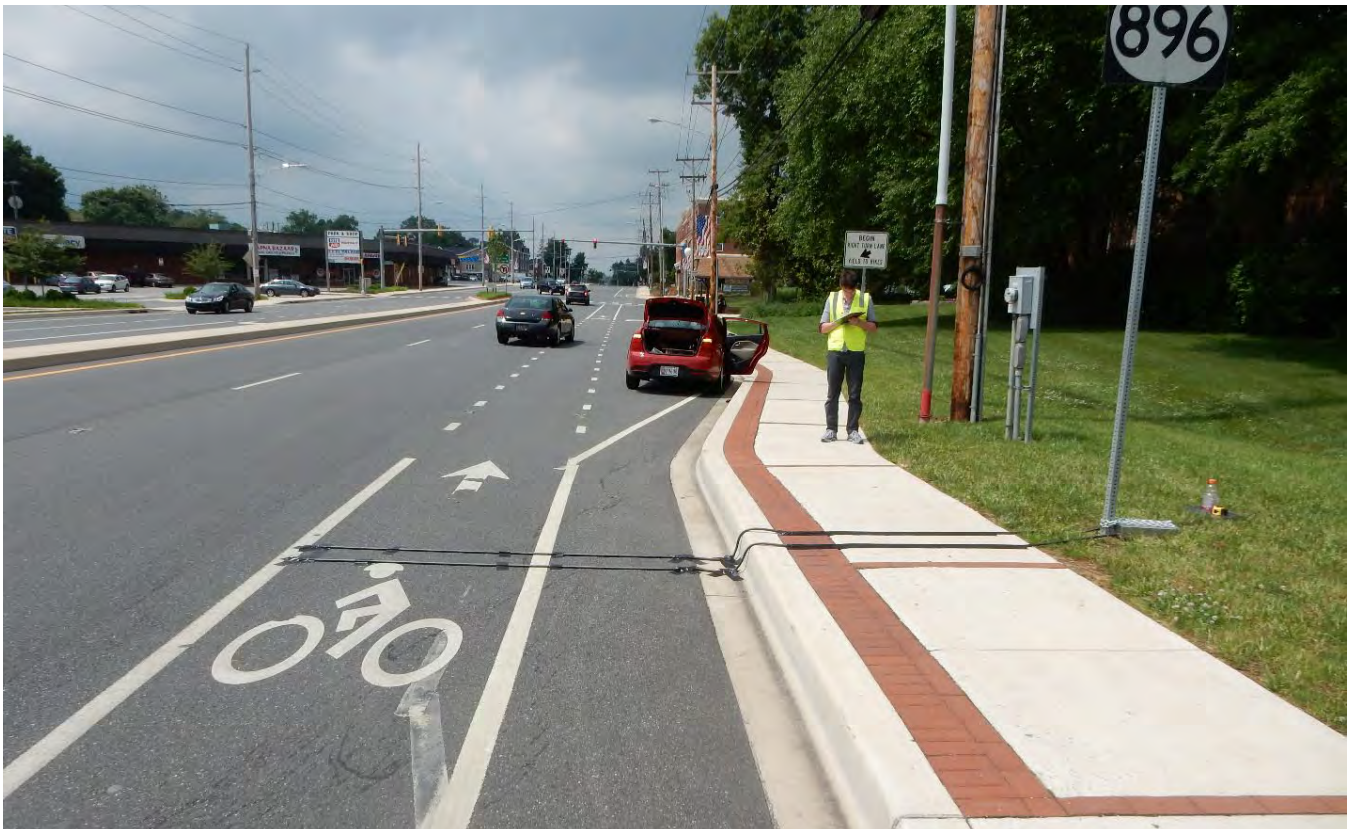
Figure A-5. Pneumatic Tube Installation on a Bicycle Lane
