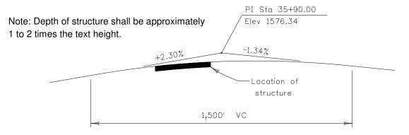
Figure 6.5-1 Typical Profile Grade Diagram
