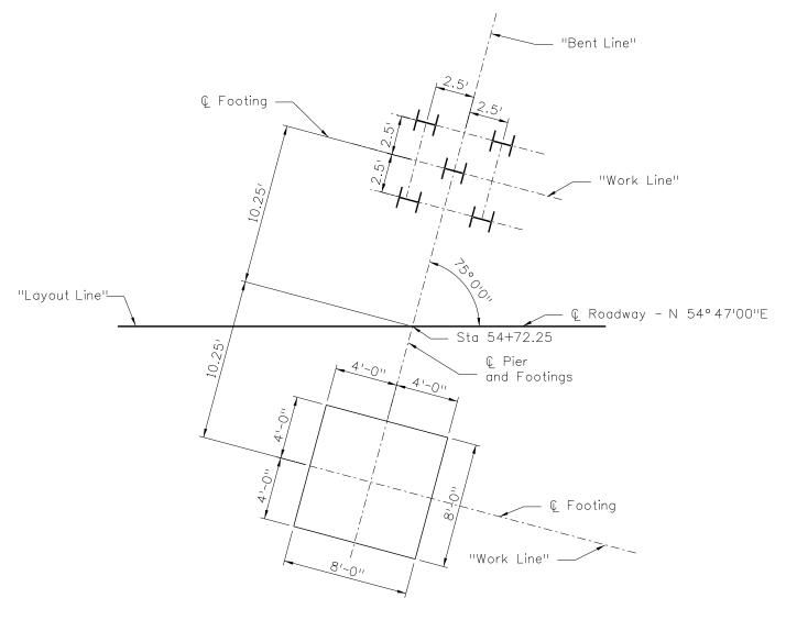
Fig. 10.5-1 Detail of Layout, Bent, and Work Lines
