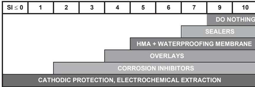
**Figure 33-2: Optimal Corrosion Control Based on Susceptibility Index**
