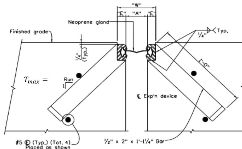
**FIGURE 1 - BRIDGE EXPANSION DEVICE (0 - 4 INCH)**
