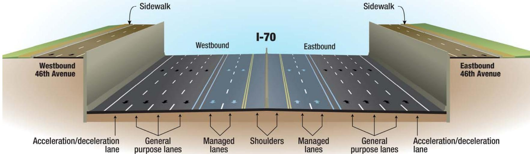
*Note: Ultimate typical section width will be constructed as shown. Phase 1 striping will only include (1) Tolloed Express Lane in each direction*
