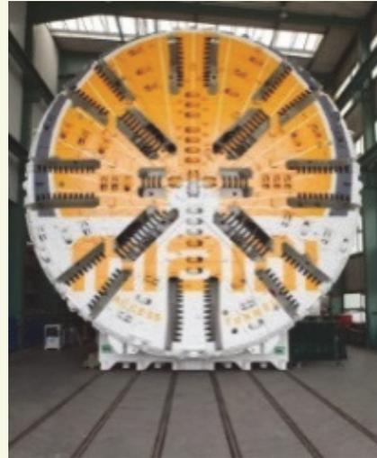
*MAT's tunnel boring machine manufactured specifically for POMT*
