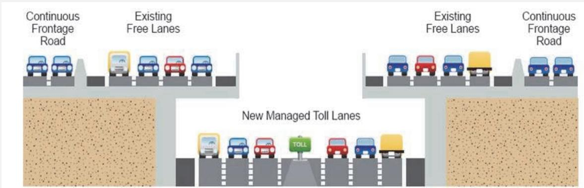
*Cross section at cut and partial cover echoes the scope of I-70 East*
