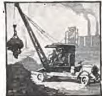
Equipped with electric magnet—metal parts, scrap iron, etc., quickly and easily moved about.
