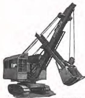
P & H 206— $\frac{3}{4}$ -yd. Shovel which may be converted into dragline, clam shell bucket crane, back-filler and pile-driver by removing shovel boom.
