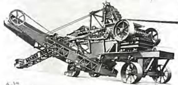
Heavy duty portable screening, crushing and loading plants. Built to stand up under the severest conditions and produce large yardage.
