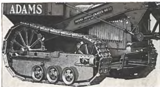
No. 12 has Trackson Full Crawlers to meet the requirements of exceptionally soft going on dirt roads.
