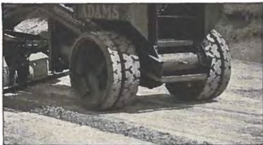
No. 10 is furnished with 6-inch wheel extensions as extra equipment to increase tire width to 16 inches if desired.
