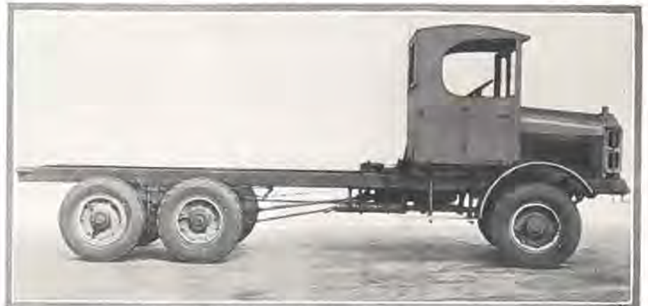
New six-wheel type FWD truck designed to carry the heaviest loads without damage to modern pavements.
