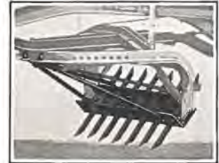
Above: ADAMS scarifier attachment fits in place of moldboard on graders where scarifier is not permanently attached ahead of the blade.
