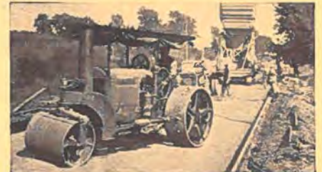
A 6-ton roller in which are seen the familiar lines of the McCormick-Deering power plant. Effective combinations of equipment with this power are almost limitless.
