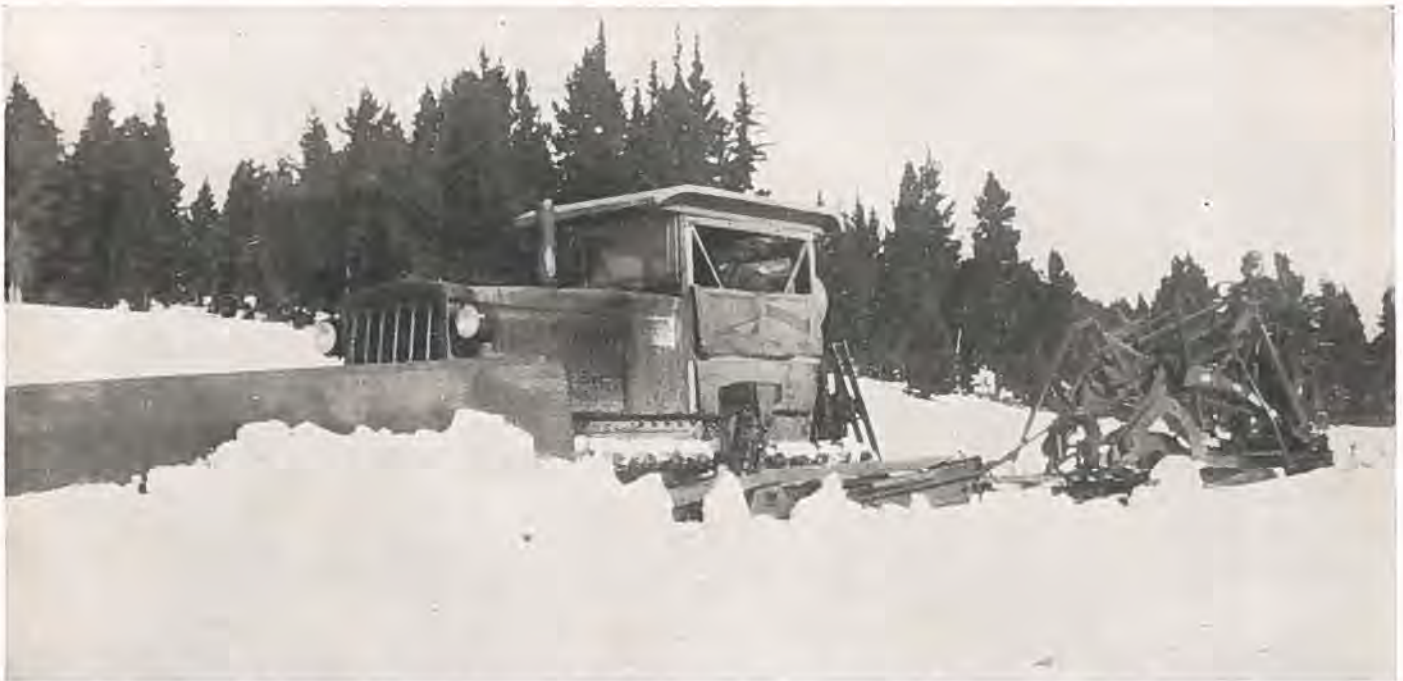
State maintenance tractor-grader outfit, equipped with snowplow, clearing snow from Tennessee Pass—to keep traffic moving throughout the winter months at 10,000 feet altitude.
