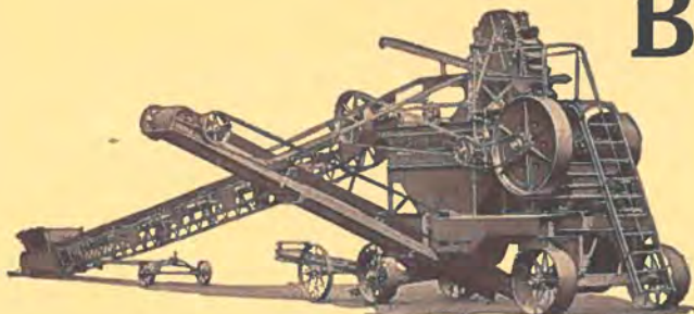
PIONEER SCREENING, CRUSHING AND LOADING PLANT, No. 60
