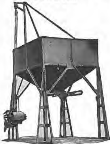
21-yard "Pioneer" Bin made of No. 10 gauge steel, riveted and reinforced, equipped with structural steel legs with built-in lifting jacks—one man operated. Bottom opening is 19 inches square, with sliding shutters. Will fill truck almost instantly. Easily moved.
