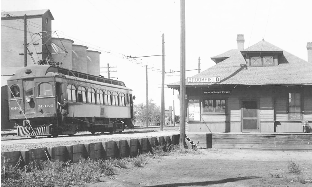
Figure 114. D&I car outside of the Broomfield Depot, originally located at West 120 th Avenue and the C&S tracks. Note the diamond-shaped pantograph atop the car. 542
