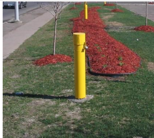
Figure 4.25. Above-Grade Completion of a Groundwater Monitoring Well
