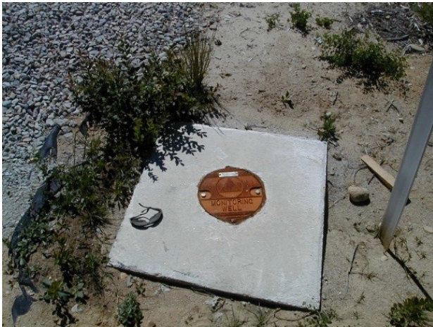
Figure 4.24. Flush-Mounted Surface Completion of a Groundwater Monitoring Well
