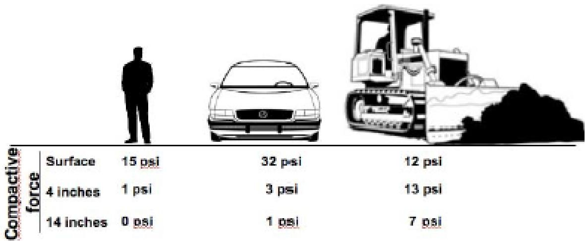
The above diagram above illustrates the compactive forces of foot traffic, a car, and construction equipment. At the surface, the compact forces of equipment and a human is similar, but equipment has a greater impact below the surface where it compacts the void spaces between soil particles. Source: Larry Morris, University of Georgia.
