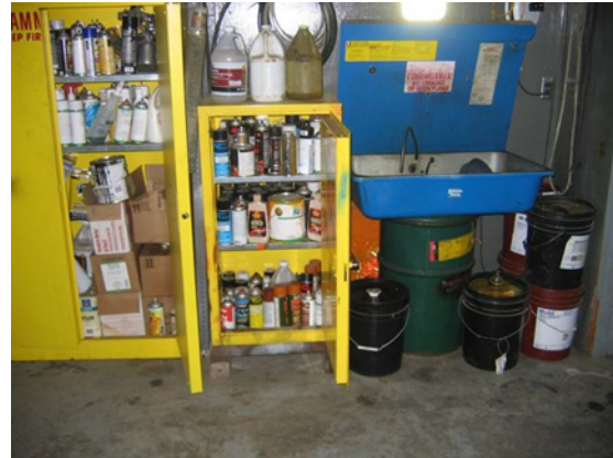
Multiple aerosols, paint cans, 5-gallon buckets, and a parts washer with a 30-gallon drum.
