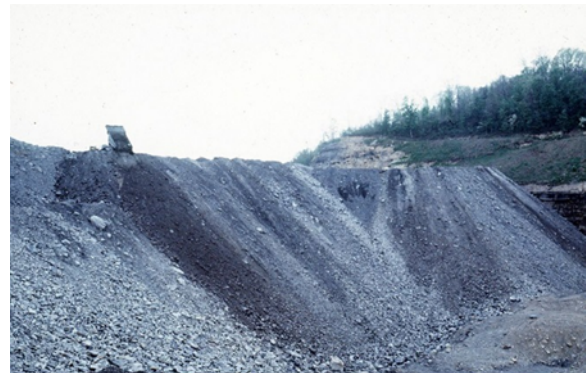
Trucks dumping mining waste at the edge of stockpiles.
