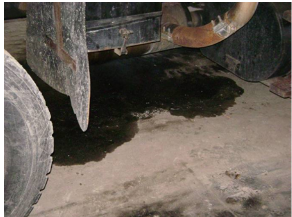
Surficial staining from a leaking vehicle. Presumably, motor oil, but other possibilities include antifreeze, transmission fluid, etc.
