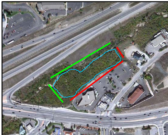
Figure 33. A FACWet test site on Straight Cr. in Summit County, along the I-70 corridor. The blue outlined polygon is the AA. Green lines indicate where buffer land cover exceeds 5m in width. Red lines mark where no buffer exists. Fifty-two percent of this test site had buffer, placing it at the bottom of the functioning category ( \sim 0.72 ).
