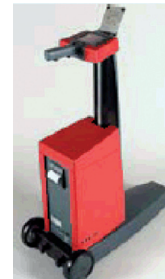
The pavement marking retroreflectometer purchased was a Delta LTL-X
