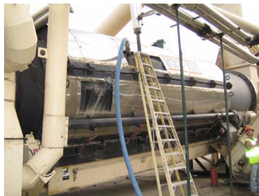
Figure 5 Feeding Advera WMA through Fiber Feed Line
