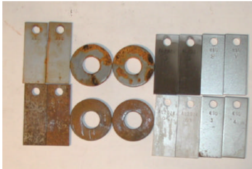
Fig. 2-10 Coupons exposed to distilled water (Upper: from the NACE test of 109 days, lower: from the SAE test of 81 days)
