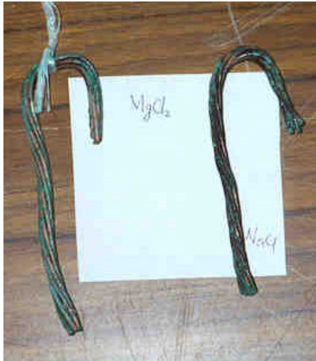
Figure 14: Corroded copper wires after SAE J2334 testing
