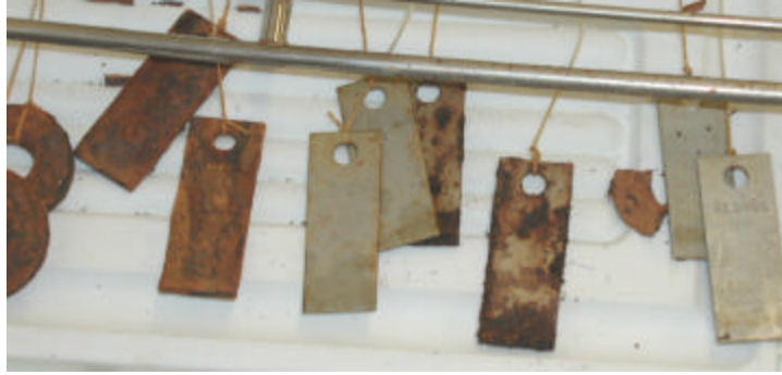
Fig. 2-12 The coupons of the SAE test at 20 days
