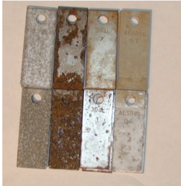
Fig.2-17 Coupons after the SAE test (Upper: exposed to the NaCl solution, lower: exposed to the MgCl 2 solution)
