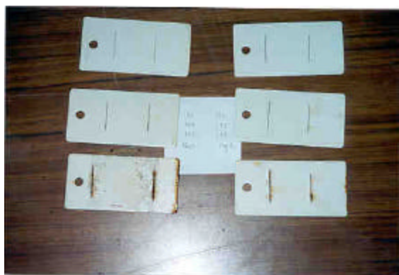
Figure 8: Coupons Corroded by a mixture of \text{NaCl} and \text{MgCl}_2 (practical salts)
