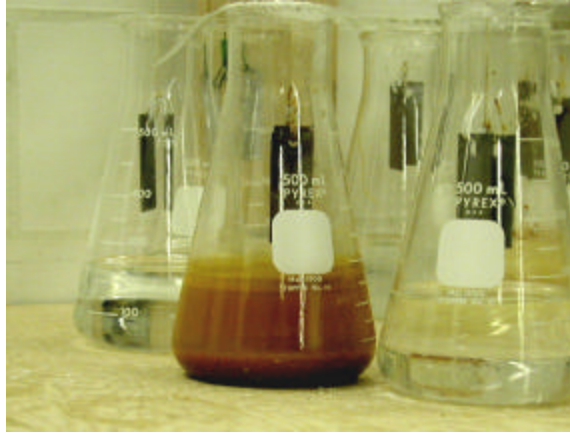
Fig. 2-11a. The NaCl solution in the NACE test (at 69 days)
