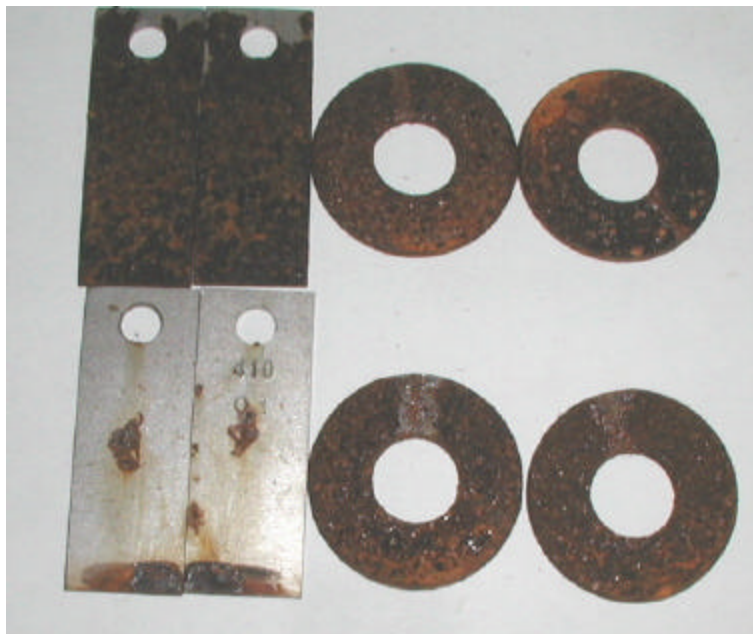
Fig. 2-24a Coupons by the SAE test without the dry stage after 7 days (upper: by MgCl_2 ; lower: by NaCl)
