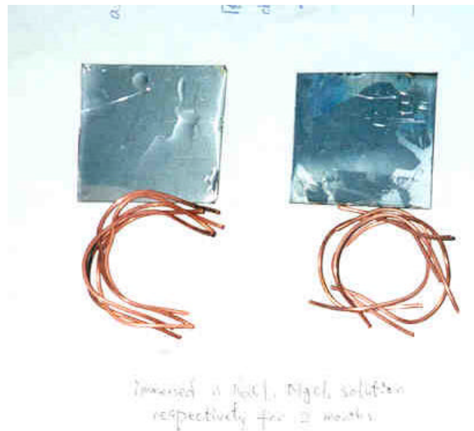
Figure 13: Immersion tests of SS410 and copper wires.
