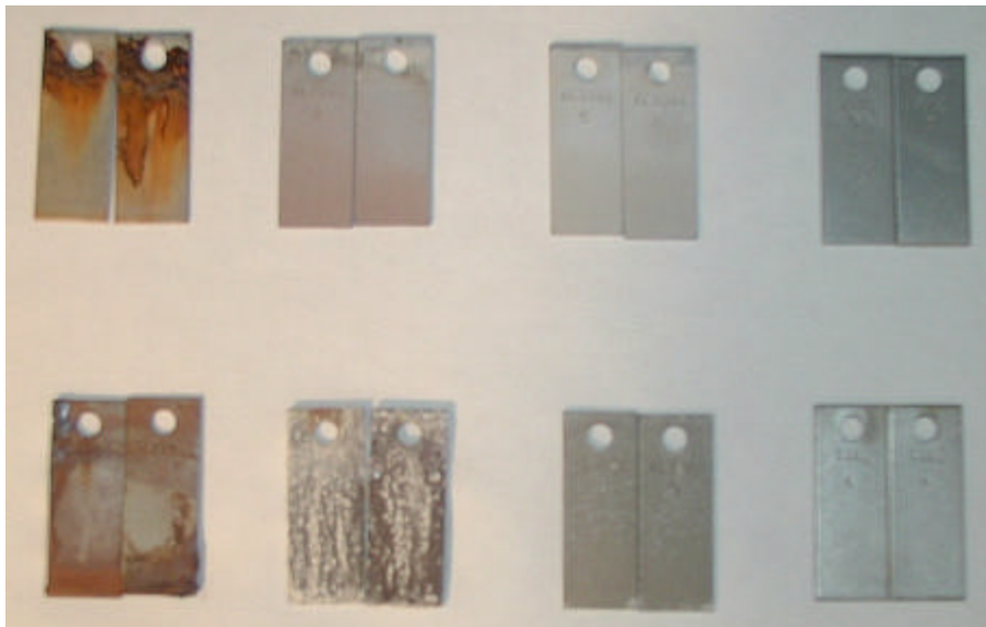
Fig. 2-16 Coupons after the NACE test (Upper: exposed to the MgCl 2 solution, lower: exposed to the NaCl solution)
