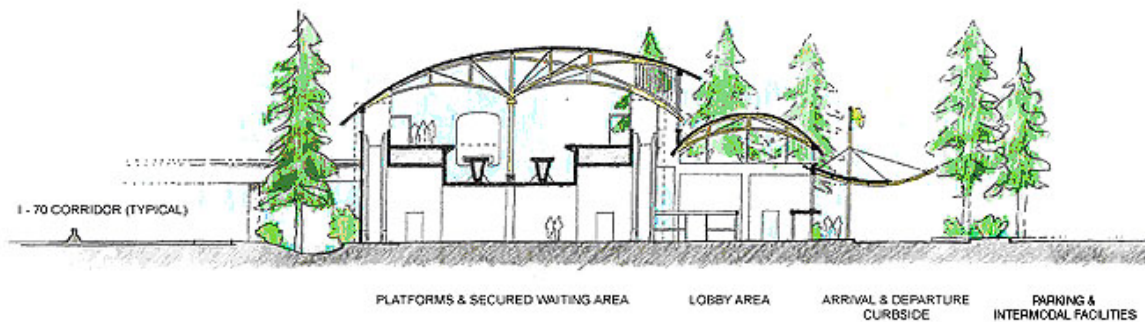
Figure 75: Maglev Station Prototype: Cross-Section
