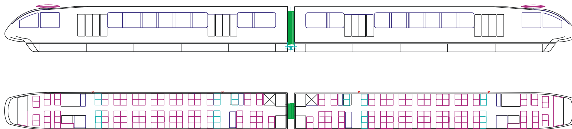
Figure 13: Colorado 200 Vehicle Interior Layout
