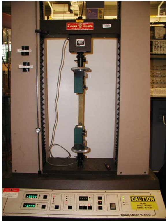
Figure 6. Experimental setup for uniaxial tension test of a GFRP specimen
