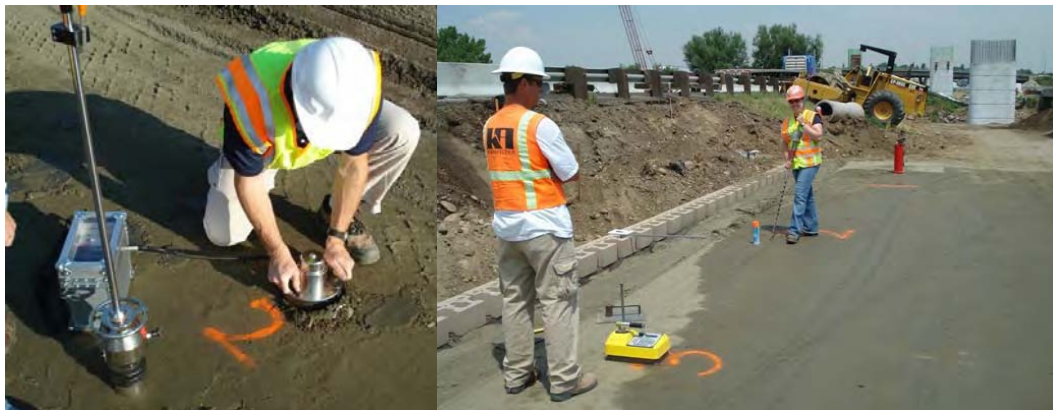
Figure 3-3. DCP and Clegg Impact Hammer Operation
