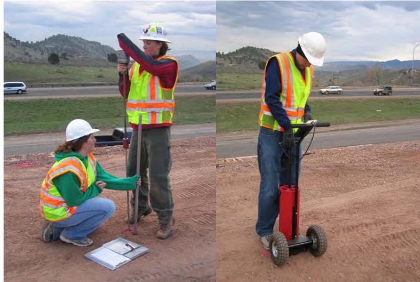
Figure 3-3. DCP and Clegg Impact Hammer Operation
