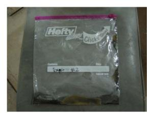
Figure 29. Sediment collected from the gutters and catchment box following a pollutant runoff experiment.
