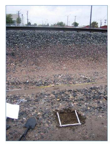
Figure 15. Soil sampling at the toe of ballasted tracks near Broadway Light Rail Station, east of I-25.
