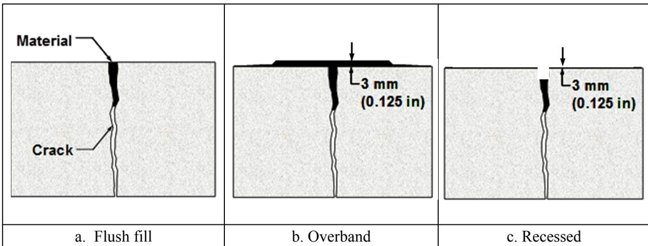
Figure 20. Commonly used CDOT crack sealing configurations.
