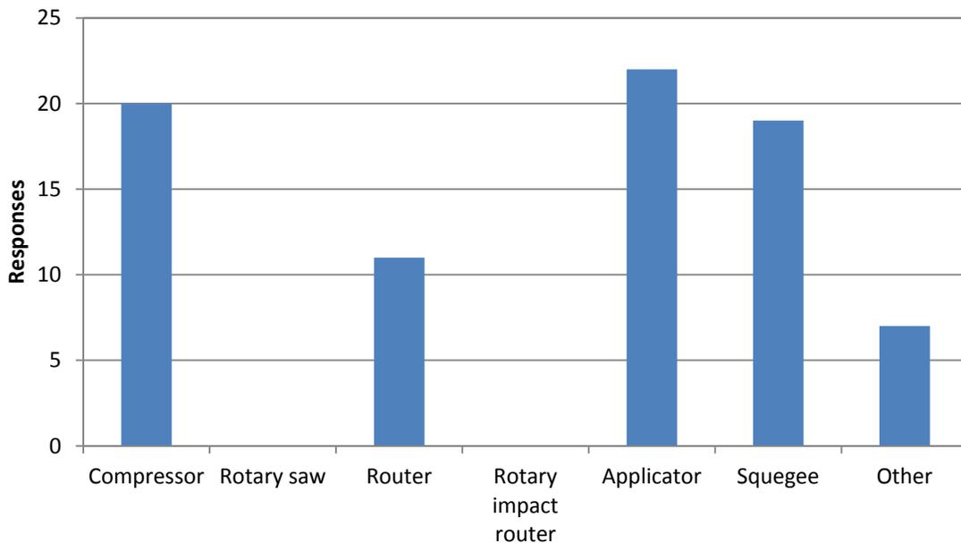
Figure 13. Typical equipment used in the crack sealing process from survey responses.
