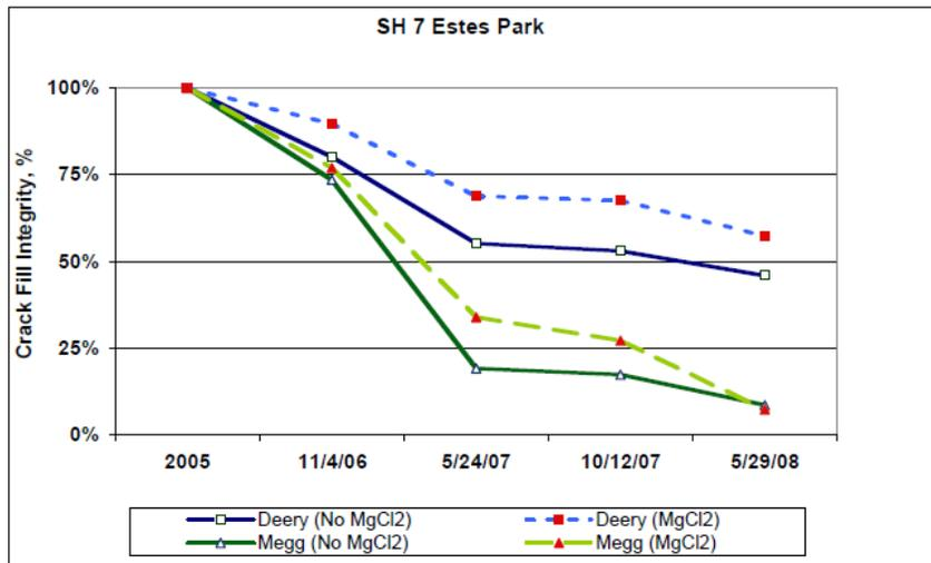
Figure 16. Crack seal effectiveness over time at SH 7 Estes Park (Shuler 2010).
