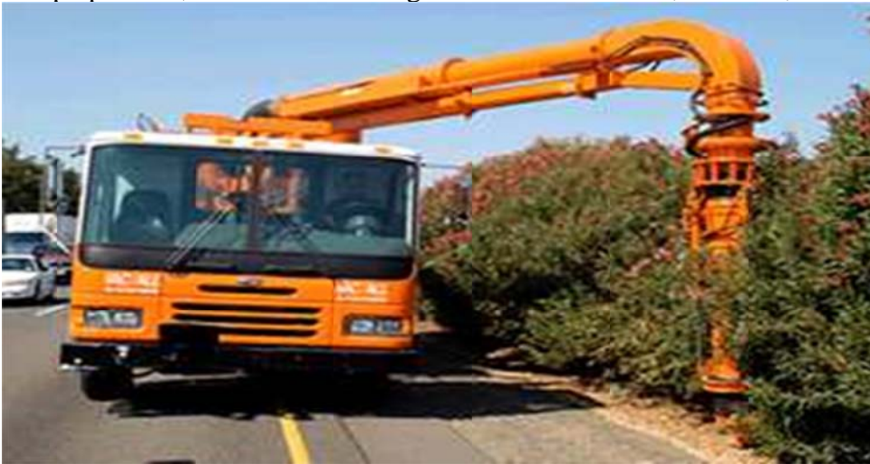
Figure 2: Automated Litter Bag/Debris Collection Vehicle
