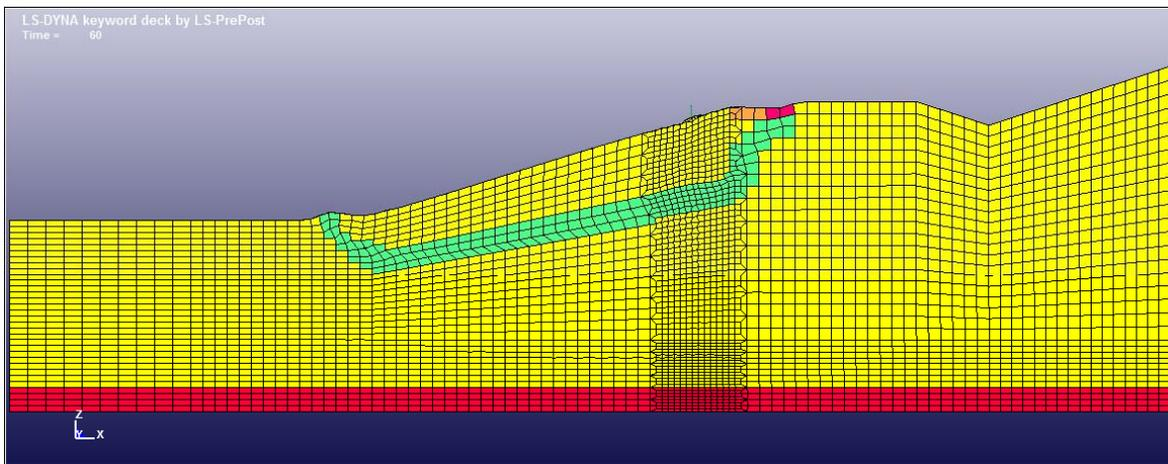
(B): Mitigation based on HP 14x102 driven piles spaced at 5 ft.
