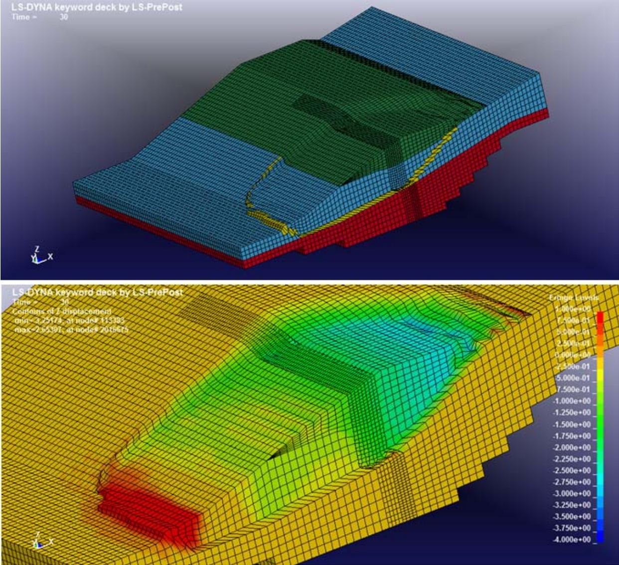
Figure 6: Failed 3-D slope before mitigation and contours of vertical deformation
