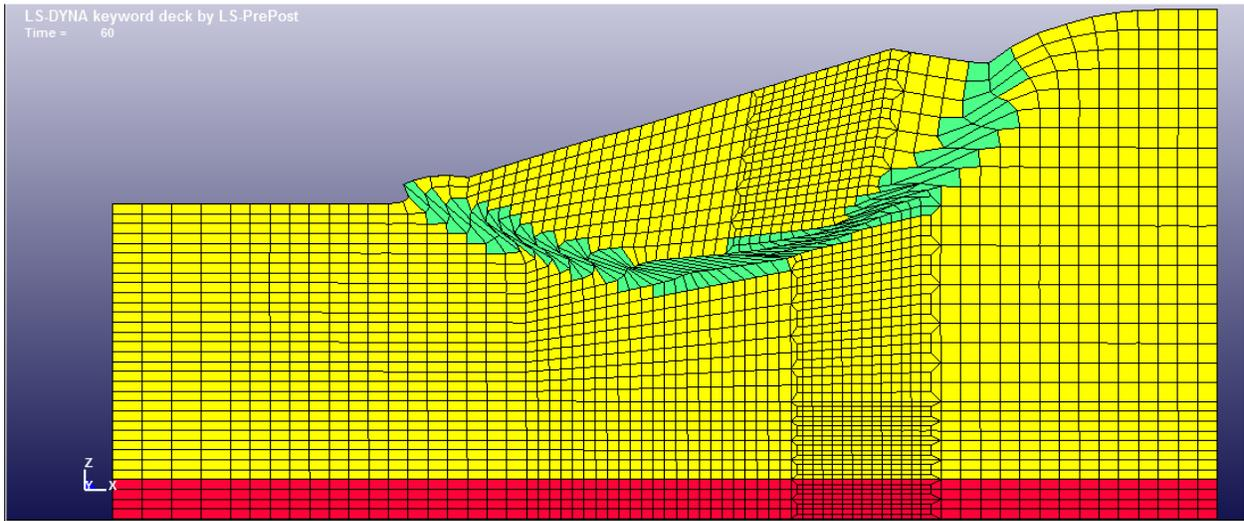
(B): Unmitigated failure of a 2:1 slope embankment
