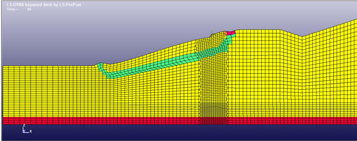
(A): Mitigation based on HP 12x53 driven piles spaced at 5 ft.
