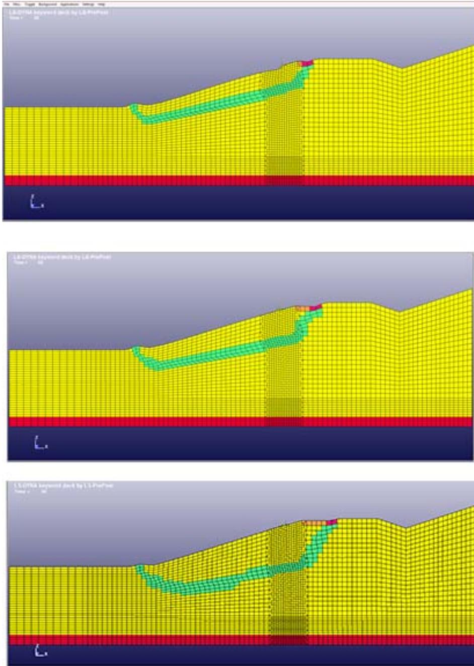
**Figure 1: Embankments with 3:1 slope and varying depths of the failure zone**
