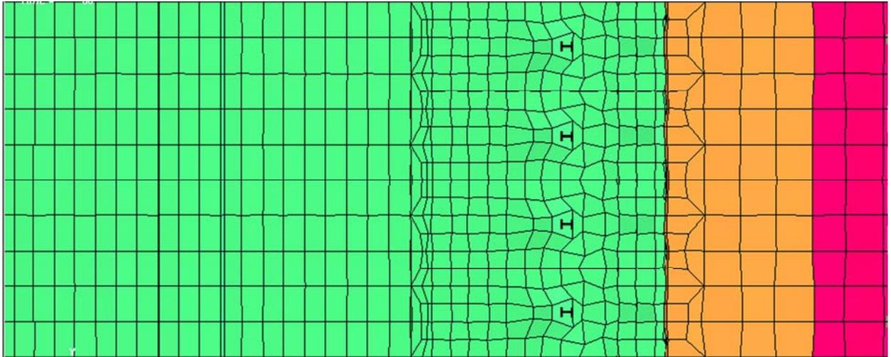
**Figure 19: Soil flow between driven piles**
