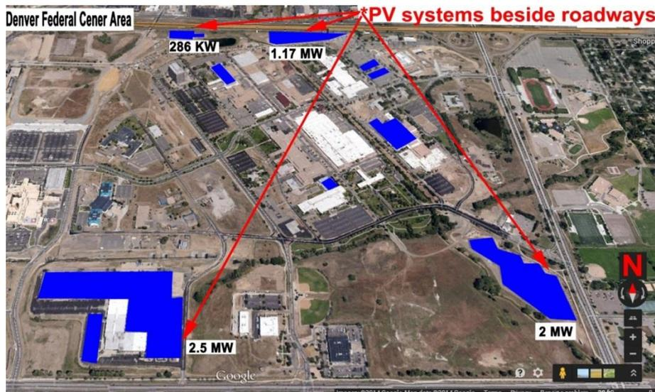
As shown in Figure 7, four PV array sites are located beside roadways; consequently, due to adjacency to roadways, inevitable impacts on motorists such as glare may cause driver distraction. For illustration, a PV array sited near the bridge adjacent to highway US-6 is shown in Figure 8. Glare from the PV array adjacent
