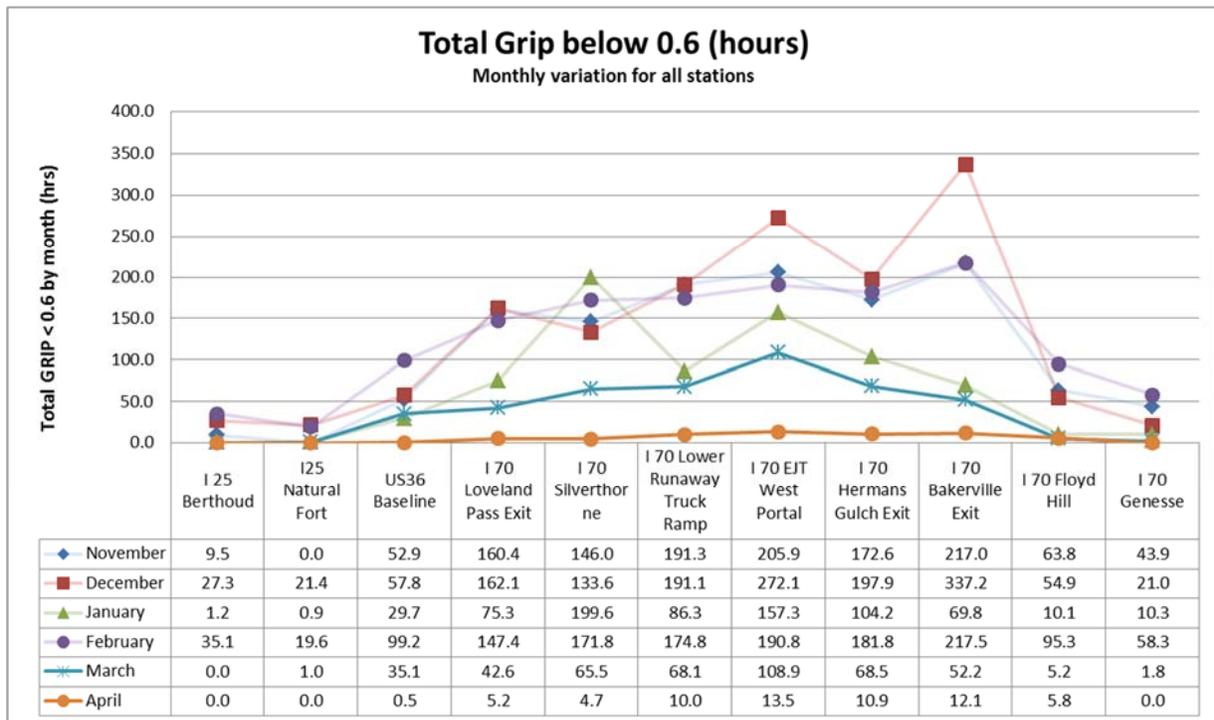
Graph 7: Monthly breakdown of hours that RWIS measured GRIP falling to less than 0.6
