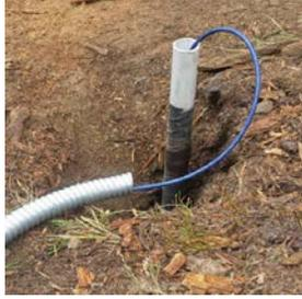
**Figure C.12 Piezometer placed in borehole**
