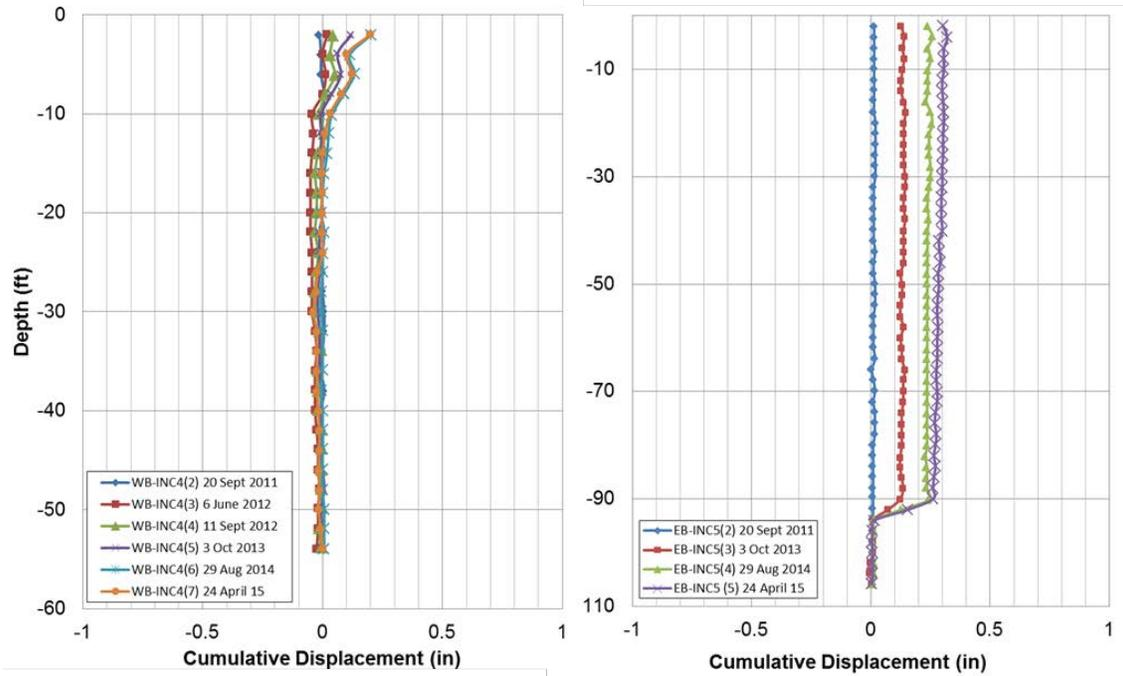
**Figure 5. Inclinometer data from 2011-2015 (a) INC4 along the westbound shoulder and (b) INC5 along the eastbound shoulder (CDOT, 2015).**
