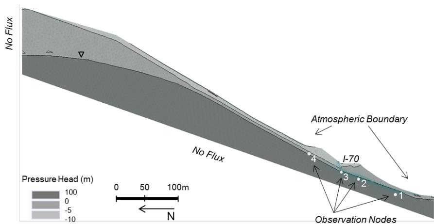
**Figure 10. Numerical model domain: boundary conditions, initial conditions, and observation nodes.**
