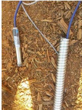
**Figure C.10 Piezometer cable protected with aluminum conduit**
