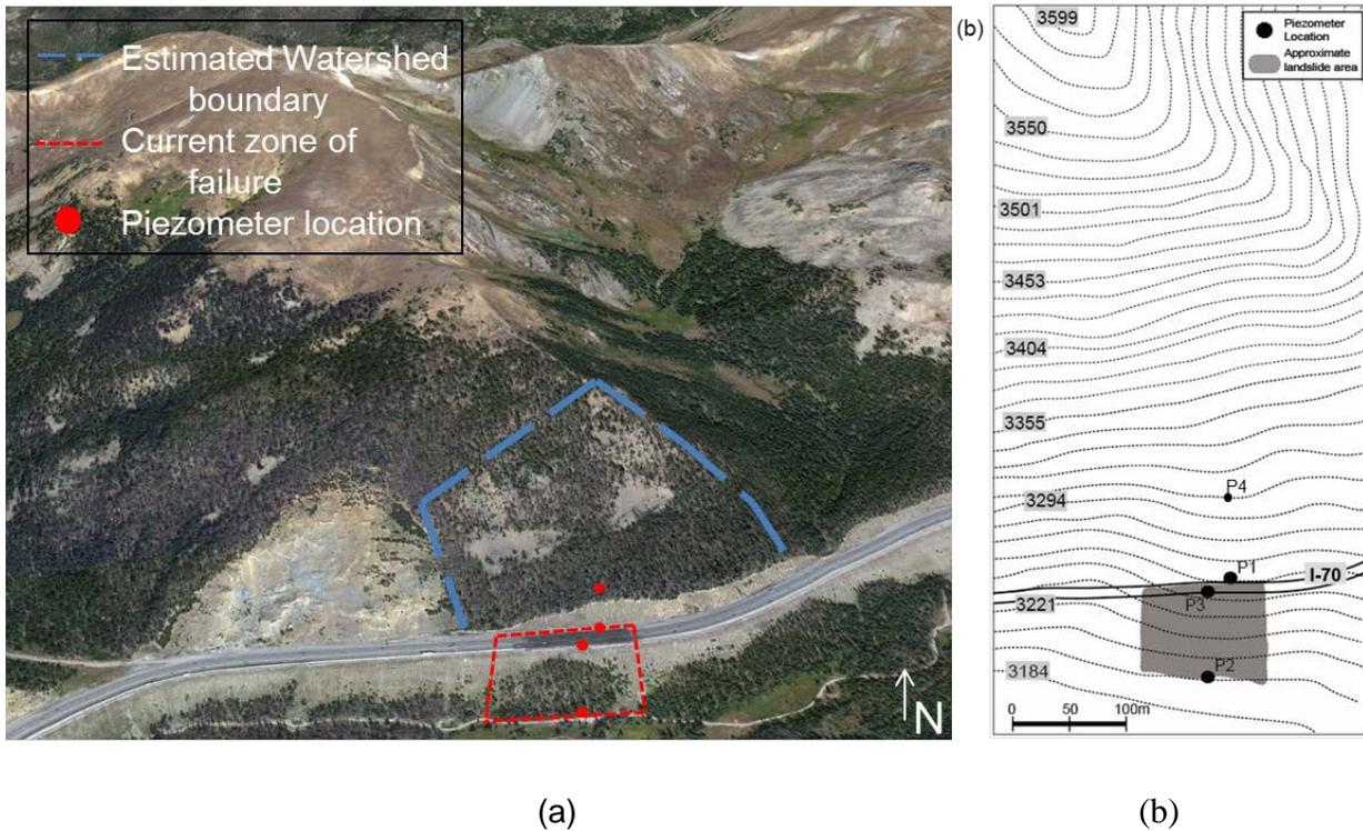
**Figure 1. (a) Plan view of estimated watershed area, (b) contour map of area and piezometers location.**
