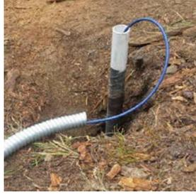
**Figure C.12 Piezometer placed in borehole**
