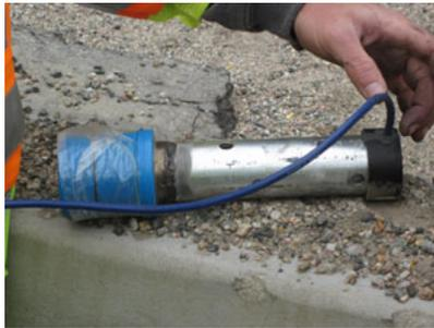
**Figure C.5. Piezometer installed in a cage on the tip of the inclinometer casing**
