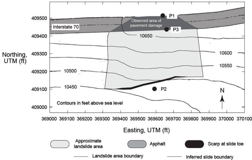
**Figure 3. Plan view of GPS mapped landslide.**
