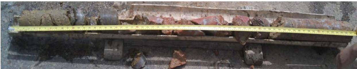
**Figure C.3. Sharp transition between clay/weathered bedrock layer and bedrock at 91.5 ft**
