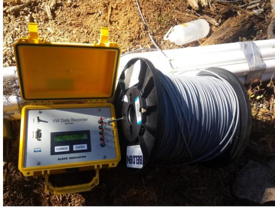
**Figure C.9 Field calibration and accuracy check of piezometer in borehole**
