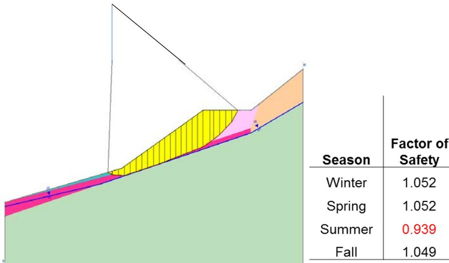
**Figure 16. Stability analysis using modified Bishop's method that accounts for suction stress**
