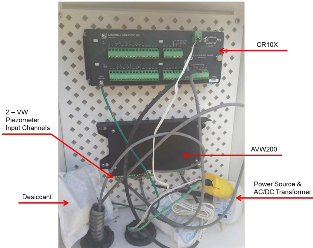
**Figure C.6. Sample datalogger field setup with CR10X and AVW200 sampling 2 VW piezometers**
