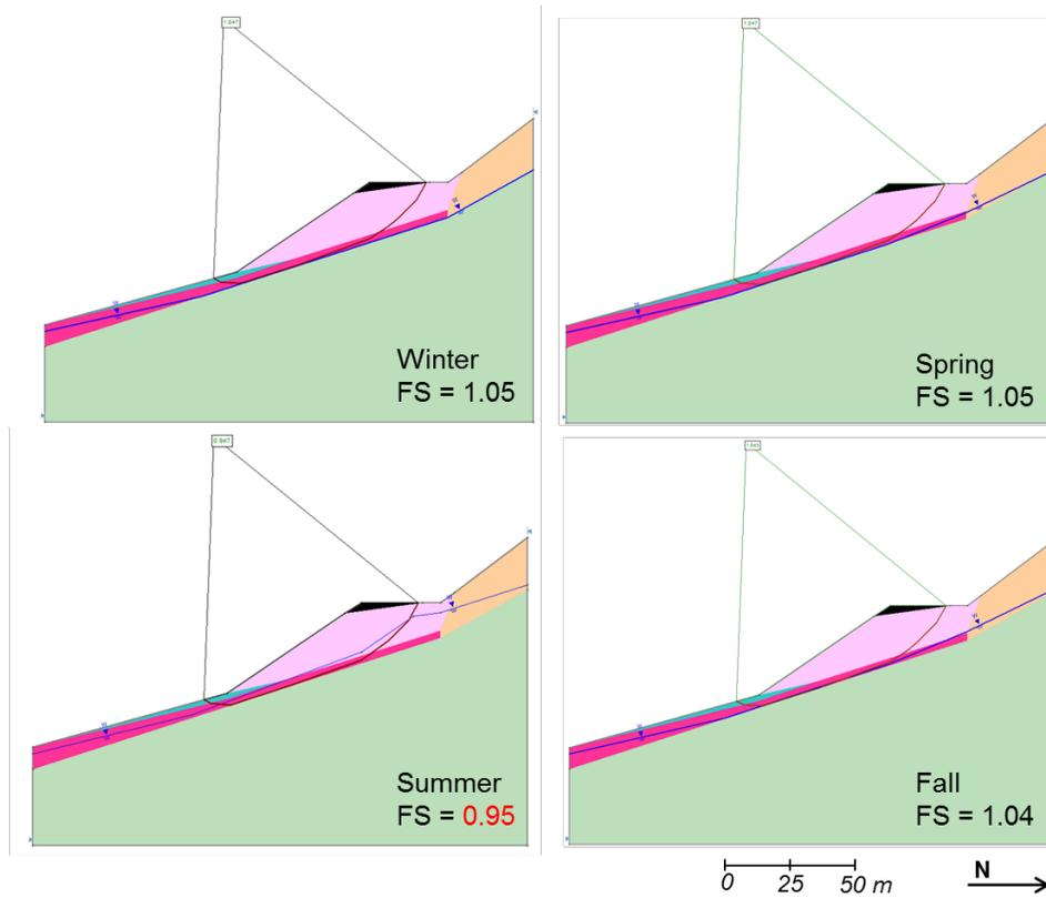
**Figure 14. Slope stability results using Modified Bishop's method of slices**
