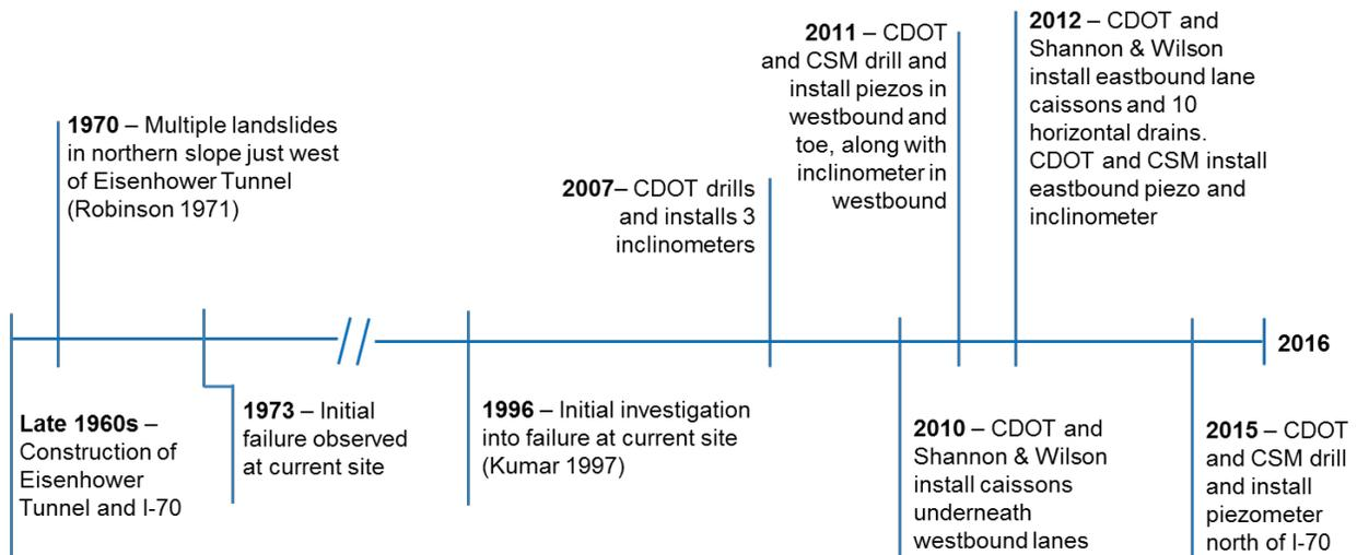
**Figure 2. Timeline of work performed on site since construction of I-70.**
