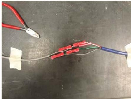
**Figure C.8 Piezometer cable splicing in laboratory**
