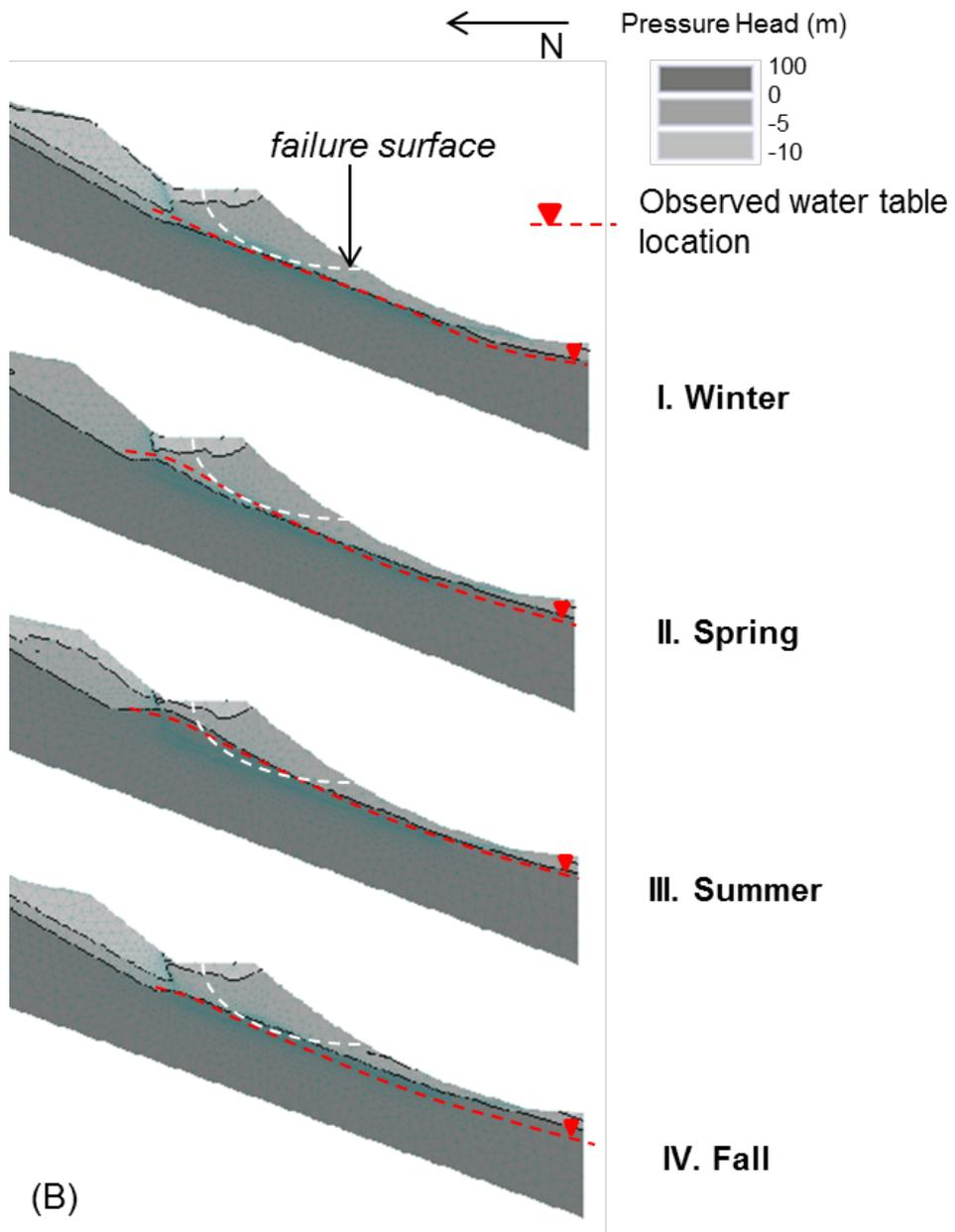
**Figure 13. (a) Simulated pore water pressure distribution throughout the watershed and (b) simulated water table near I-70 compared with observed water table during each conceptual model stage over the course of one year.**
