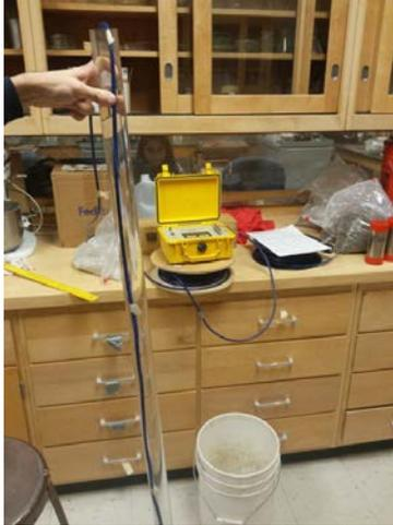
**Figure C.7 Laboratory calibration of vibrating-wire piezometer**
