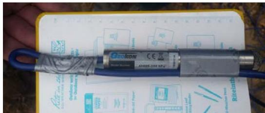
**Figure C.11 Piezometer oriented to stay tip-up when installed in borehole**
