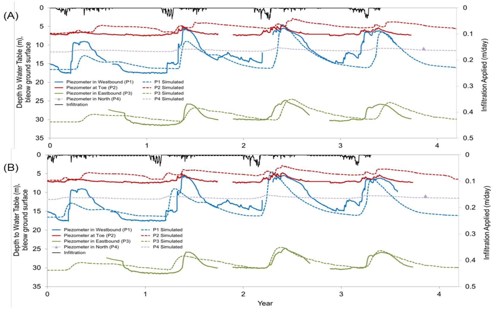
**Figure 5.5 Comparison of field measurements and simulation results of ground water table elevations at observation points with (a) original infiltration data from Grizzily Peak SNOTEL and (b) infiltration data timing adjusted to match water table response in simulation to observe water table behavior**
