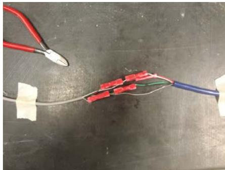
**Figure C.8 Piezometer cable splicing in laboratory**
