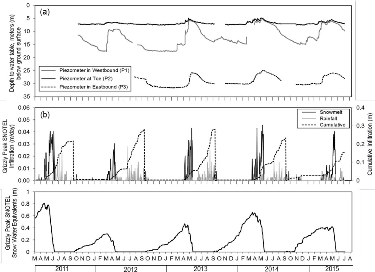
**Figure 7. (a) 4 years of piezometer data, (b) infiltration data from Grizzly Peak, and (c) snow water equivalent data from Grizzly Peak.**
