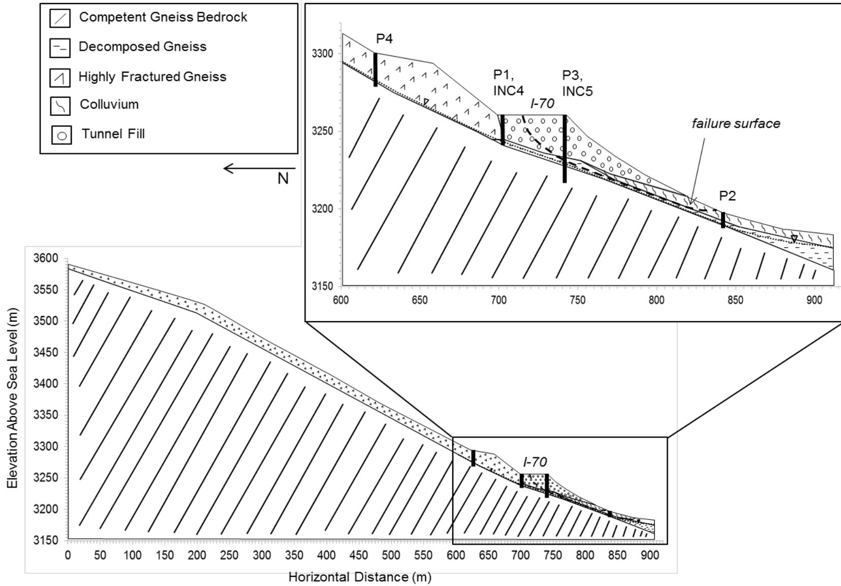
Figure 4. Geologic cross section with instrumentation, boreholes, and failure surface.
