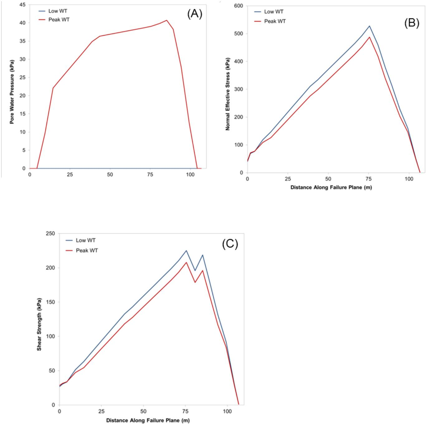
**Figure 15. (a) pore water pressure, (b) effective stress, and (c) shear strength along the failure surface from toe to scarp during peak summer flow and low winter flow conditions**
