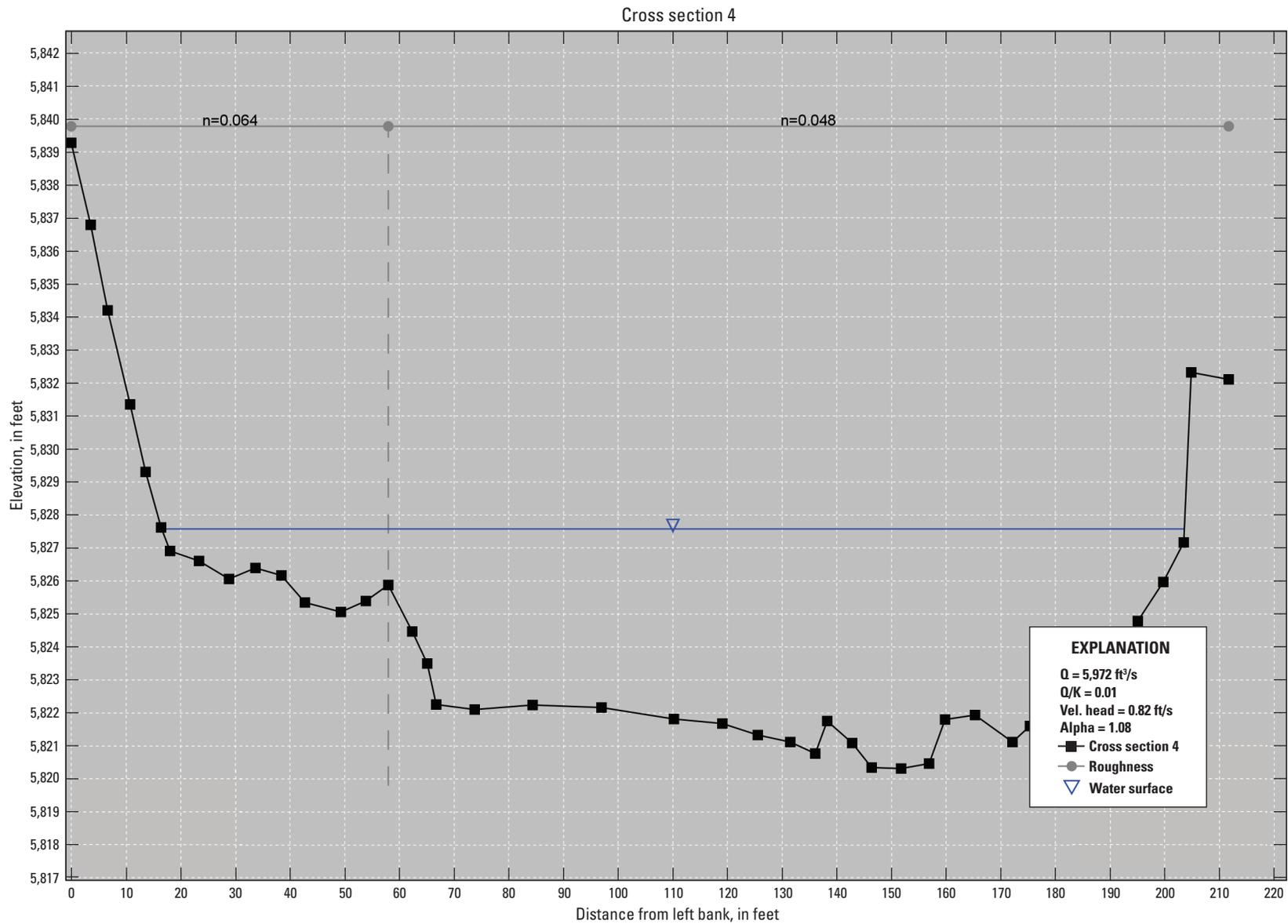
**Figure 10-4.** Cross section 4 with the Manning roughness coefficient (n) assignment for Fountain Creek below U.S. Highway 24 in Colorado Springs, Colorado; generated from the Slope-Area Computation Graphical User Interface. [X4, cross section 4; Q, discharge; ft<sup>3</sup>/s, cubic foot per second; K, conveyance; Vel., velocity; ft/s, foot per second]
