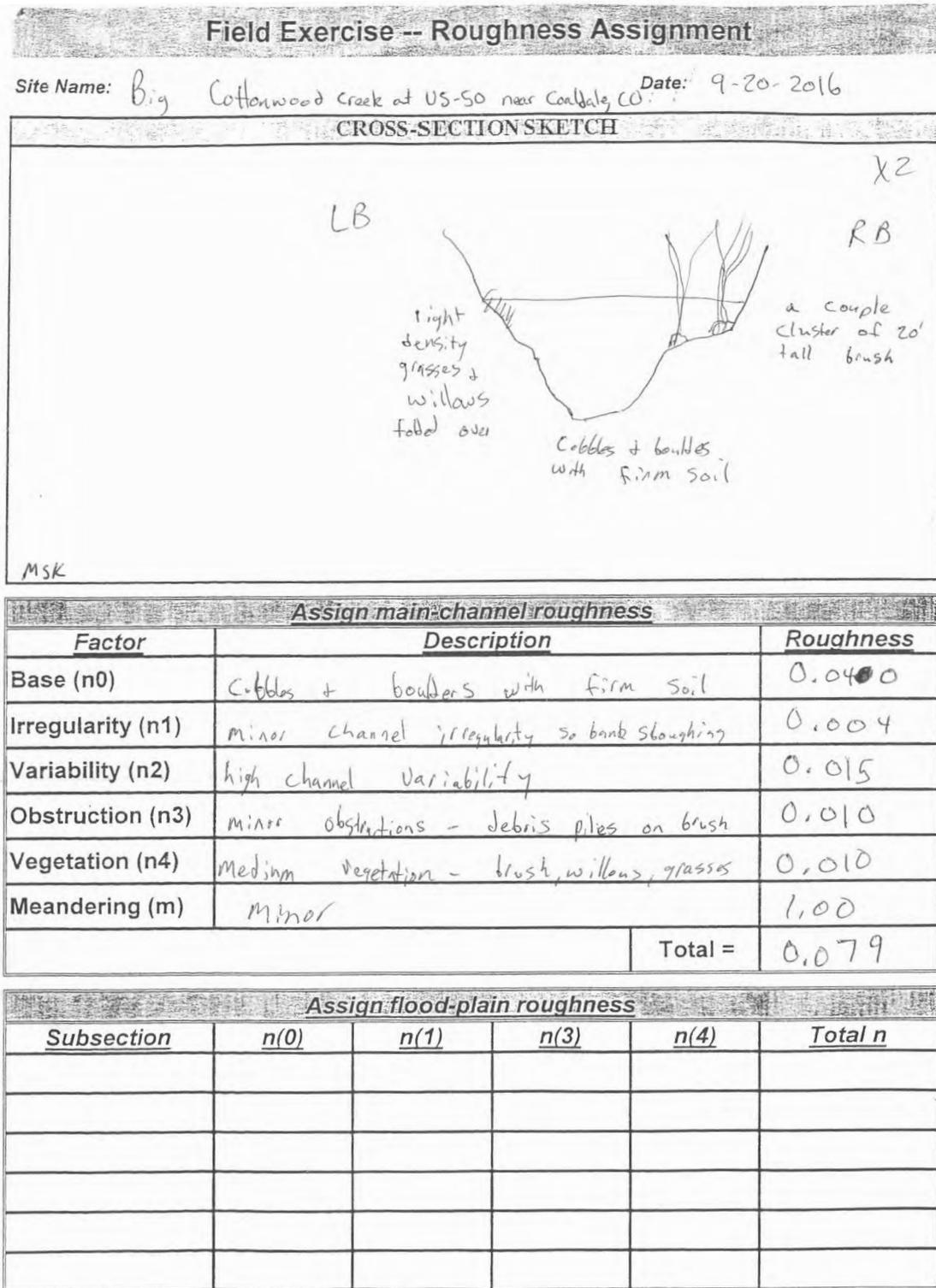
**Figure 4-2.** The Manning roughness coefficient (n) assignment for cross section 2 on Big Cottonwood Creek at U.S. Highway 50 near Coaldale, Colorado.
