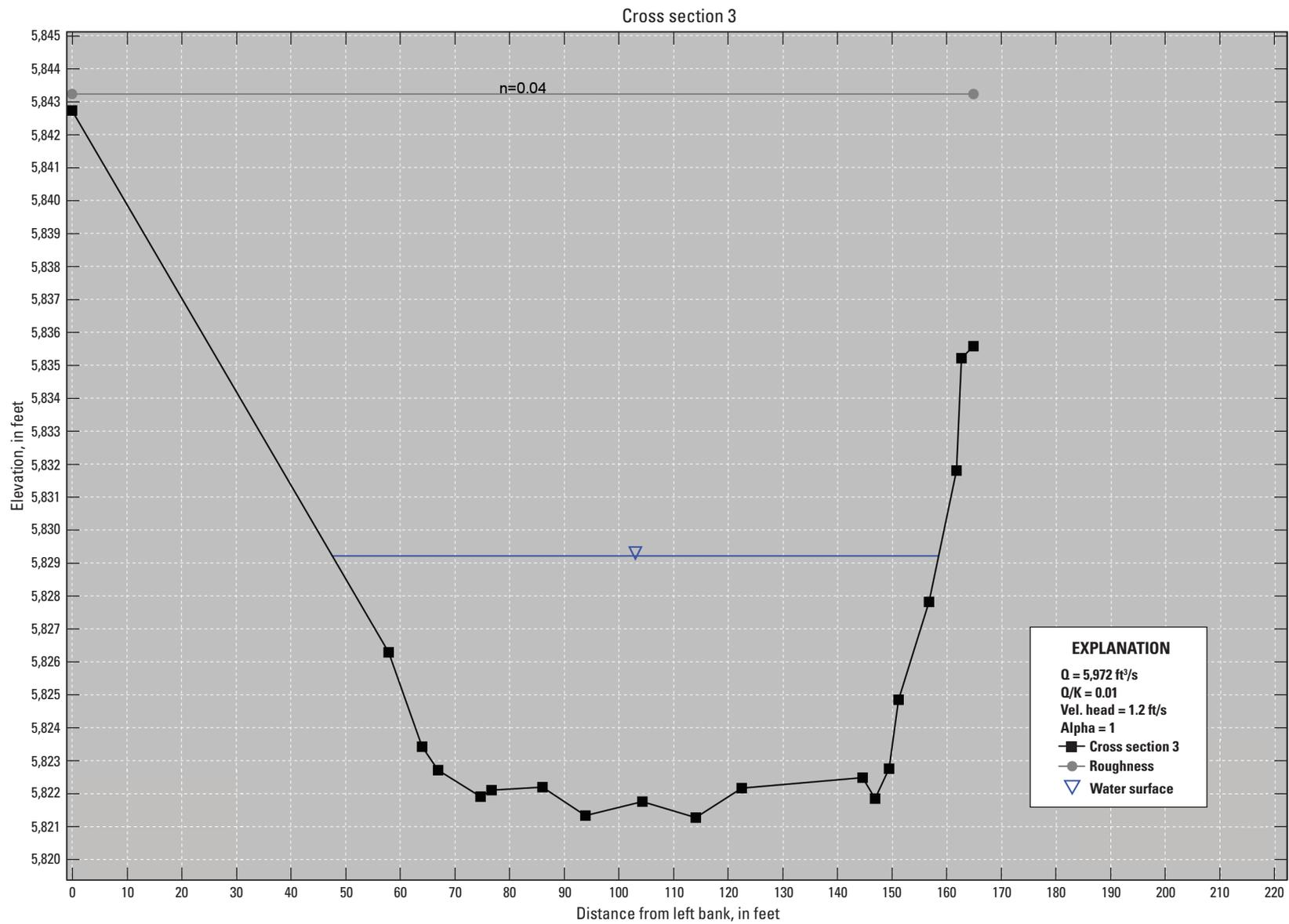
**Figure 10-3.** Cross section 3 with the Manning roughness coefficient (n) assignment for Fountain Creek below U.S. Highway 24 in Colorado Springs, Colorado; generated from the Slope-Area Computation Graphical User Interface. [X3, cross section 3; Q, discharge; ft<sup>3</sup>/s, cubic foot per second; K, conveyance; Vel., velocity; ft/s, foot per second]
