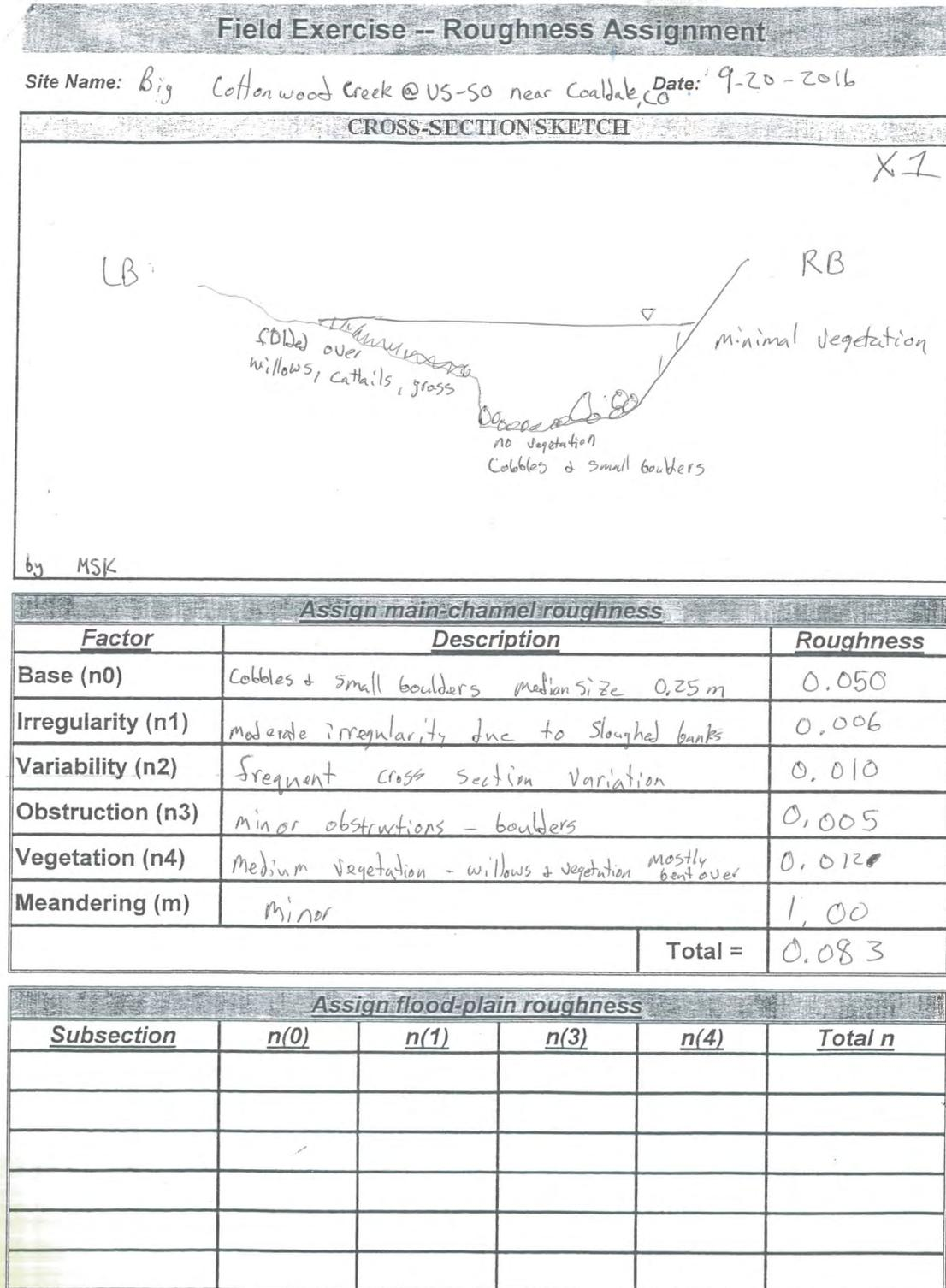
**Figure 4-1.** The Manning roughness coefficient (n) assignment for cross section 1 on Big Cottonwood Creek at U.S. Highway 50 near Coaldale, Colorado.
