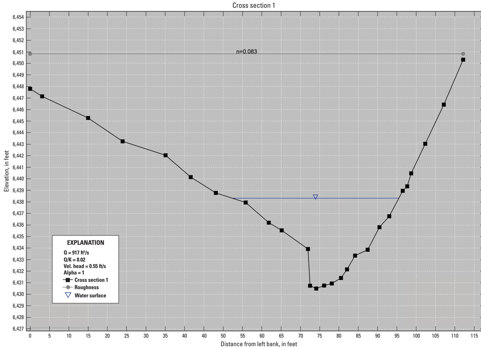
**Figure 5-1.** Cross section 1 with the Manning roughness coefficient (n) assignment for Big Cottonwood Creek at U.S. Highway 50 near Coaldale, Colorado; generated from the Slope-Area Computation Graphical User Interface. [X1, cross section 1; Q, discharge; ft<sup>3</sup>/s, cubic foot per second; K, conveyance; Vel., velocity; ft/s, foot per second]
