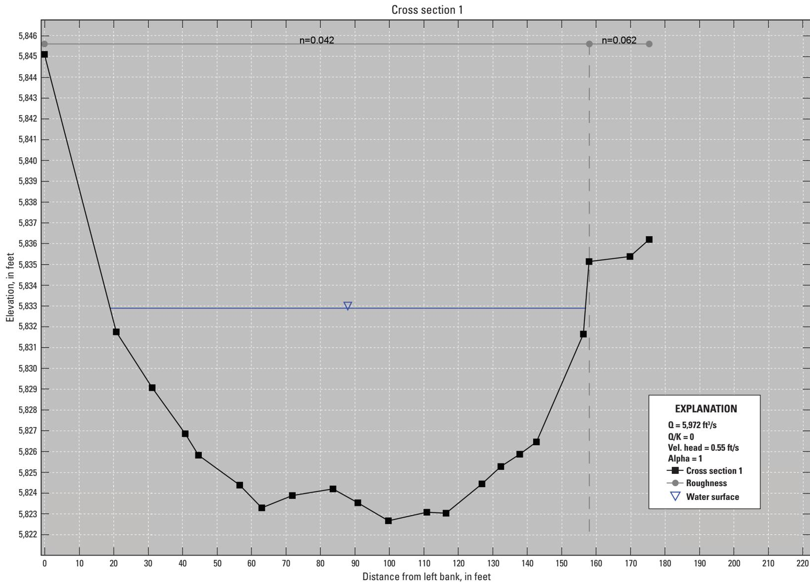
**Figure 10-1.** Cross section 1 with the Manning roughness coefficient (n) assignment for Fountain Creek below U.S. Highway 24 in Colorado Springs, Colorado; generated from the Slope-Area Computation Graphical User Interface. [X1, cross section 1; Q, discharge; ft<sup>3</sup>/s, cubic foot per second; K, conveyance; Vel., velocity; ft/s, foot per second]
