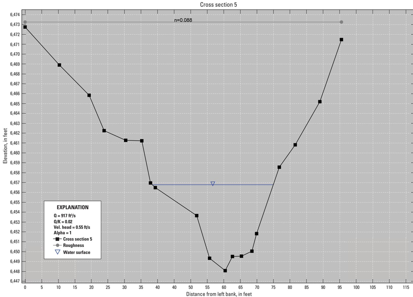
**Figure 5-5.** Cross section 5 with the Manning roughness coefficient ( $n$ ) assignment for Big Cottonwood Creek at U.S. Highway 50 near Coaldale, Colorado; generated from the Slope-Area Computation Graphical User Interface. [X5, cross section 5;  $Q$ , discharge;  $\text{ft}^3/\text{s}$ , cubic foot per second;  $K$ , conveyance; Vel., velocity;  $\text{ft/s}$ , foot per second]
