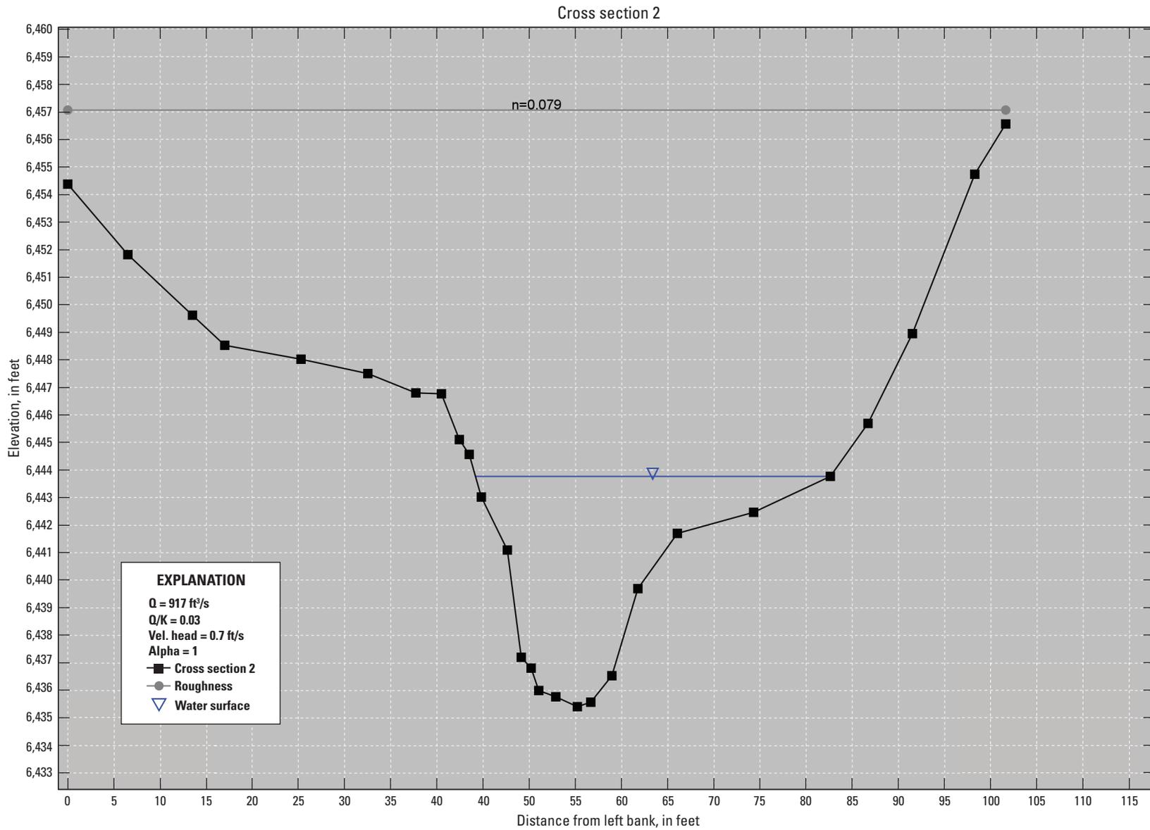
**Figure 5-2.** Cross section 2 with the Manning roughness coefficient ( $n$ ) assignment for Big Cottonwood Creek at U.S. Highway 50 near Coaldale, Colorado; generated from the Slope-Area Computation Graphical User Interface. [X2, cross section 2;  $Q$ , discharge;  $\text{ft}^3/\text{s}$ , cubic foot per second;  $K$ , conveyance; Vel., velocity;  $\text{ft/s}$ , foot per second]
