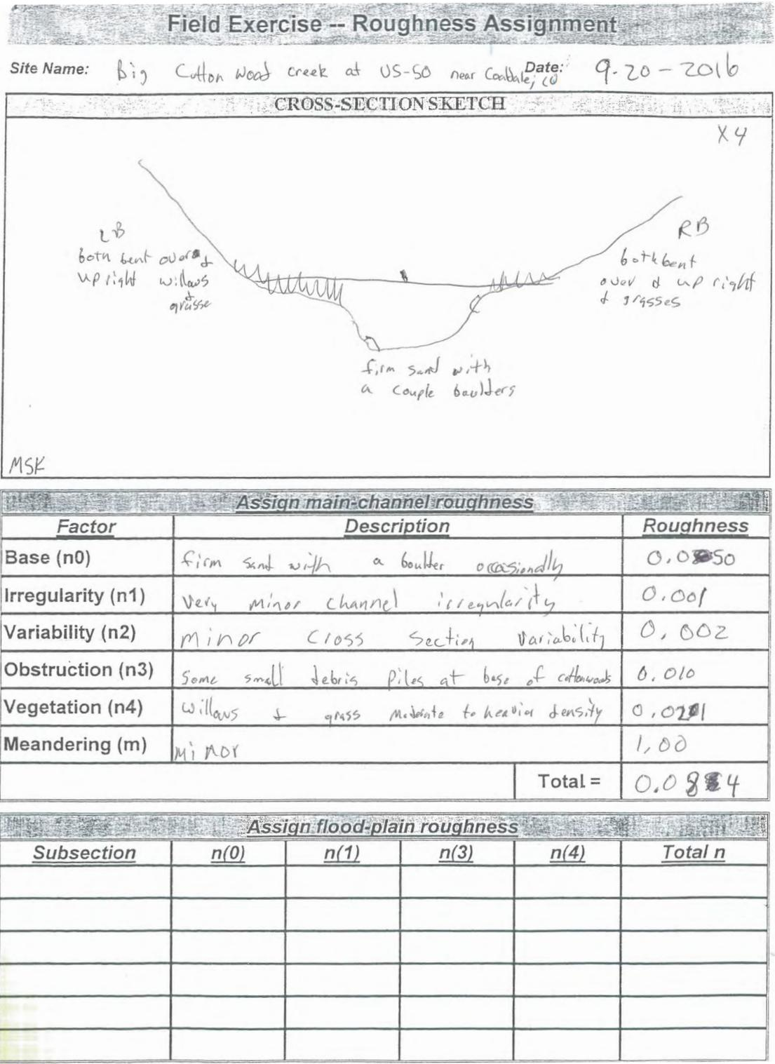
Figure 4-4. The Manning roughness coefficient (n) assignment for cross section 4 on Big Cottonwood Creek at U.S. Highway 50 near Coaldale, Colorado.
