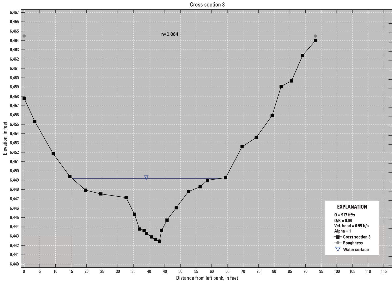
**Figure 5-3.** Cross section 3 with the Manning roughness coefficient (n) assignment for Big Cottonwood Creek at U.S. Highway 50 near Coaldale, Colorado; generated from the Slope-Area Computation Graphical User Interface. [X3, cross section 3; Q, discharge; ft³/s, cubic foot per second; K, conveyance; Vel., velocity; ft/s, foot per second]
