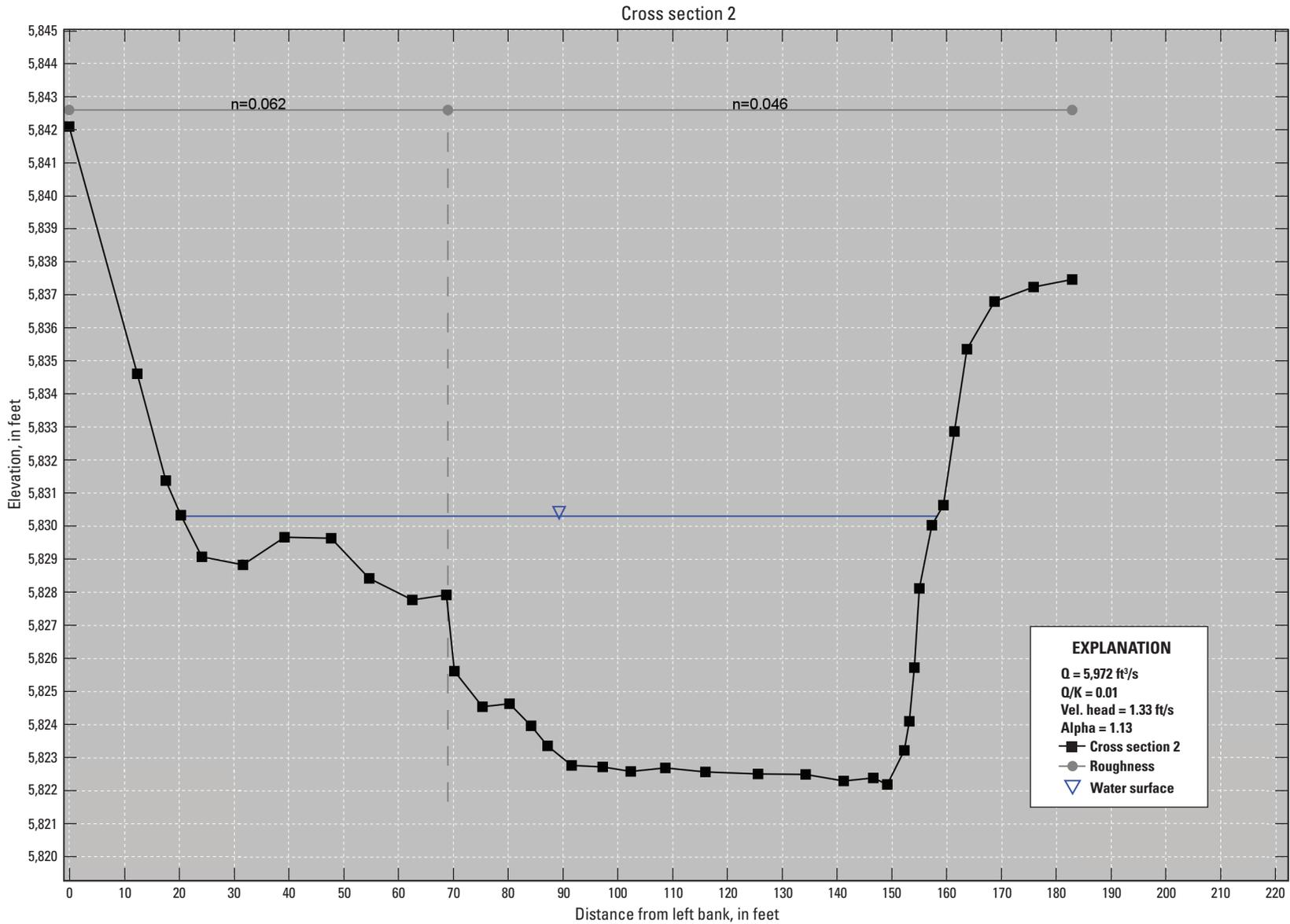
**Figure 10-2.** Cross section 2 with the Manning roughness coefficient (n) assignment for Fountain Creek below U.S. Highway 24 in Colorado Springs, Colorado; generated from the Slope-Area Computation Graphical User Interface. [X2, cross section 2; Q, discharge; ft<sup>3</sup>/s, cubic foot per second; K, conveyance; Vel., velocity; ft/s, foot per second]
