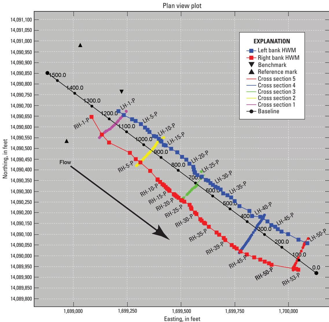
**Figure 10.** Plan view of the site showing the left and right bank high-water marks (HWMs) and cross sections for Fountain Creek below U.S. Highway 24 in Colorado Springs, Colorado; generated from the Slope-Area Computation Graphical User Interface. For readability, not all data points are labeled.
