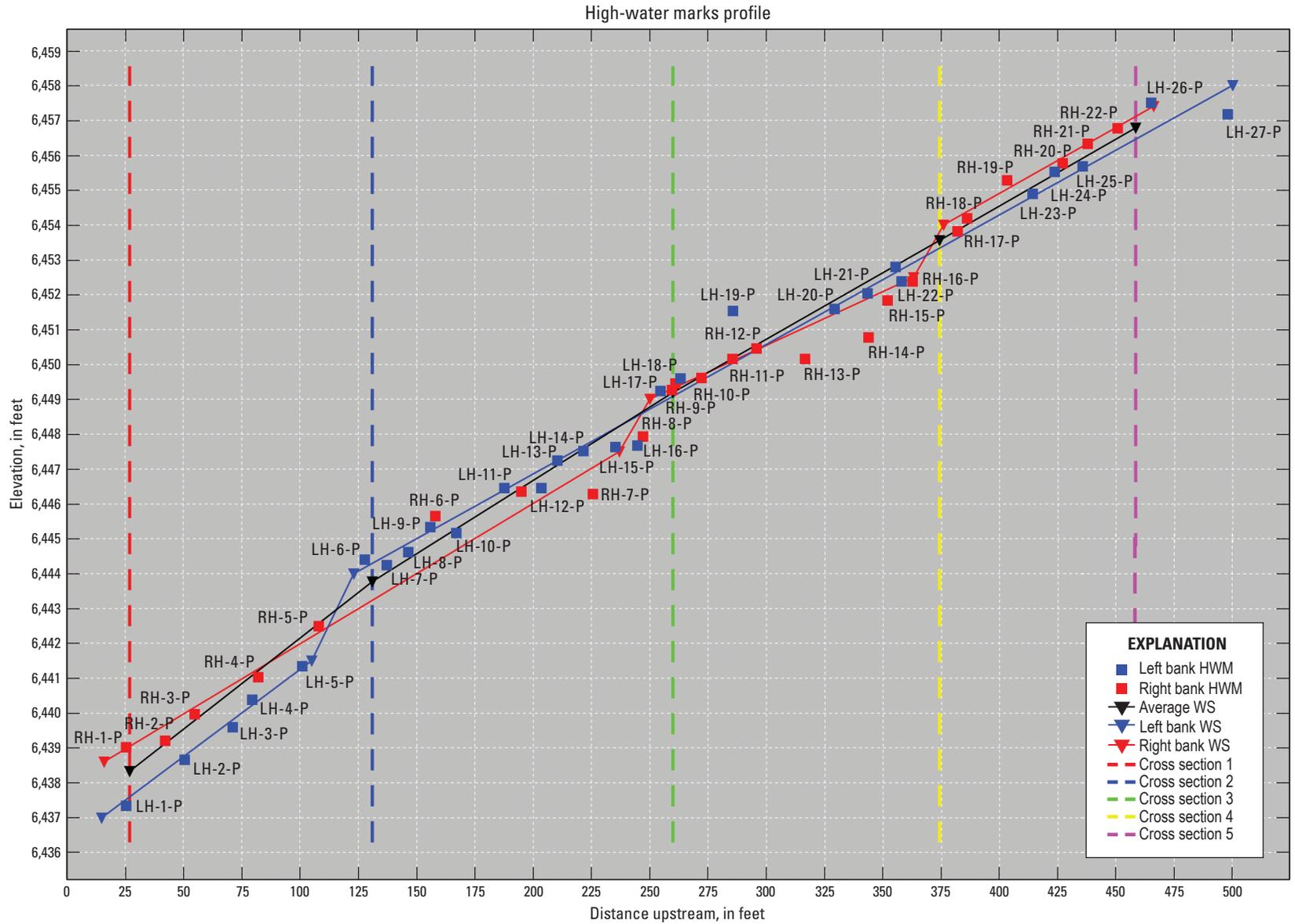
**Figure 4.** Profile view of the left and right bank high-water marks (HWMs) and cross sections for Big Cottonwood Creek at U.S. Highway 50 near Coaldale, Colorado; generated using the Slope-Area Computation Graphical User Interface. For readability, not all data points are labeled. [WS, water surface]
