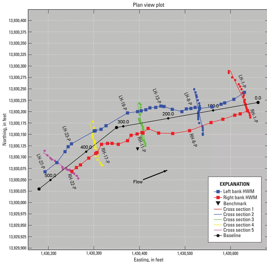
**Figure 3.** Plan view of the site showing the left and right bank high-water marks (HWMs) and cross sections for Big Cottonwood Creek at U.S. Highway 50 near Coaldale, Colorado; generated using the Slope-Area Computation Graphical User Interface. For readability, not all data points are labeled.
