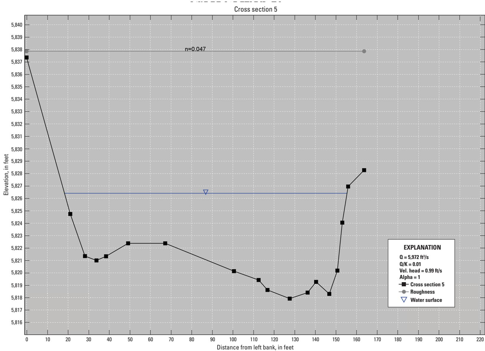
**Figure 10-5.** Cross section 5 with the Manning roughness coefficient (n) assignment for Fountain Creek below U.S. Highway 24 in Colorado Springs, Colorado; generated from the Slope-Area Computation Graphical User Interface. [X5, cross section 5; Q, discharge; ft<sup>3</sup>/s, cubic foot per second; K, conveyance; Vel., velocity; ft/s, foot per second]
