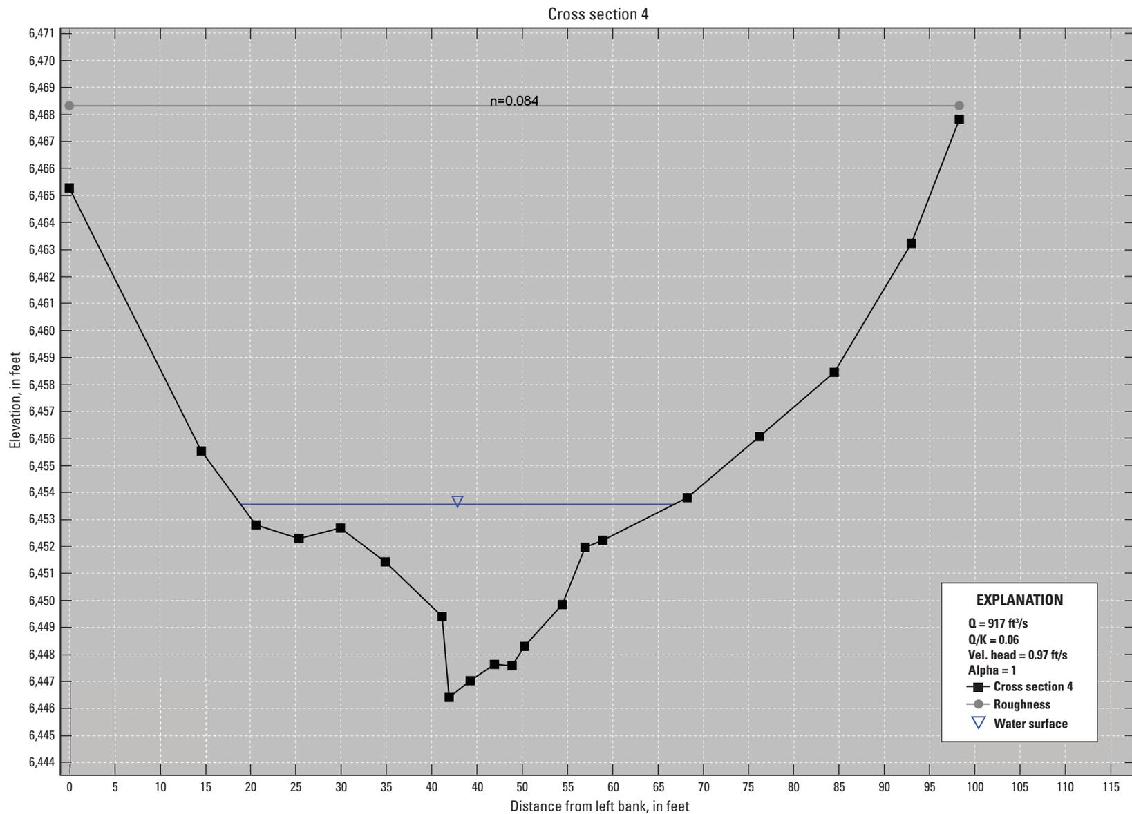
**Figure 5-4.** Cross section 4 with the Manning roughness coefficient (n) assignment for Big Cottonwood Creek at U.S. Highway 50 near Coaldale, Colorado; generated from the Slope-Area Computation Graphical User Interface. [X4, cross section 4; Q, discharge; ft<sup>3</sup>/s, cubic foot per second; K, conveyance; Vel., velocity; ft/s, foot per second]
