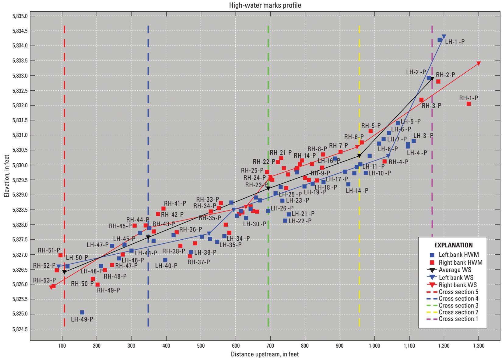
**Figure 11.** Profile view of the left and right bank high-water marks (HWMs) and cross sections for Fountain Creek below U.S. Highway 24 in Colorado Springs, Colorado; generated using the Slope-Area Computation Graphical User Interface. For readability, not all data points are labeled. [WS, water surface]
