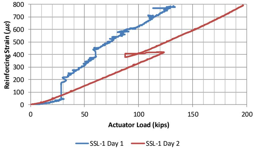
Figure 80 - Comparison of Days 1 and 2 Actuator Load and Reforcing Strain
