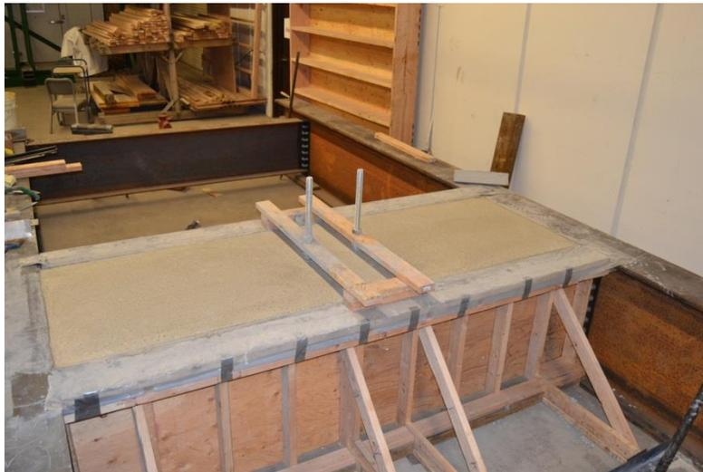
**Figure 48 - Self-Reacting Load Frame - Finished Concrete Support Pier**
