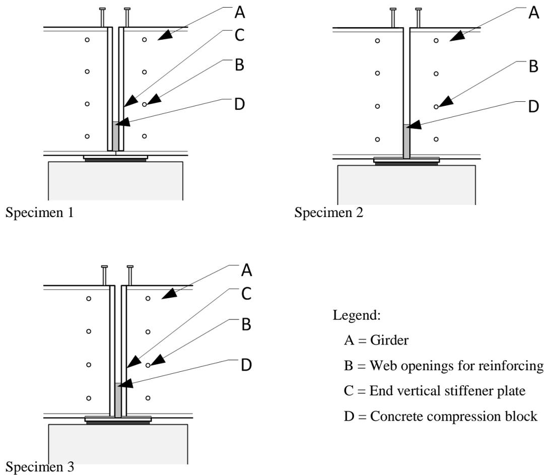
**Figure 2 - Girder Connection Specimens Tested at University of Nebraska-Lincoln (Farimani M. , 2006)**
