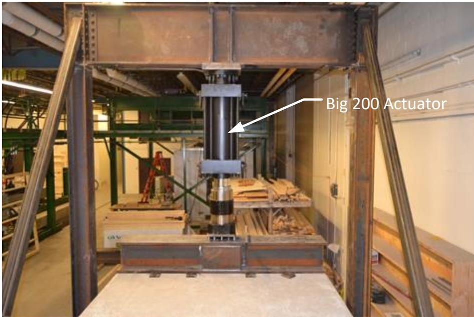
**Figure 54 - 220 kip Actuator and Load Application Beam**
