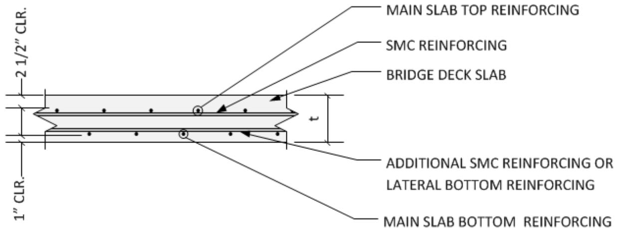
**Figure 101 Slab Reinforcing Placement**
