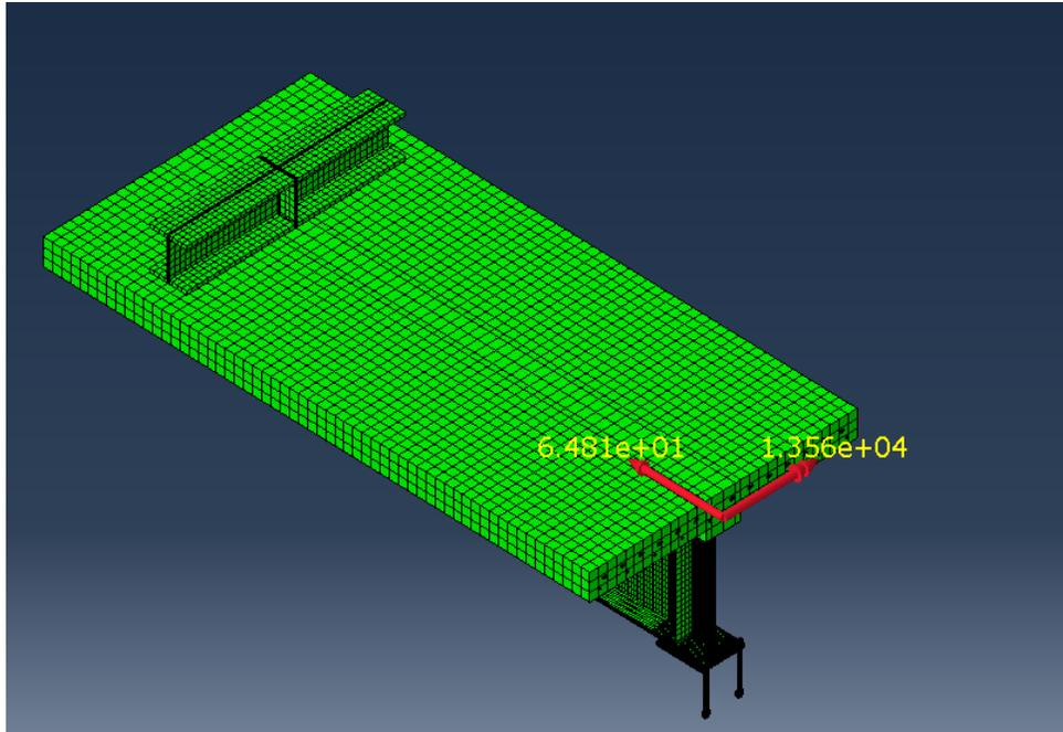
**Figure 38 - Centerline Negative Moment at SMC Connection**
