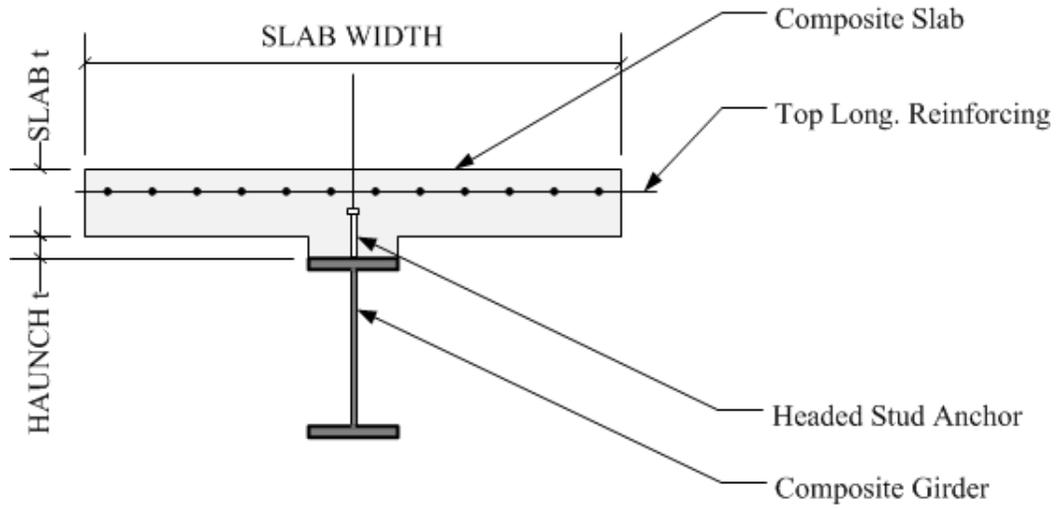
Figure 32 - Sensitivity Analysis Composite Girder - Section
