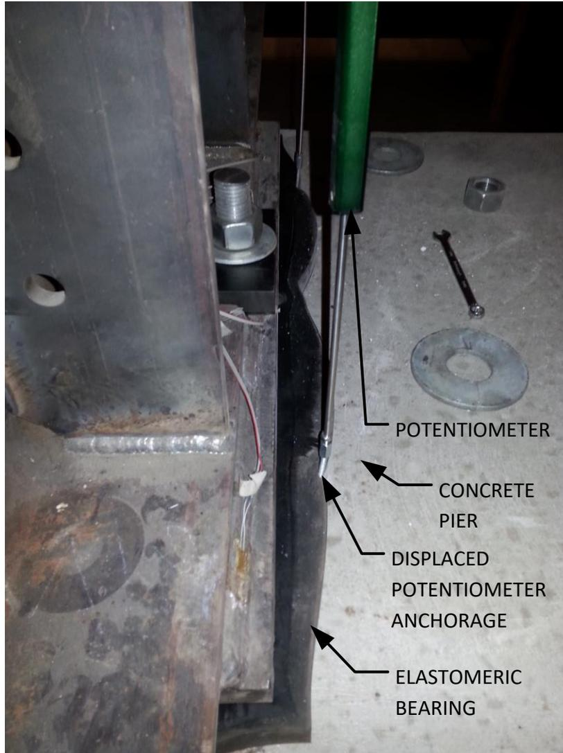
**Figure 92 - Distorted Potentiometer Anchorages - Day 2**
