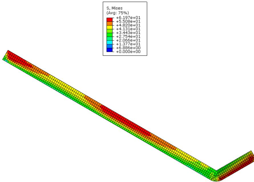
**Figure 45 - von Mises Stress in Weld after 75% of Concentrated Load Application**
