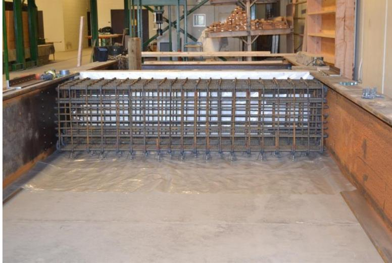
**Figure 47 - Self-Reacting Load Frame - Concrete Support Pier Reinforcing**
