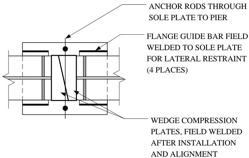
**Figure 108 - SMC Girder Support Detail 3 - Plan View**
