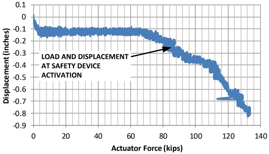
**Figure 75 - Displacement at North Girder vs. Actuator Force –Day 1**
