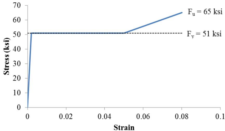
**Figure 22 - Stress-strain diagram for stud shear connectors**
