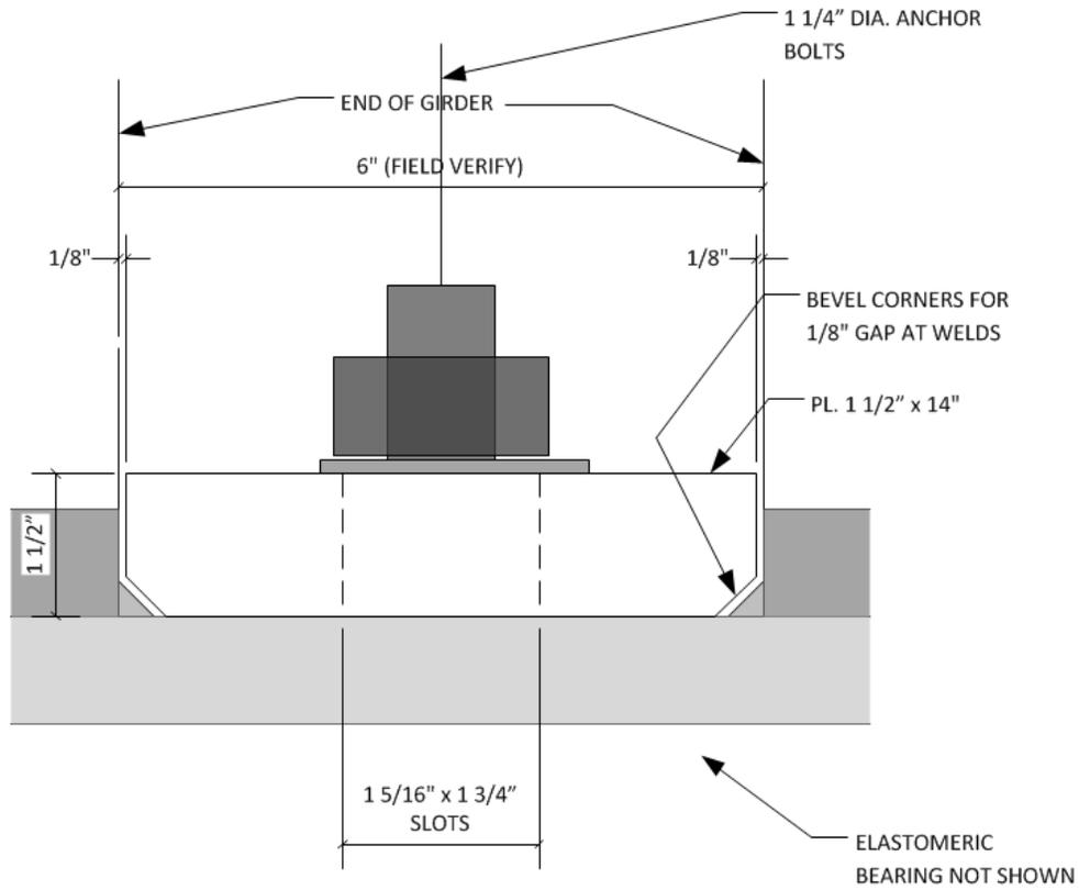
**Figure 49 - Safety Device Details**
