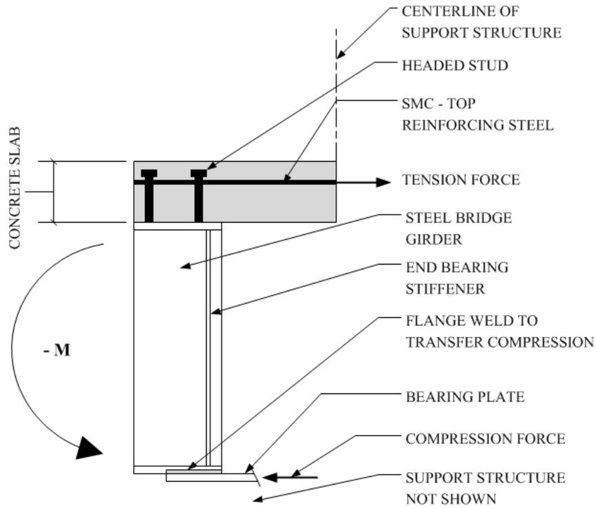
**Figure 14 – Steel SMC Connection Elements without Concrete Diaphragm**
