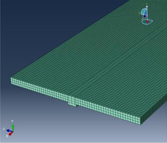
**Figure 29 - Meshed Slab and Haunch**
