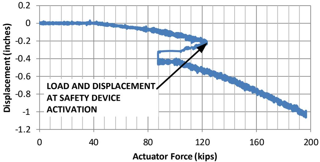
Figure 90 - Displacement at North Girder vs. Actuator Force - Day 2
