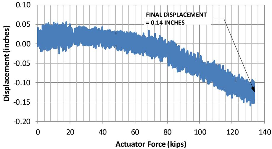
Figure 77 - Displacement of North Elastomeric Bearing – Day 1
