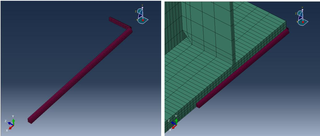
**Figure 28 - Weld (left), Weld and Girder (right)**
