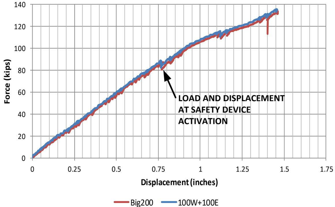
**Figure 70 - Actuator Force vs. Displacement – Day 1 Test**
