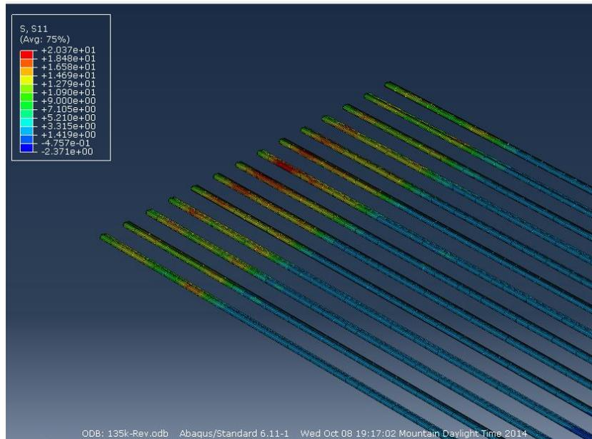
**Figure 97 - Axial Stress in SMC Top Reinforcing Steel**
