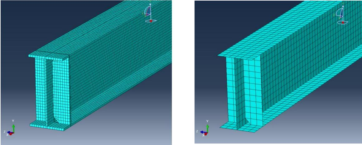
**Figure 25 - Meshed Girders - Solid Brick Elements (left) and Shell Elements (right)**
