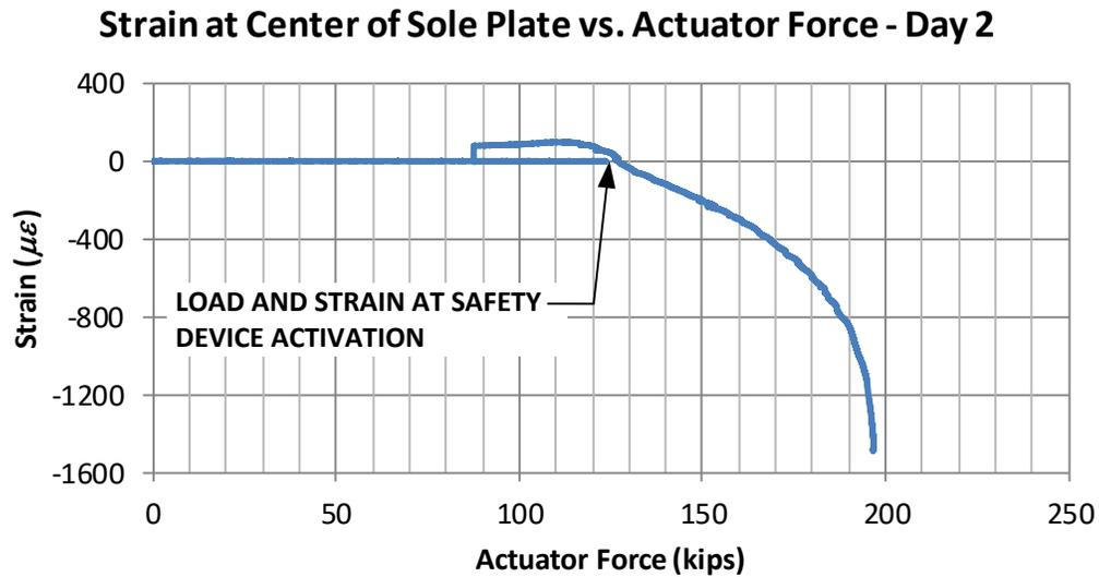
**Figure 88 - Strains at Center of Safety Device - Day 2**
