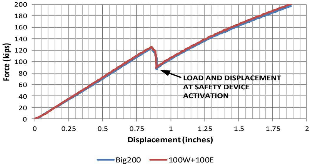
**Figure 79 - Actuator Force vs. Displacement - Day 2 Test**
