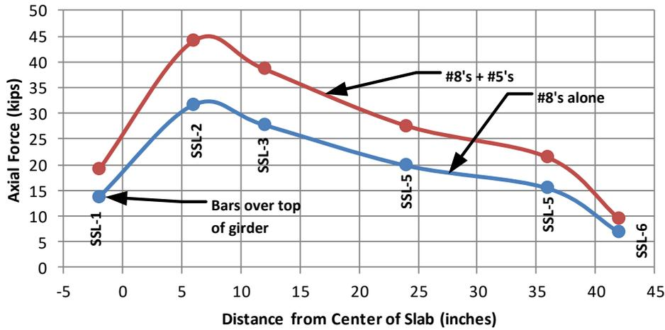
Figure 83 - Shear Lag in Top SMC Bars - Day 2 Test - Safety Device Activation
