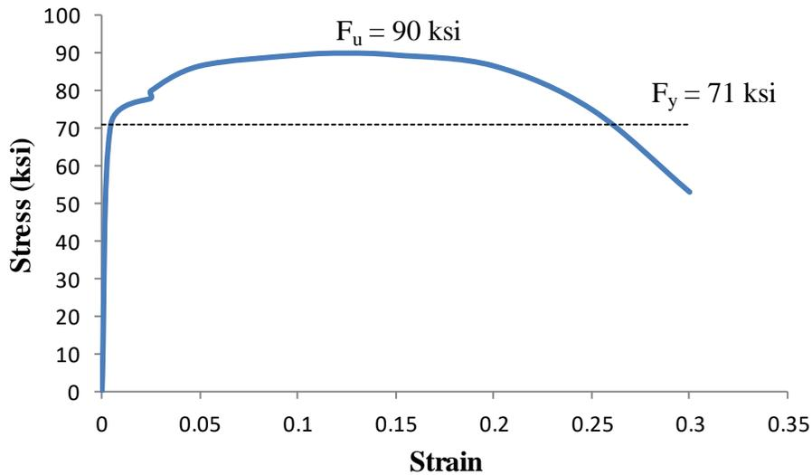
**Figure 21 - Stress-Strain Diagram for Weld Metal (Ricles, 2000)**
