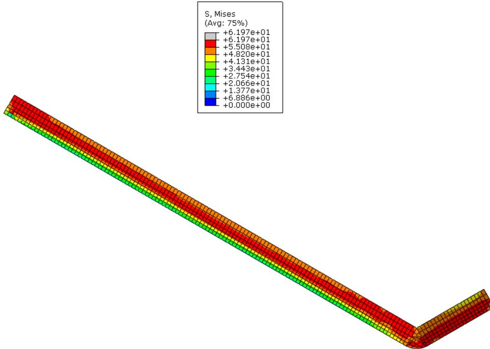
**Figure 46 - von Mises Stress in Weld after 100% of Concentrated Load Application**
