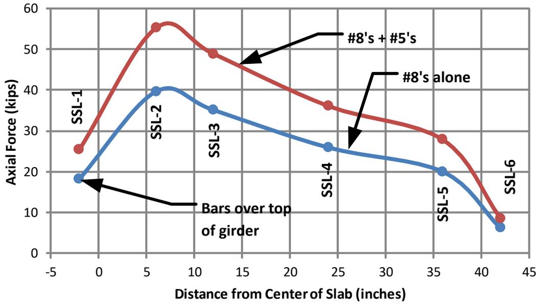
**Figure 71 - Shear Lag in Top SMC Bars - Day 1 Test**
