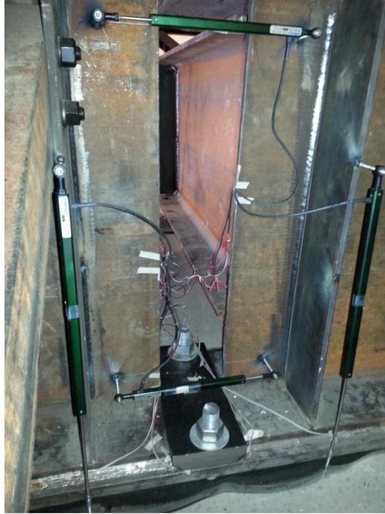
Figure 59 - Pots 3, 4, 5 and 6 in Position During Testing
