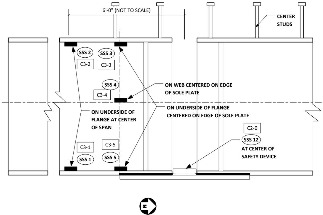
Figure 60 - Instrumentation at the Girder Ends -2
