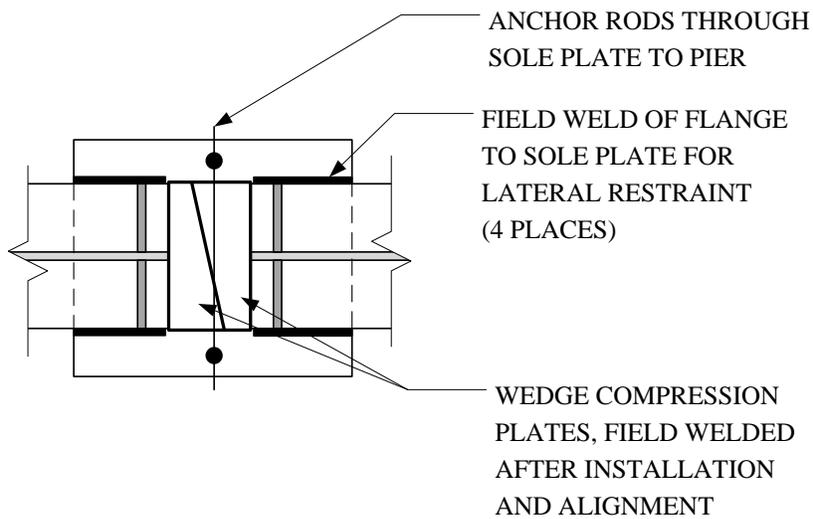
**Figure 106 - SMC Girder Support Detail 2 - Plan View**
