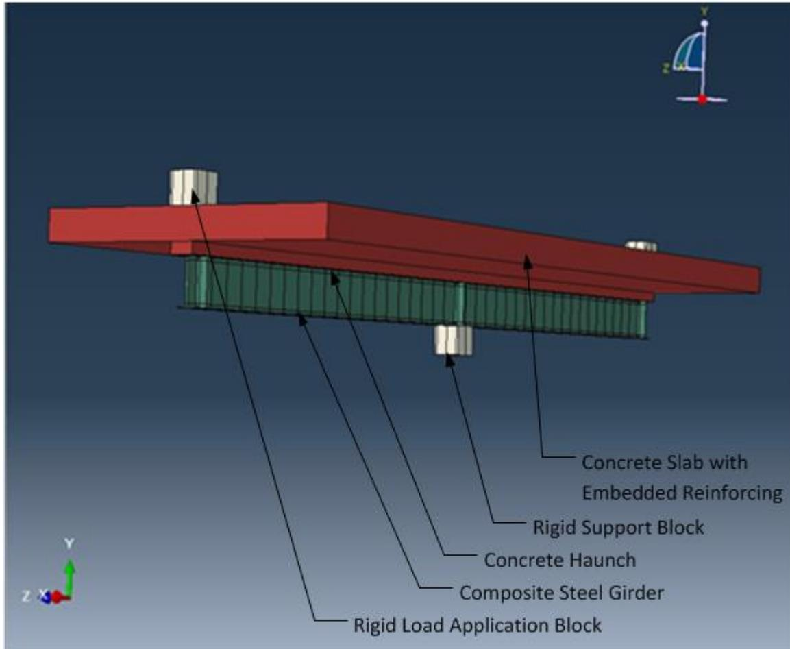
Figure 33 - Sensitivity Girder - ABAQUS Model
