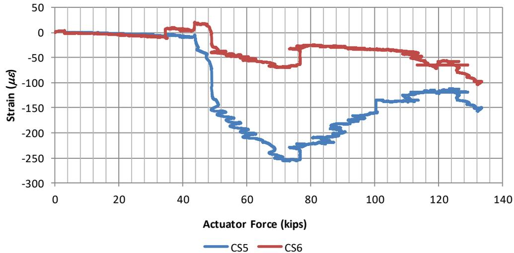
**Figure 73 - Concrete Bottom Surface Strains**
