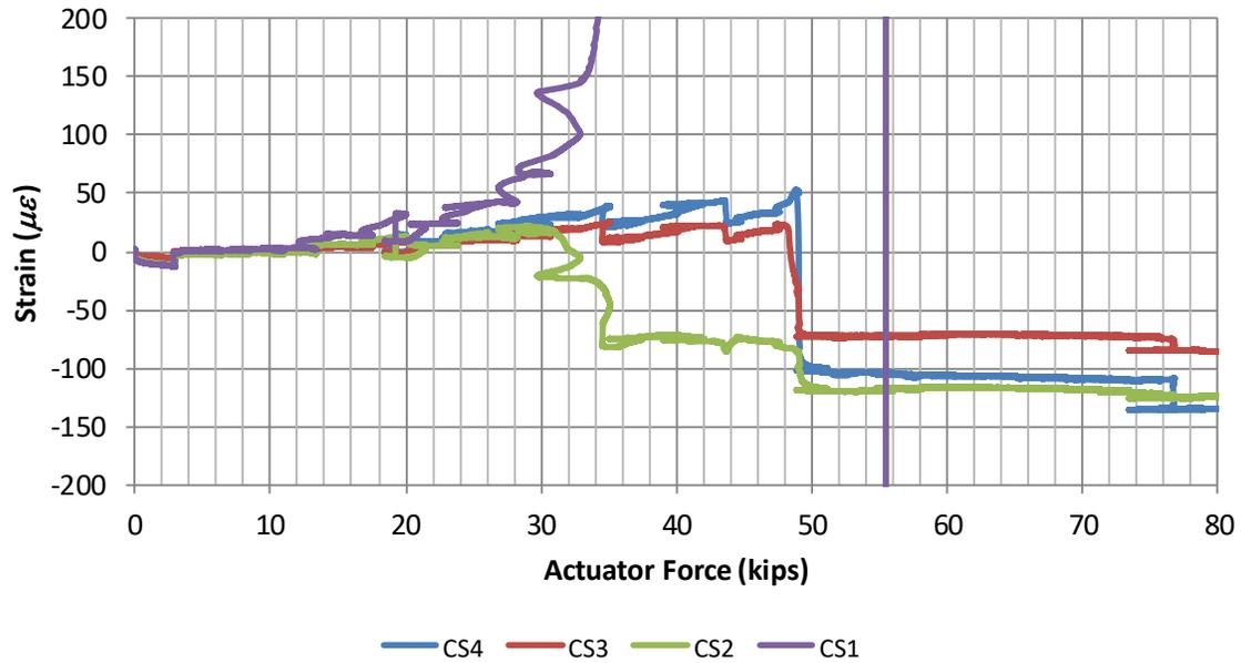
**Figure 72 - Concrete Top Surface Strains**
