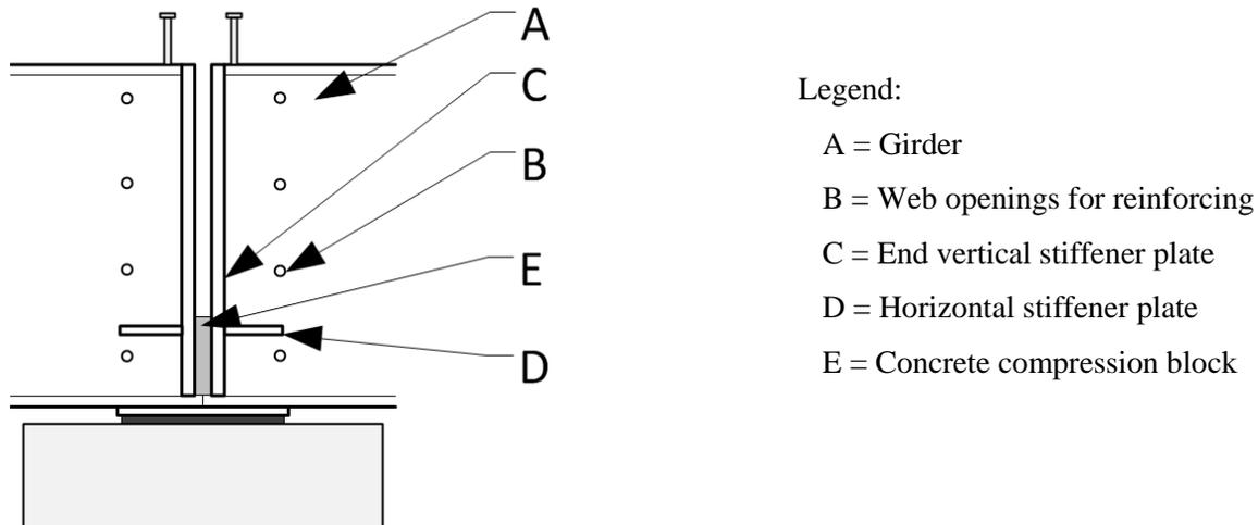
**Figure 1 - Girder connection specimen modeled at University of Nebraska - Lincoln (Lampe N. J., 2001)**
