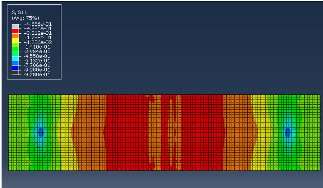
**Figure 43 - Concrete Surface Axial Stress after 100% of Concentrated Load Application**
