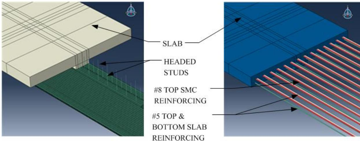
**Figure 37 - Slab, Studs and Reinforcing Constraints**
