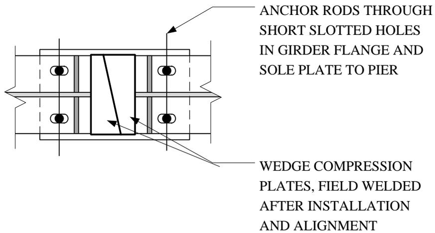
**Figure 104 - SMC Girder Support Detail 1 - Plan View**
