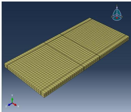
**Figure 26 - Meshed Sole Plate**
