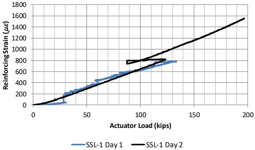
Figure 82 - Comparison of Days 1 and 2 Actuator Load and Reforcing Strain - Scheme 2
