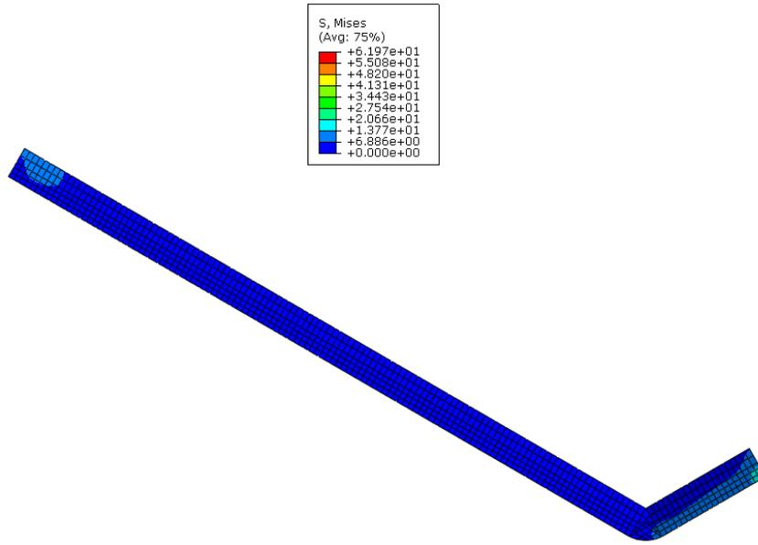
**Figure 44 - von Mises Stress in Weld after Dead Load Application**
