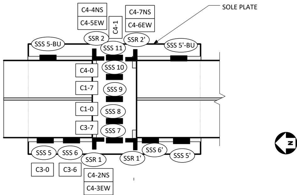
**Figure 61 - Instrumentation Layout at the Sole Plate**
