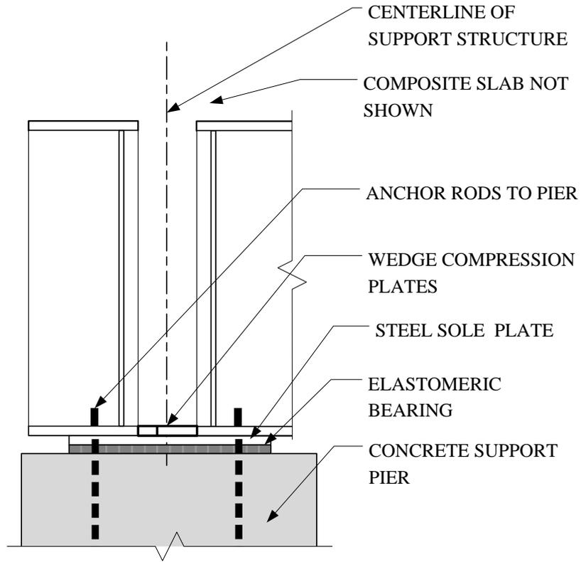
**Figure 103 - SMC Girder Support Detail 1 – Side View**
