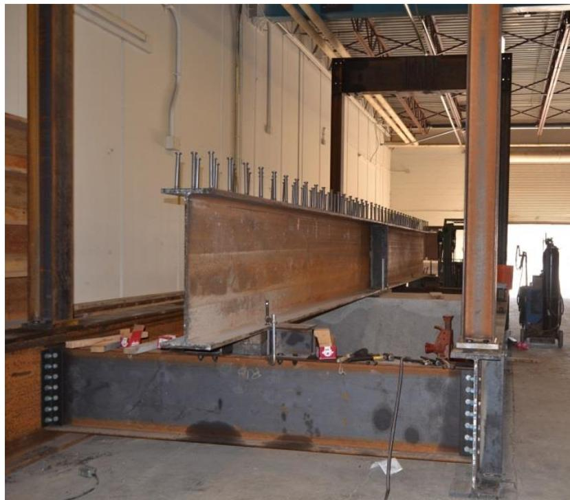
**Figure 50 - Bridge Girders with Studs**
