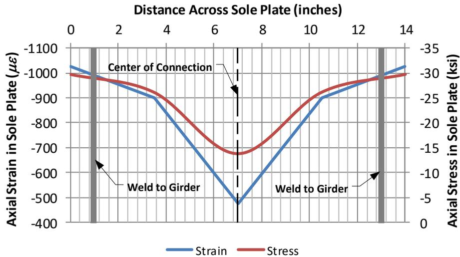
**Figure 74 - Sole Plate Strains and Stresses - Day 1 (Note that strains and stresses are compressive and thus negative)**
