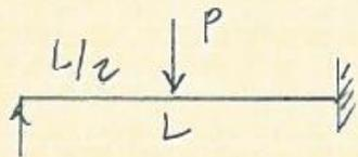
IT'S APPARENT THAT DUE TO INDETERMINACY, THE REQUIRED  $I_x$  FOR THESE CONDITIONS WOULD BE LESS THAN THOSE FOR THE CORRESPONDING SIMPLE BEAM CONDITIONS.
