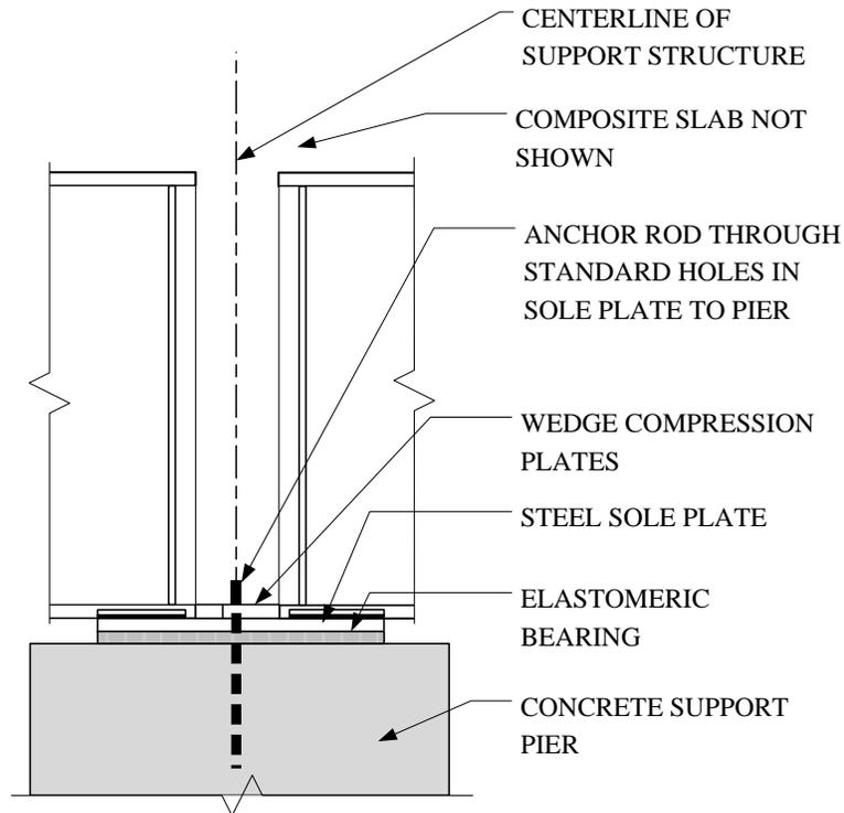
**Figure 107 - SMC Girder Support Detail 3 - Side View**
