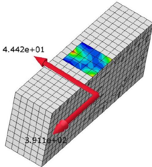
**Figure 39 - Axial Force at Pier**
