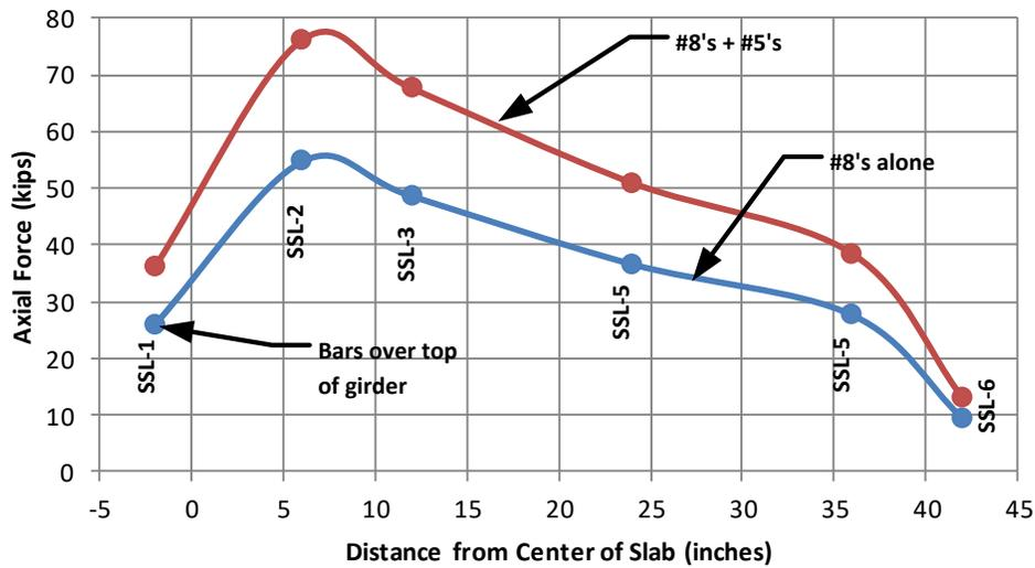
Figure 84 - Shear Lag in Top SMC Bars - Day 2 Test - End of Test
