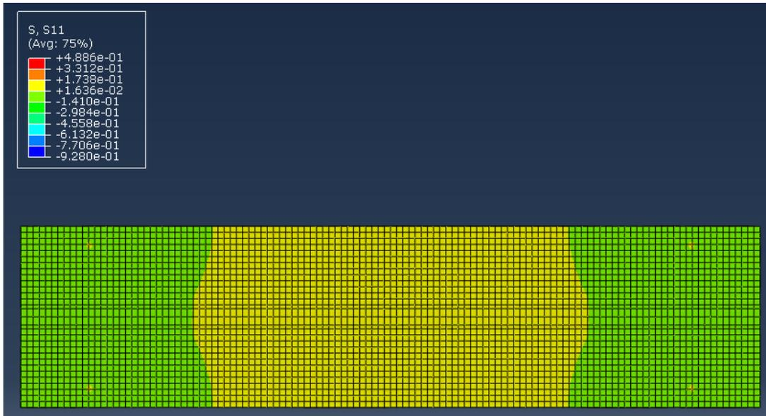
Figure 41 - Concrete Surface Axial Stress after Dead Load Application
