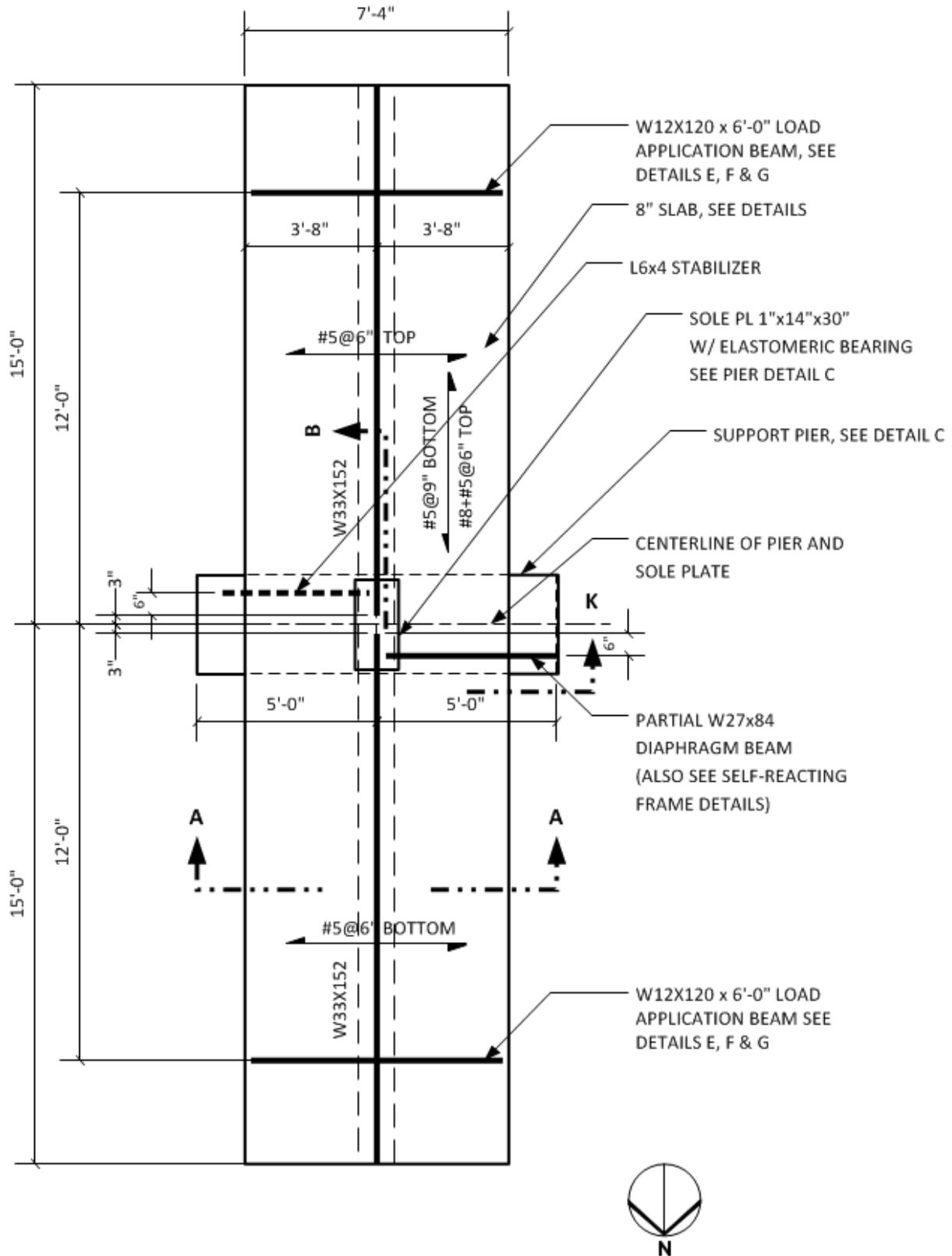
Figure 56 - Plan of Constructed Physical Model
