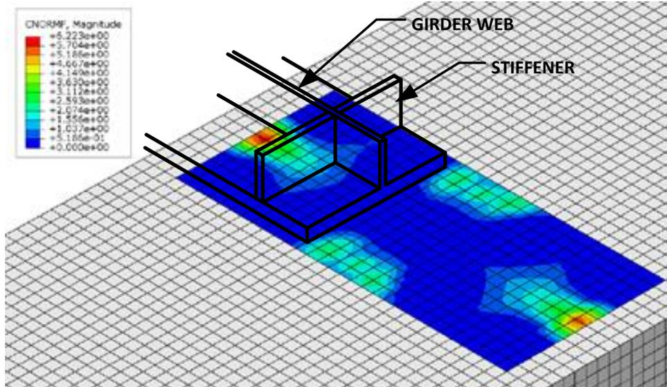
**Figure 96 - Normal Forces on Sole Plate – Abaqus**
