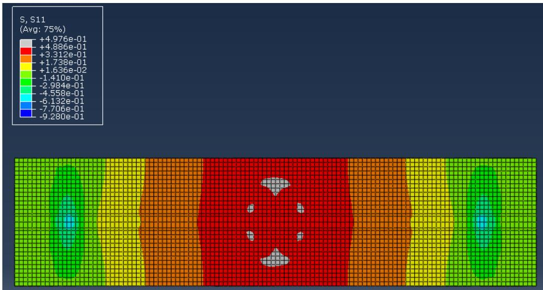
**Figure 42 - Concrete Surface Axial Stress after 75% of Concentrated Load Application**
