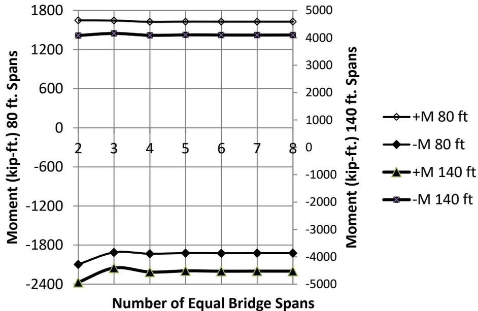
Figure 102 Maximum and Minimum Moments vs. Spans (note: moment scales are different)
