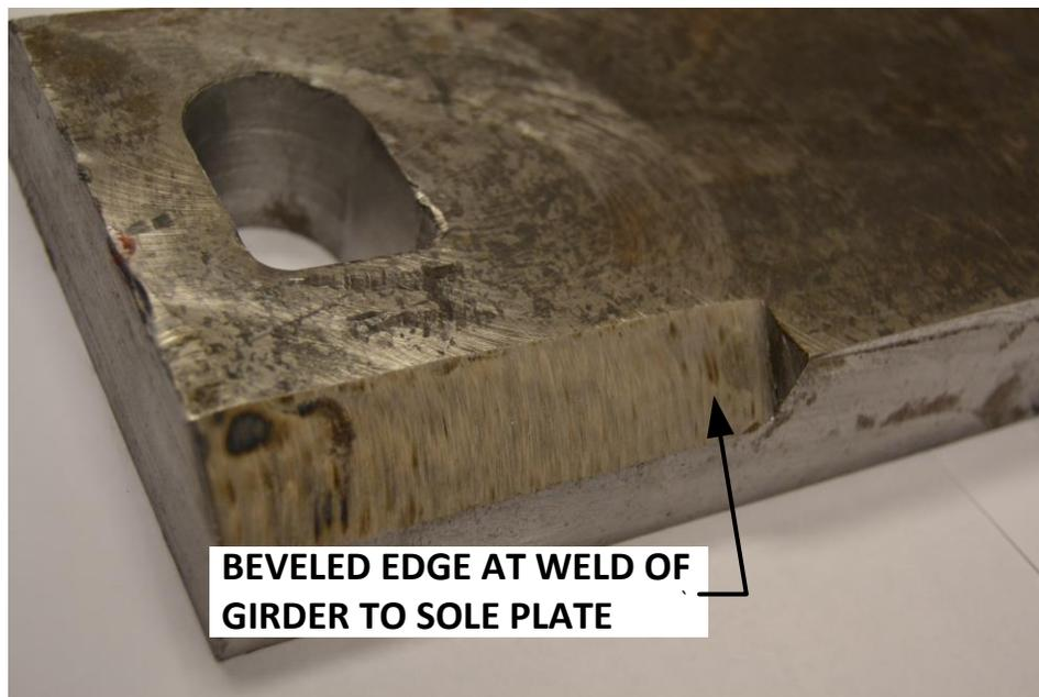
**Figure 89 - Detail of Sole Plate Showing Bevel at Weld**
