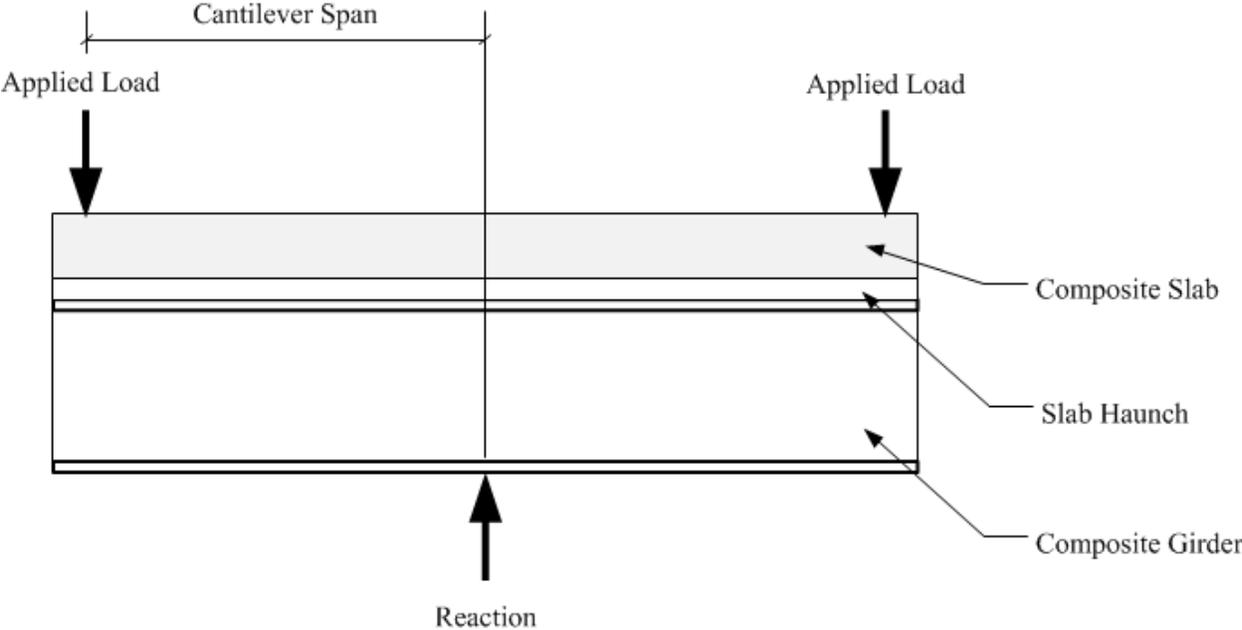
Figure 31 - Sensitivity Analysis Composite Girder - Elevation
