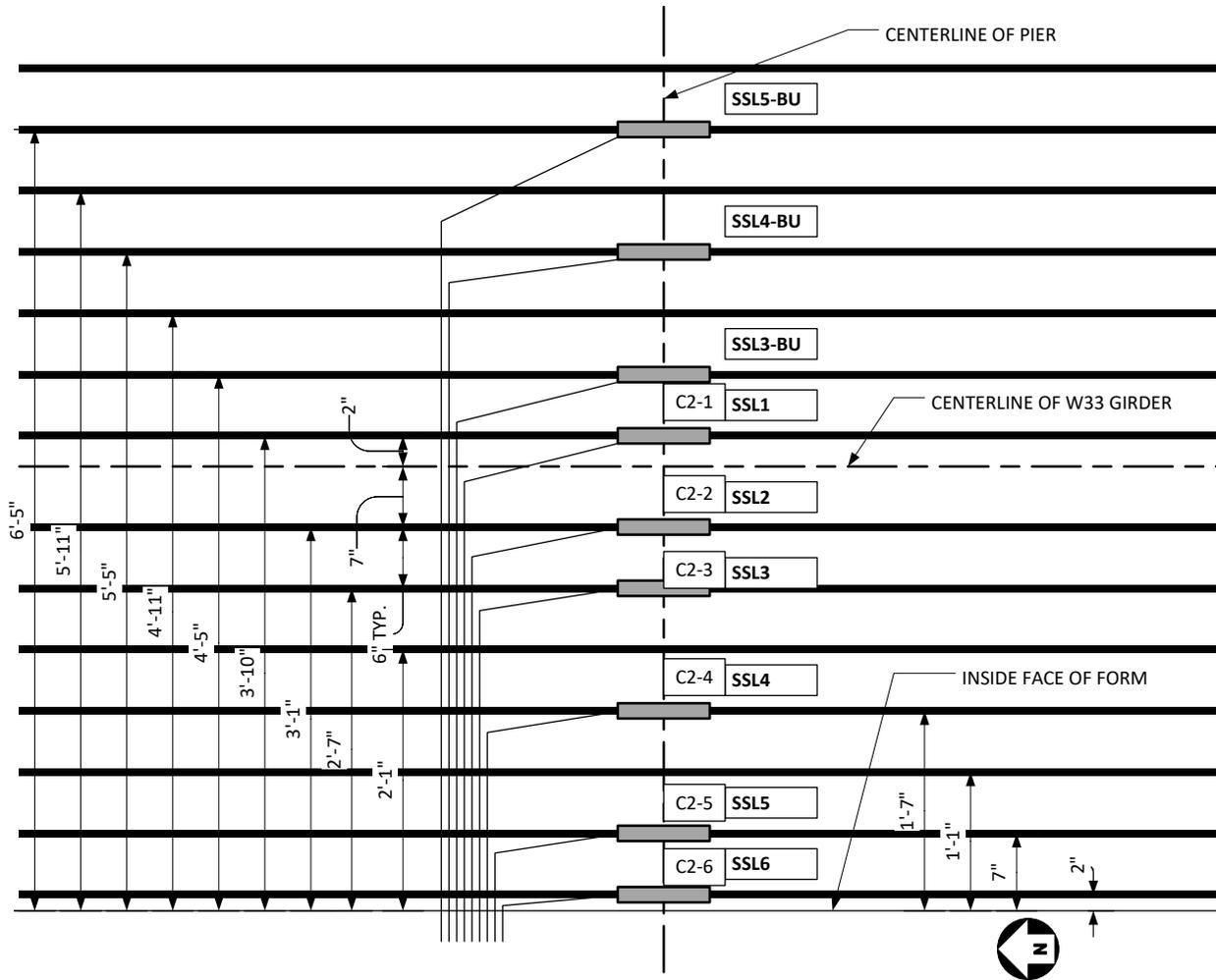
Figure 65 - Instrumentation Layout on the Slab Reinforcing
