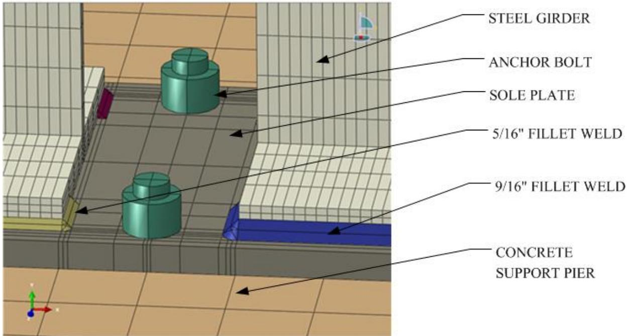
**Figure 36 - Contacts and Constraints at Support Pier**
