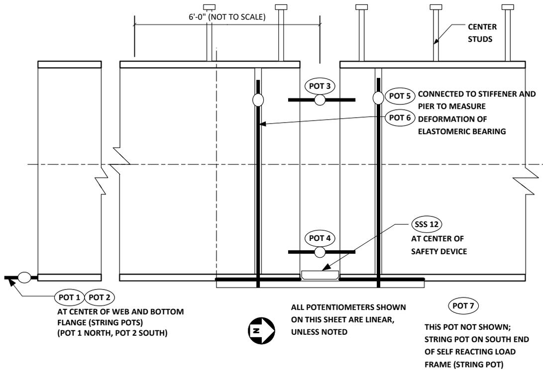
**Figure 58 - Instrumentation Layout at the Girder Ends – 1**
