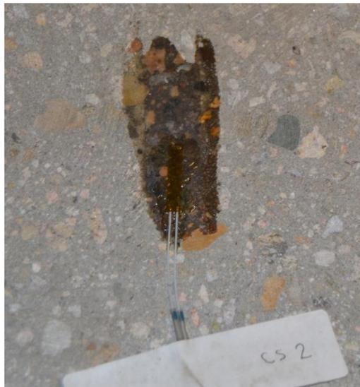
**Figure 63 - Strain Gage Attached to Top of Slab**
