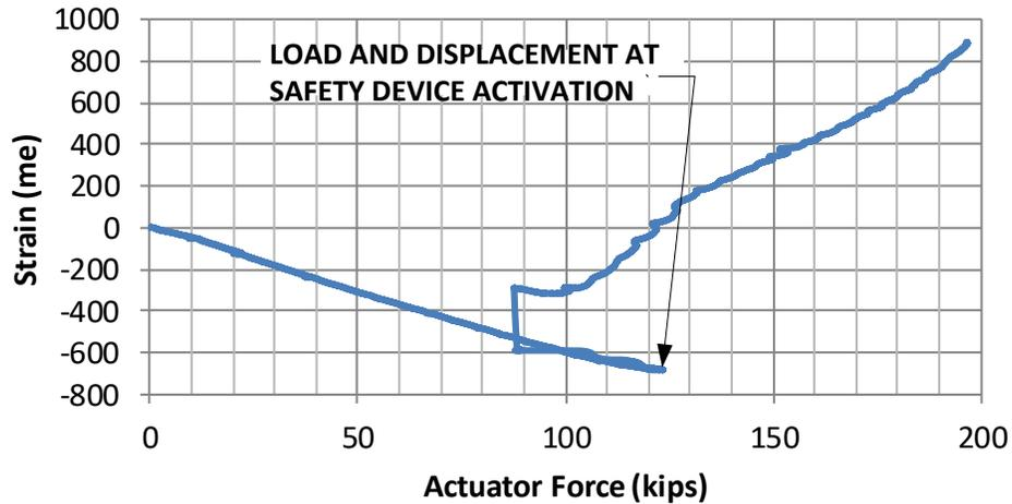
Figure 86 - Strains at Center of Sole Plate
