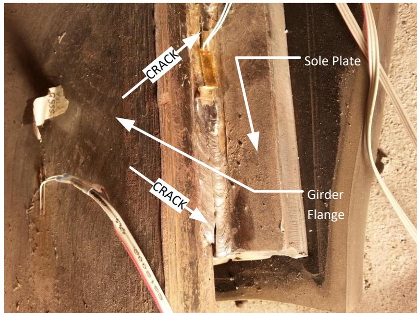
**Figure 69 - Failed Weld on West Side of North Girder**
