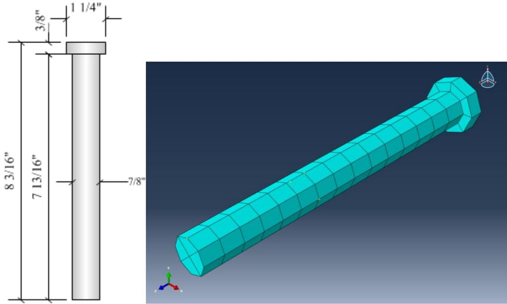
**Figure 27 - Shear Stud Connector Dimensions and as Modeled (brick elements)**
