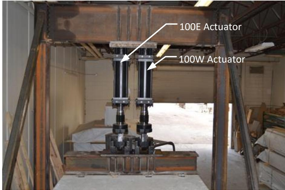
**Figure 55 - (2) 110 kip Actuators and Load Application Beam**
