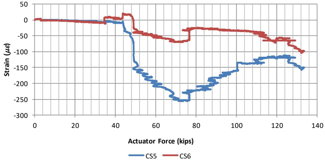
**Figure 73 - Concrete Bottom Surface Strains**
