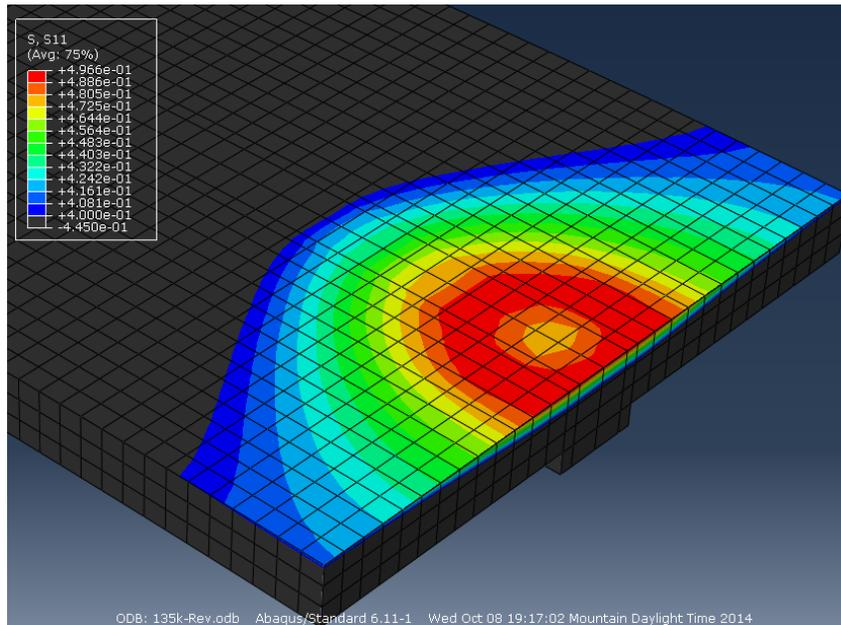
**Figure 99 - Early Shear Lag in Top of Concrete Slab**
