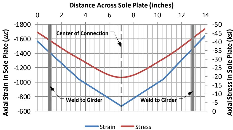
Figure 87 - Sole Plate Strains and Stress at Safety Device Activation - Day 2
