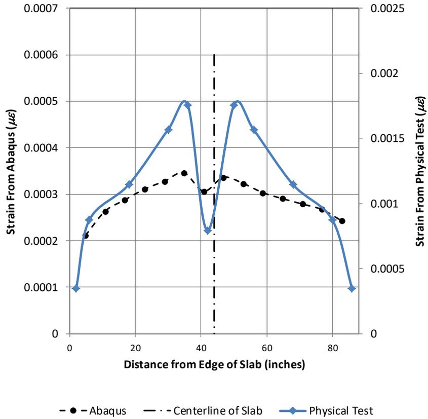
**Figure 98 - Comparison of SMC Reinforcing Strains**
