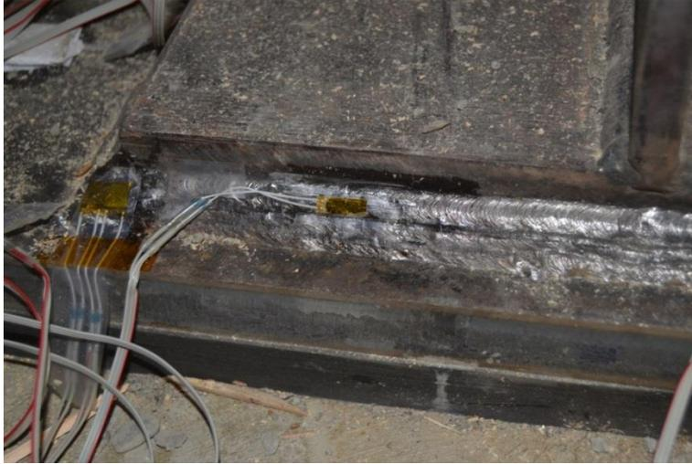
**Figure 62 - Gage Placement at 5/8" Sole Plate Fillet Weld**
