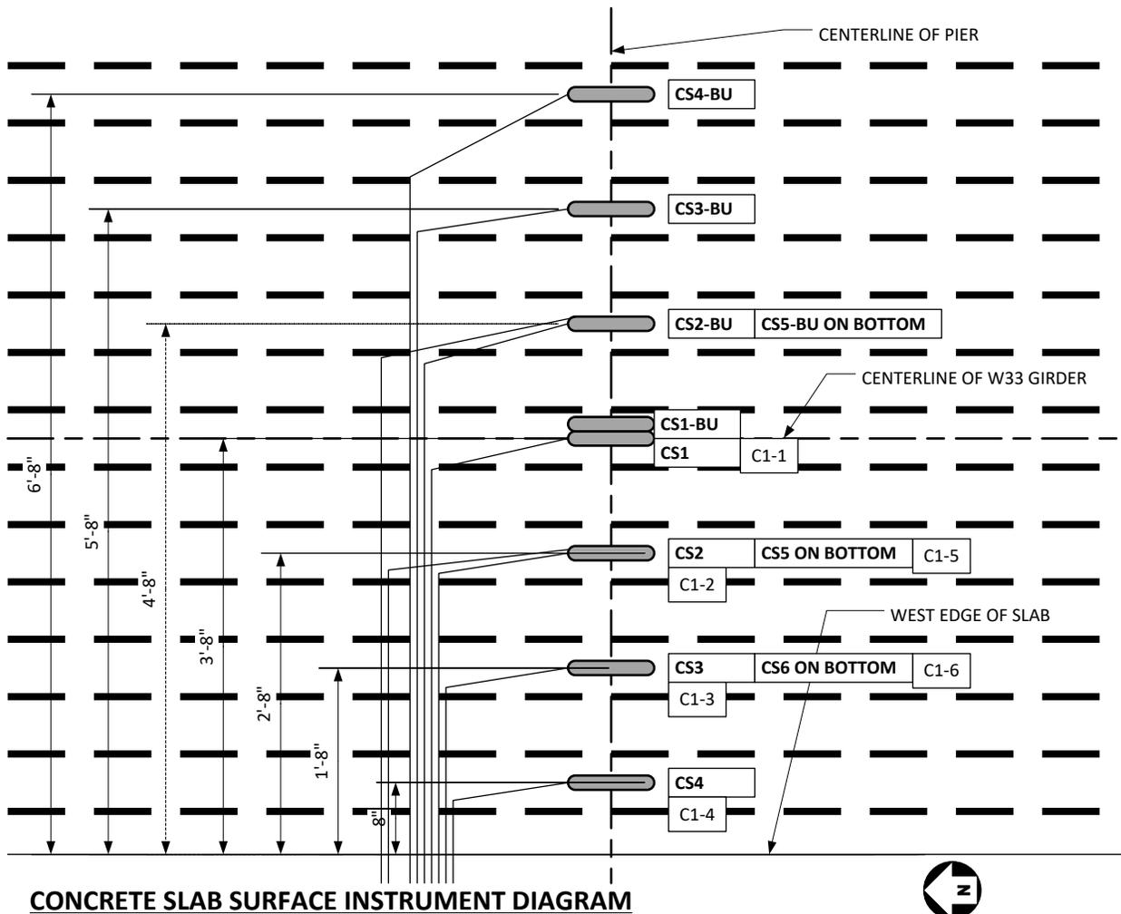
**Figure 64 - Instrumentation Layout on the Top and Bottom of Slab**
