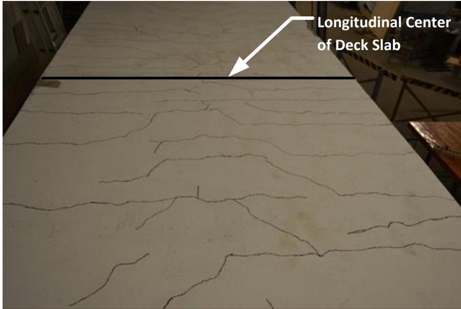
**Figure 93 - Final Crack Pattern in Top of Deck Slab (looking south)**
