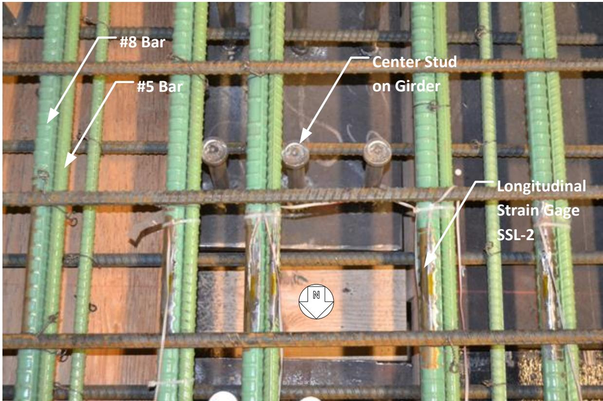
**Figure 66 – Strain Gages Attached to Reinforcing Steel**
