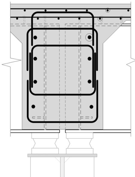
**Figure 7 - Bridge over the Scioto River pier detail**
