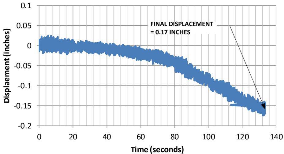
**Figure 78 - Displacement of South Elastomeric Bearing – Day 1**
