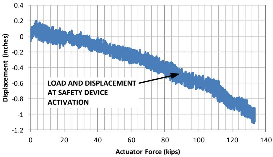
**Figure 76 - Displacement at South Girder vs. Actuator Force – Day 1**
