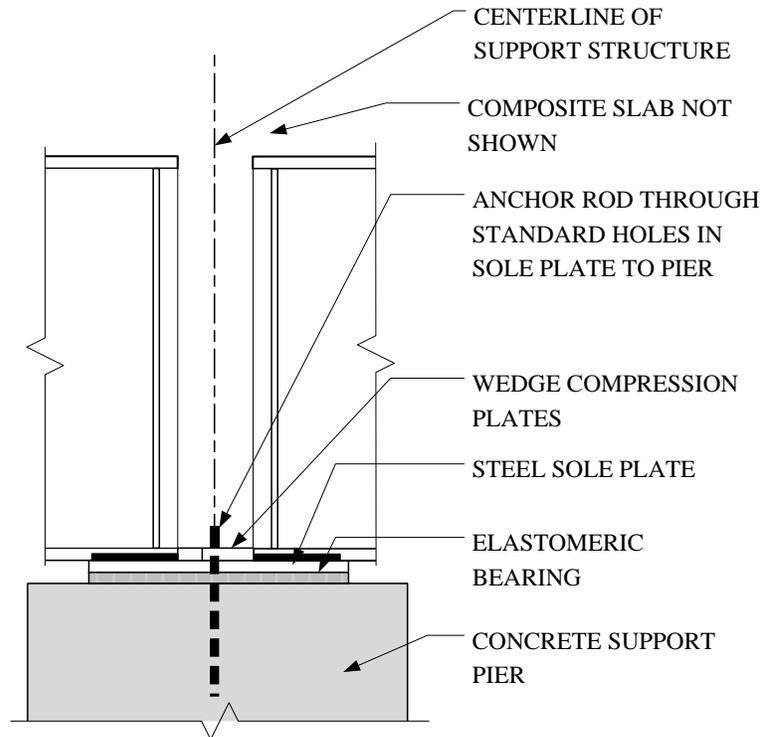
**Figure 105 – SMC Girder Support Detail 2 – Side View**
