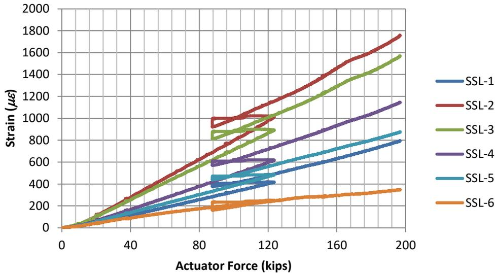
Figure 110 - Day 2 SMC Reinforcing Strains vs. Actuator Force
