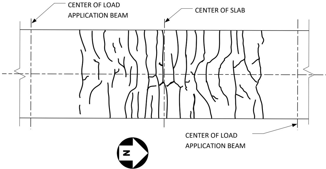
**Figure 94 - Crack Pattern in Top of Deck Slab**
