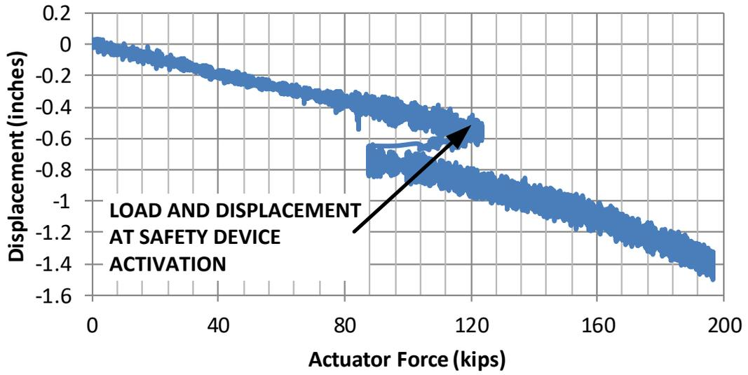
**Figure 91 - Displacement at South Girder vs. Actuator Force - Day 2**
