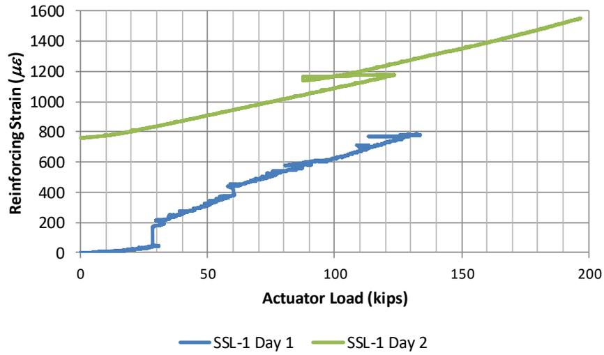
Figure 81 - Comparison of Days 1 and 2 Actuator Load and Reforcing Strain - Scheme 1
