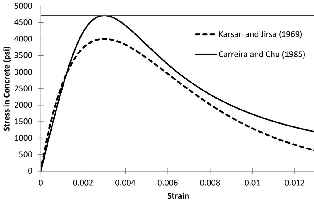
Figure 24 – Damage Model for Concrete in Uniaxial Compression for  $f'_c = 4712$  psi
