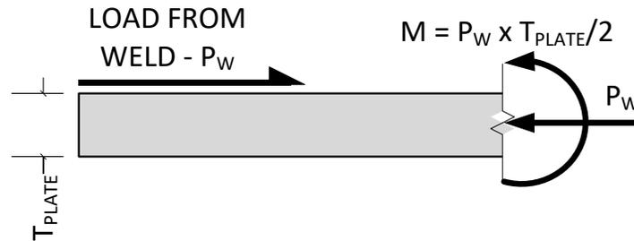
**Figure 67 - Free Body Diagram of Sole Plate**
