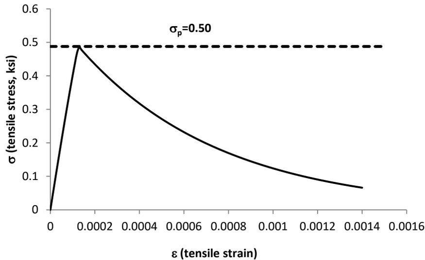
**Figure 23 - Softening Response to Uniaxial Loading Based on Plain Concrete Tensile Damage (Gopalaratnam, 1985)**
