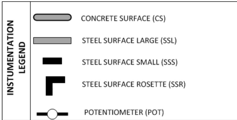
Figure 57 - Legend for Instrumentation Layouts
