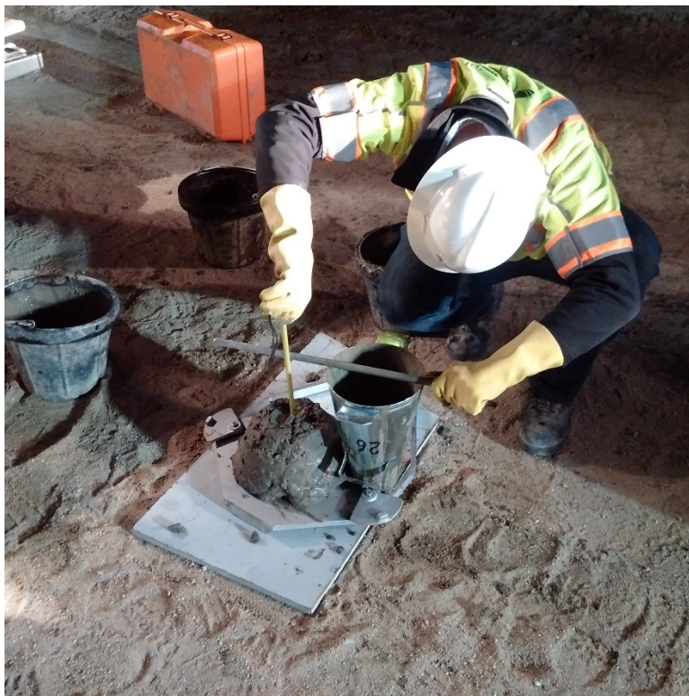
Figure 4-3. Slump test before casting the concrete
