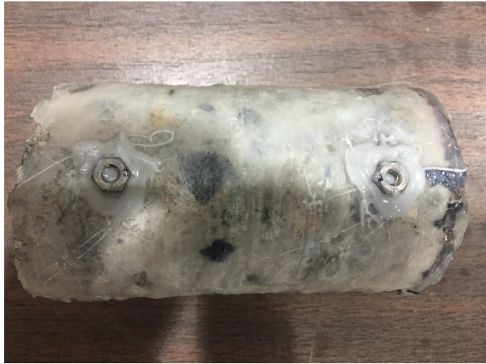
Figure 3-10. Sample prepared for freeze-thaw test
