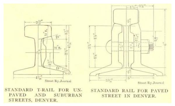
Figure 195. Examples of two variations of T-rails used in Denver.<sup>771</sup>
