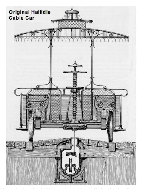
Figure 4. Cross-Section of Hallidie's original cable-car design showing the central cable conduit and grip mechanism beneath the streetcar.<sup>24</sup>
