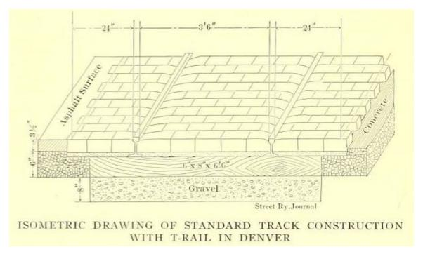
Figure 193. Diagram of a paved section of a Denver streetcar line showing gravel substrate, wooden rail tie stabilized with concrete, and T-rails flanked by brick pavers.<sup>769</sup>
