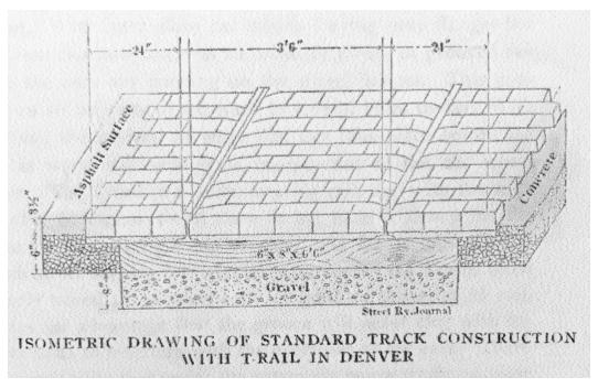
Figure 59. Drawing of Tramway track standards from 1903.<sup>309</sup>
