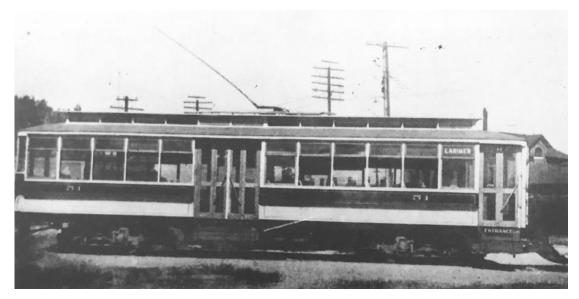
Figure 11. A Safety Car, in which passengers entered from the front and exited from the middle. 147
