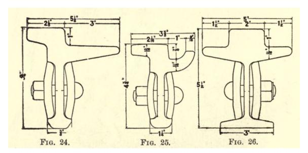
Figure 196. Examples of three configurations of girder rails. From left to right: side bearing, grooved, and center bearing.<sup>772</sup>
