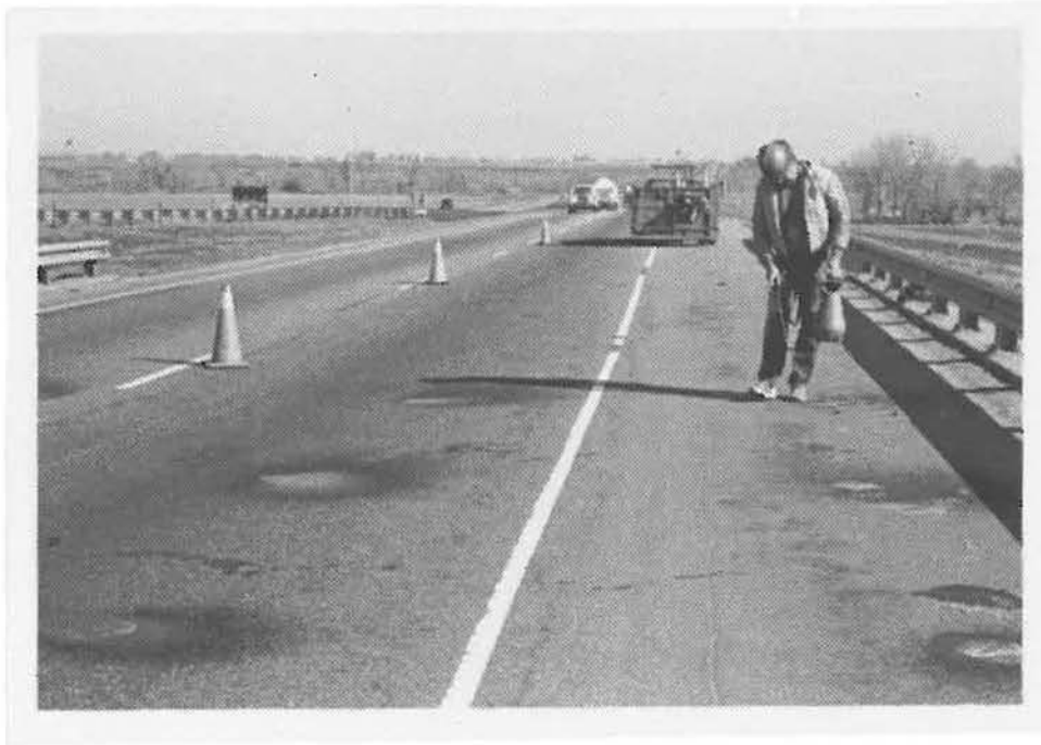
Photograph 1. Prior to testing, the deck is pre- wetted with a mixture of water and soap. The tests are taken on a ten- foot grid.
