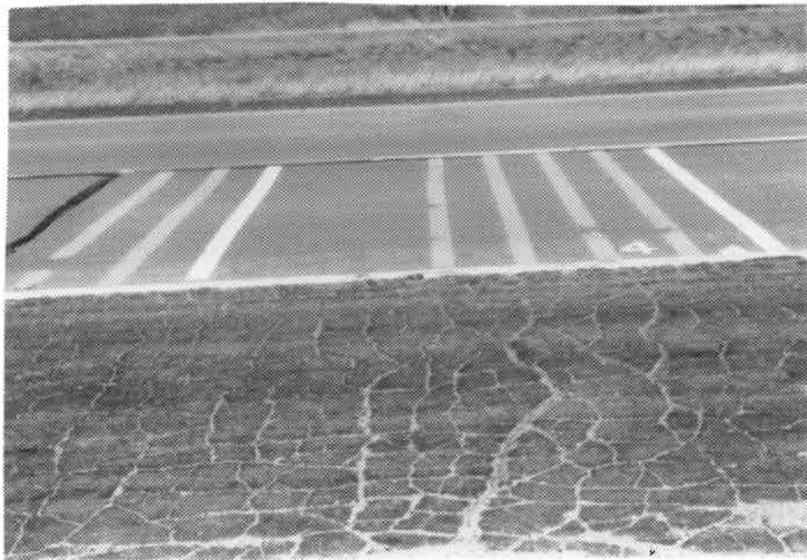
Photo 35. 3/8/89 Cataphote permanent grade preformed plastic on concrete.
