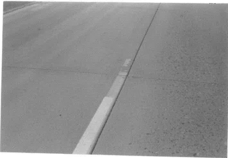
Photo 13. 1/25/88 I76 southbound, just north of Bromley Lane, 1987 fast-dry alkyd paint on bottom, 1986 epoxy paint on top of photo.
