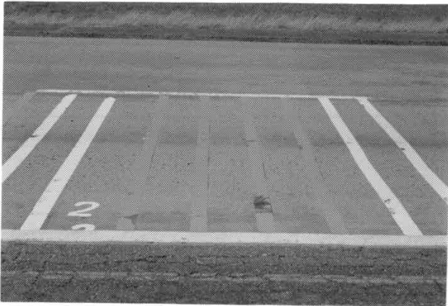
Photo 22. 3/29/88 Swarolite removable grade preformed plastic on concrete.
