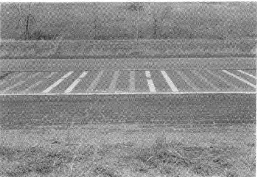
Photo 36. 3/8/89 3M-Std. permanent grade preformed plastic on concrete on left and 3M- 350 permanent grade preformed plastic on concrete.
