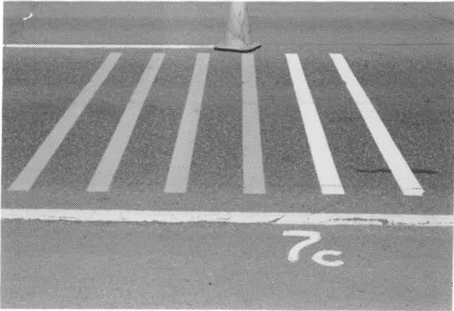
Photo 28. 3/29/88 3M removable grade preformed plastic on asphalt. (Center four stripes)
