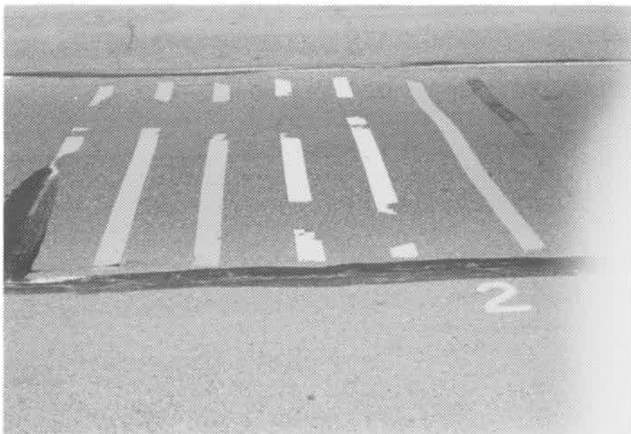
Photo 42. 3/8/89 Swarolite permanent grade preformed plastic on asphalt.
